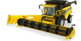
ERT13830 NH CR8090 Comes with 30ft grain head and 12 row corn head, pivoting unloading auger
