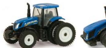
ERT13844 NH T7.235 Oscillating front axle, updated exhaust system and fuel tanks, rear duals
