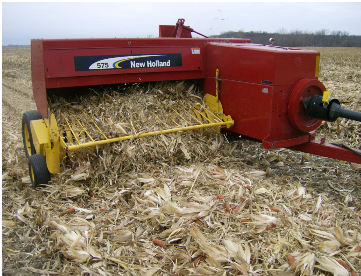
Figure 5 New Holland 575 baler baling stover windrow prepared by the Cornrower at 3.5 mph. Stover moisture is 35% and baling operation followed shelling operation by approximately one hour on a cloudy November day.
