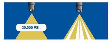
Today's sophisticated diesel engines require cleaner fuel than ever before to operate efficiently, due to injection pressures of more than 30,000 PSI and extremely tight tolerances.
