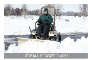
These durable 48- and 60-inch blades are highly efficient at moving snow, and three types of blades are available to meet your needs. Operator's seating position directly above the drive wheels enhances traction in deep, heavy snows.
