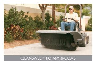
PTO-driven rotary brooms sweep dirt and debris away in record time, making it ideal for sidewalks, parking lots – even walking paths and tracks. Powerful performance also cleans up to 8 inches of snow and reduces time and labor by more than 60%. Learn more at grasshoppermower.com/brooms.
