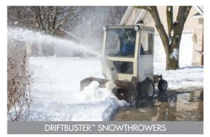
PTO-driven 48- and 60-inch snowthrowers propel snow up to 30 feet and operate in both forward and reverse to maximize efficiency and eliminate three-point turns. The discharge spout rotates a full 180 degrees for on-target placement.
