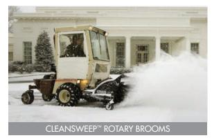
Powerful, PTO-driven 48- and 60-inch rotary brooms clear up to 8 inches of snow, leaving a clean, dry path. Fixed-angle and bidirectional models are available.
