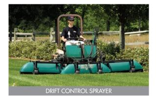
A productive and cost-effective way to apply liquid fertilizers, pesticides and herbicides to turf areas, the ProLawn shielded sprayer applies small droplets that "stick" to vegetation, minimizing chemical use and reducing time and labor more than 60%. *Learn more at grasshoppermower.com/sprayer.*
