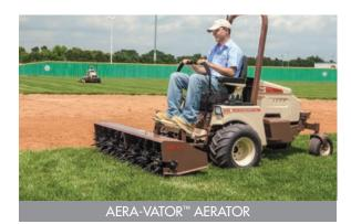
The powerful gyrations of the PTO-driven AERA-vator<sup>™</sup> aerate and loosen compacted soil in 1/4 the time and with 1/4 the labor of walk-behind units, leaving no cores to clean up. Turf is ready for use immediately. *Learn more at grasshoppermower.com/aerate.*
