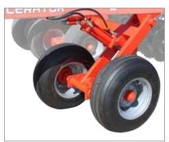
Standard heavy-duty walking beams on the center section feature 8-bolt transport wheel hubs. Wheel spindles are "slip-in" replaceable for easy servicing. Walking beam tandems on each wing frame have 6-bolt hubs with bolt in spindles as standard equipment.
