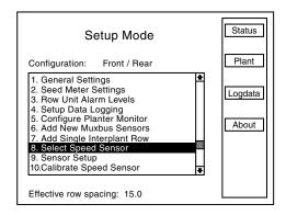
STEP 2 Press knob or Enter key, a drop down menu appears. Highlight "Coil Pick-Up" and press knob or Enter key.
