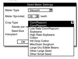
STEP 4 Turn knob or use arrows keys to highlight a crop for planting then press knob or Enter key. Once crop type is entered, "Seeds per rev" is automatically set .
