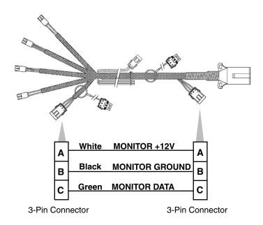
Light package supplied on Model 3000 planter meets ASABE Standards. For correct wiring harness to be wired into lights on your tractor, check with tractor manufacturer.
