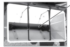
Flighting must move chemicals from center to outside of hopper.
