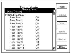
STEP 5 Plug in first pull row unit seed sensor (row 1), working from left to right across planter. Connect interplant unit sensors after all pull row unit sensors have been connected following the same pattern. When a sensor is connected to planter harness wait for monitor to acknowledge sensor with two beeps.
