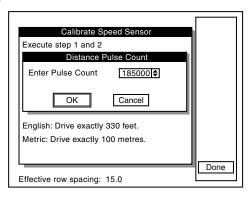
When "Enter Pulse Count" value is highlighted press knob or Enter key and a drop down key pad will appear. Turn knob or use arrow keys to highlight "0", zero, and press knob or Enter key. Turn knob or use arrow keys to highlight "OK" and press knob or Enter key to return to the "Calibrate Speed Sensor" screen.
