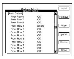
STEP 4 Seed Counting Sensors Too Dirty Warning - When powering on KPM III, seed sensor performs a self check. If a seed tube is too dirty, the message "Clean or Replace Sensor as Necessary" displays and bargraph for that row will flash.. Sensor will not function until problem is corrected.
