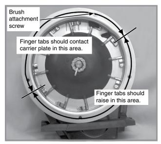
A buildup of debris or chaff may prevent proper finger operation and requires disassembly and cleaning of finger pickup meter.
