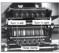
Adjusting squeeze pump end hoses
