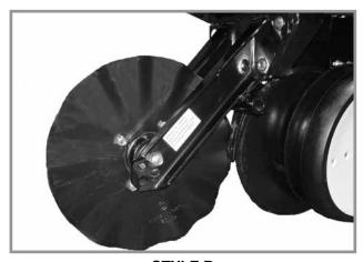
STYLE B (One sleeve for coulter mounted residue wheels)
