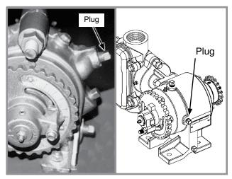
Piston pump oil fill plug location
