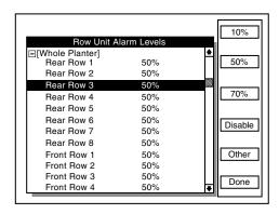
STEP 2 To set alarm thresholds for whole planter, turn knob or use arrow keys to highlight "[Whole Planter]" line. Press key next to desired threshold. When desired threshold is specified for all row units, press F6 key next to "Done".
