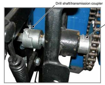
Transmission shaft and drill shaft coupler
