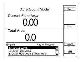
• <u>To Clear Field Area And Total Area</u>, highlight "Clear Field Area & Total Area" and press knob or Enter key. A note will appear to verify decision to reset field area and total area to zero. Highlight "OK" and press knob or Enter key to clear field. Highlight "Cancel" and press knob or Enter key to retain current field values.
