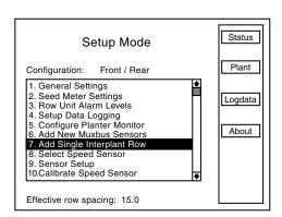
STEP 2 To confirm note below turn knob or use arrow keys to highlight "OK" button, then press knob or Enter key to confirm. If single Interplant row is not to be added select "Cancel" key and press knob or Enter key to cancel or press ESC key.
