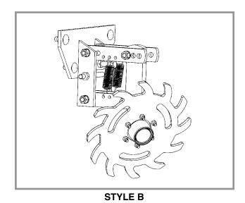
Wheel hub is equipped with sealed bearings. If a bearing sounds or feels rough when wheel is rotated, replace them.
