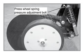
Soil press wheel down pressure adjustment
