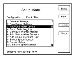
Alarm thresholds can be set for whole planter, any planter section, or individual rows.
