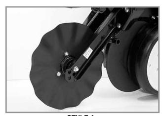
STYLE A (Two sleeves for coulter mounted residue wheels)
