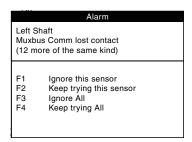
NOTE: When a known sensor or group of sensors are faulty, press F1 or F3. Monitor stops communication with affected sensors and corresponding bargraphs are grayed out on main "Planter Configuration" screen.
