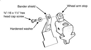
Granular chemical bander shield installation
