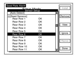
NOTE: Only way to remove an alarm is to find problem and correct it. Alarms are not reported for rows with seed rate alarm thresholds disabled.
