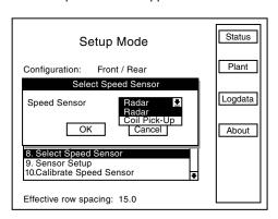
NOTE: To prevent configuration from being changed select Cancel, then press rotary encoder knob, Enter key or ESC key.
