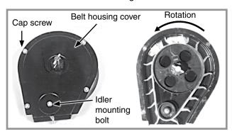
If belt is replaced, make sure paddles are correctly oriented as shown. A diagram molded into the drive sprocket also shows correct orientation.
