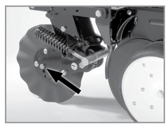
NOTE:Torque %" spindle hardware to 120 ft.lbs.(162.7 N-m)
