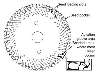
Most seed disc wear is found in the agitation groove area (area between seed loading slots). Wear affects planting accuracy at high RPM. Lay a straight edge across disc surface at agitation groove area and measure gap between disc and straight edge. If agitation groove areas are worn in excess of .030" (7.6 mm) and accuracy starts to drop off at higher meter RPM, replace seed disc.
