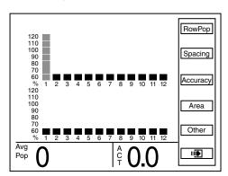
NOTE: Press F2 or F4 if sensors are not faulty. After pressing F2 or F4 a message similar to the one below appears when "Status" button F1 is pressed.
