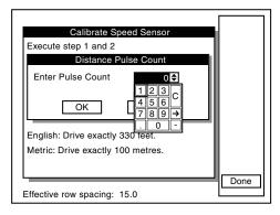
NOTE: If Distance Pulse Count number starts to count pulses with the tractor not moving, check radar distance sensor for vibration or other interference.
