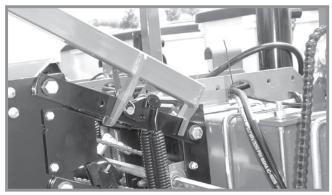
Lift lever positioned on push row unit
