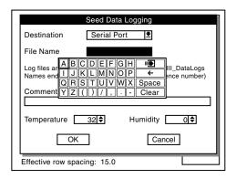
STEP 6 Use knob or arrow keys to scroll to "Comment for file" box. Press knob or Enter key to display drop down keyboard. Use keyboard to enter a Comment for the file then press Enter key.
