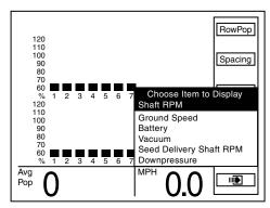
• Press F5 key next to Other for items available to display in bottom R.H. corner. Turn knob or use arrow keys to highlight "Shaft RPM". Value appears in bottom R.H. corner of display as "RPM".
