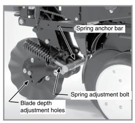
Frame mounted coulter adjustment
