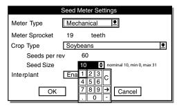
STEP 8 Turn knob or use arrows keys to highlight a crop for planting then press knob or Enter key. Once crop type is entered, the "Seeds per rev" is set automatically.
