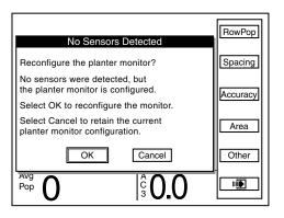
NOTE: Selecting OK reconfigures monitor requiring all sensors to be re-learned. Selecting Cancel keeps current configuration and monitor continues trying to communicate with sensors.
