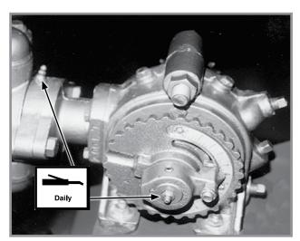
Liquid Fertilizer Piston Pump - 2 (Fill on outboard stuffing box until lubricant seeps out of drain hole in bottom.)
