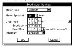
NOTE: When Vacuum "Meter Type" is selected "Meter Sprocket" automatically defaults to 28 teeth. To change "Meter Sprocket" select "Meter Sprocket" by turning knob or using arrow keys. Press knob or enter key, a drop down number pad displays. Turn knob or use arrow keys to highlight first digit of desired number and press knob. When correct number is obtain press knob or enter key.
