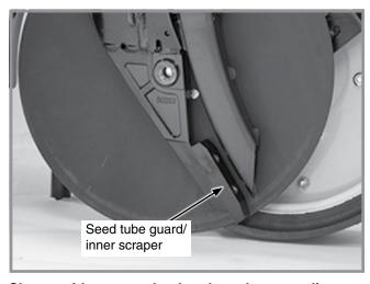
Shown with gauge wheel and seed opener disc blade removed
