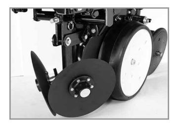
Lubricate bushings in support arm mounting bracket at frequency indicated in Lubrication of this section. Check each bolt for proper torque. If bolt is loose, it should be removed and bushing inspected for cracks and wear. Replace bushings as necessary.
