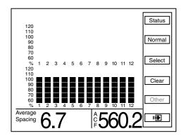
NOTE: Abbreviation for selected area counter appears in bottom R.H. corner of the screen. In above illustration "ACF" stands for Area Counter Field.
