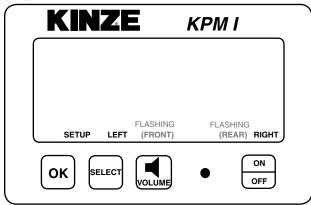
NOTE: Model 3000 planters use rear configuration only. When Interplant® Package rows are in use, select rear/front configurations. When all rows can be viewed on a single display (rear), pressing the select key has no function.
