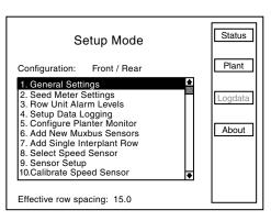
STEP 9 Turn the knob or use the arrow keys to highlight the "Row Spacing" field. Press the knob or Enter key to make the selection. A drop down number pad will appear. Adjust the row spacing to Interplant spacing by turning the knob or use the arrow keys to highlight the correct value then press the knob to select the number, for numbers containing more than one digit select one digit at a time.
