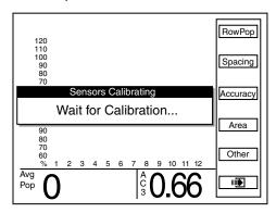
NOTE: Do not attempt planting before "Wait For Calibration" message disappears. If planter is moving while sensors are calibrating alarms will be generated.
