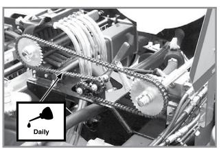
Liquid Fertilizer Drive Chain (Squeeze Pump Shown)
