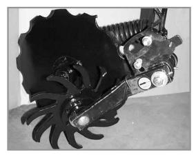
Notched single disc opener residue wheel attachment
