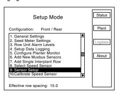
STEP 4 Turn knob or use arrow keys to highlight faulty sensor and press F2 key next to Remove.
