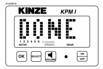
STEP 8 Follow STEPS 5 through 7 to install the second section. If no seed tubes are installed on the second section, press and hold the OK key until "DONE" shows on the screen followed by a long beep and the SAVE? icon turns off.
