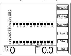
NOTE: Planter Configuration screen displays planter rows as programmed into KPM III software. The above screen shows 12 front (Interplant) rows and 12 rear rows. If the KPM III were programmed for 8 front (Interplant) rows and 8 rear rows the screen would display 8 front and 8 rear rows.
