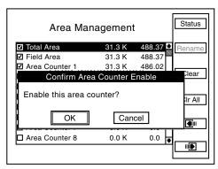
• Use knob or arrow keys to highlight "OK" button and press knob or Enter key. Enabled "Area Counter" starts accumulating area.
