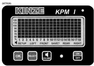
The KPM I electronic seed monitor system consists of a tractor mounted console, seed tubes with computerized sensors installed in each planter row unit, a primary harness\* connecting the console to the planter harness, and a planter harness (junction Y-harness and/or harness extension where applicable), connected to individual seed tube sensors.
