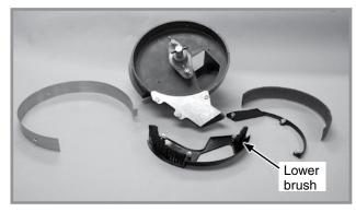
Lower brush moves seed down seed loading slots to seed pockets, isolates seed in reservoir from entering seed tube, and cleans seed loading slots.
