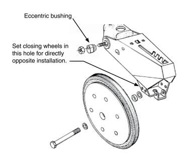
"V" closing wheels should have enough down pressure to close the seed trench and ensure good soil to seed contact. Move 5-position quick adjustable down force lever on the top of closing wheel arm to the rear to increase closing wheel spring pressure. Move lever forward to decrease pressure. Adjust all row units to a similar setting. Light soil usually requires less down force at average depth (approximately 2" (5 cm)) while heavy soil requires increased down force.
