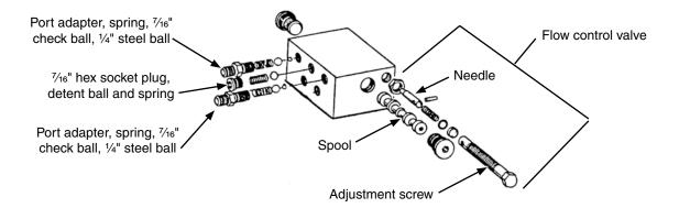
The valve block assembly consists of the row marker sequencing and flow control valves in one assembly. Sequencing valve portion consists of a chambered body containing a spool and series of check valves to direct hydraulic oil flow.
