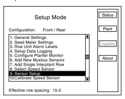
STEP 3 Turn knob or use arrow keys to highlight "8. Select Speed Sensor" and press knob or Enter key.
