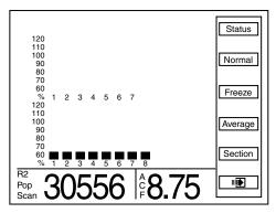
Press F3 key next to Freeze to stop scanning. Left display item will be frozen on a particular row. "Frzn" appears in lower L.H. corner to indicate display is frozen. To resume scan press F3 key next to Scan.
