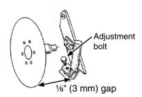
Adjust liquid drop tube/scraper so there is slight contact between blade and scraper lower leading edge, and  $\frac{1}{4}$ " (6.35 mm) clearance between liquid drop tube trailing edge and blade. Blade should turn with minimum amount of drag.
