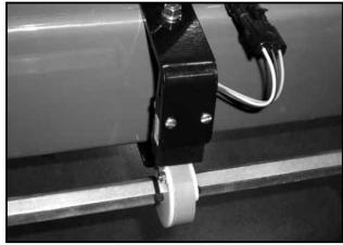
"LSHAFT" or "SHAFT 1" will display on the lower LCD when the first shaft rotation sensor is installed. "RSHAFT" or "SHAFT 2" will display when the second shaft rotation sensor is installed.
