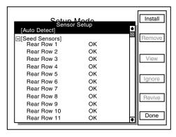
STEP 6 When "OK" appears behind ALL sensors, press F6 key next to Done. 'Setup Mode" menu displays.
