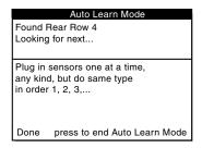
NOTE: After each sensor has been installed "OK" appears after sensor name on LCD screen.
