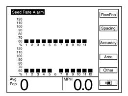
If sensor detects no seed flow it displays which row is not functioning. Alarm may be caused by a mechanical problem reducing seed flow or an electrical problem causing an incorrect seed count.
