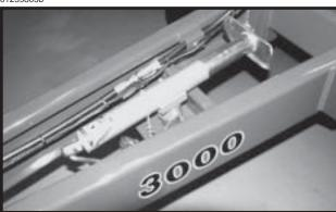
Lower planter to the planting position and check to be sure planter is level fore and aft. If hitch height is too high or low, disconnect planter and adjust hitch clevis up or down as necessary.
