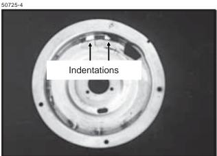
**Photo Shows Worn Carrier Plate**
