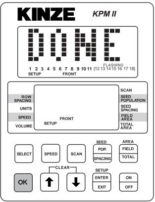
STEP 10 With the lower display showing "GNDSPD", connect the distance sensor. The monitor will display "PICKUP" if a magnetic distance sensor is connected or "RADAR" if a radar distance sensor is installed. Only one distance sensor can be connected at a time.
