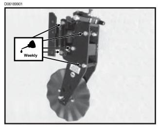
Frame Mounted Coulter Parallel Linkage - STYLE A (10 Per Row)
