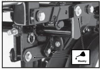
Row Unit Mounted Disc Furrower Parallel Linkage (6 Per Row)
