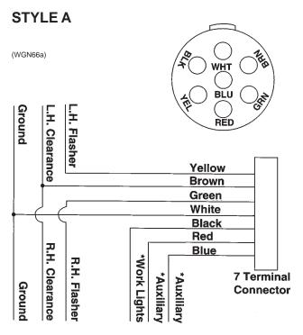
\* Optional customer-supplied auxiliary lights and wires may be wired into existing plug terminals.
