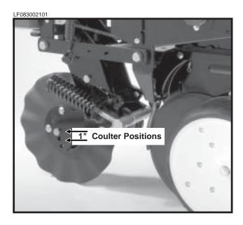
Frame mounted coulters with 1" bubbled, 1" fluted (8 flutes) or <sup>3</sup>/<sub>4</sub>" fluted (13 flutes) blades may be used on pull row units only. (Not compatible with push row units.)
