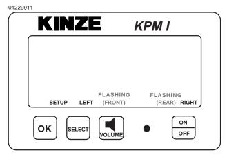
NOTE: Model 3000 planters will use the rear configuration only. When Interplant® Package rows are in use, select the rear/front configurations. When all rows can be viewed on a single display (rear), pressing the select key has no function.
