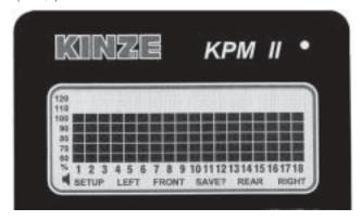
The monitor collects data on the planting rates from all active rows and calculates an average. This average will determine the 100% mark. Seed rate for each row is then compared to the average value and the result is displayed on the bar graph.
