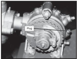
Check crankcase oil daily and maintain at plug level. Fill as needed with EP 90 weight gear oil. Total oil capacity is approximately <sup>3</sup>/<sub>4</sub> pint.
