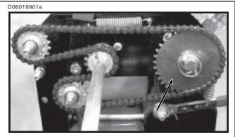
Half Rate (2 To 1) 34 Tooth Drive Sprocket
