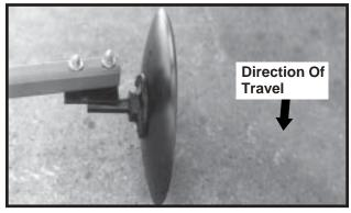
The marker blade is installed so the concave side of the blade is outward to throw dirt away from the grease seals. The spindle assembly is slotted so the hub and blade can be angled to throw more or less dirt. To adjust the hub and spindle, loosen the hardware and move the assembly as required. Tighten bolts to the specified torque.
