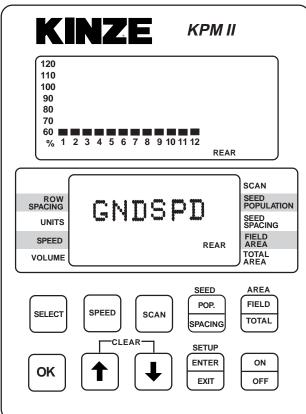
NOTE: To reprogram the system to monitor more or less rows (up to the maximum of 18 per section, 72 total in four section configuration), all sensors must be unplugged, followed by the complete setup procedure.
