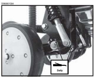
HD Single Disc Fertilizer Opener - 2 Zerks (Located On Wheel Arm And Opener Mount)
