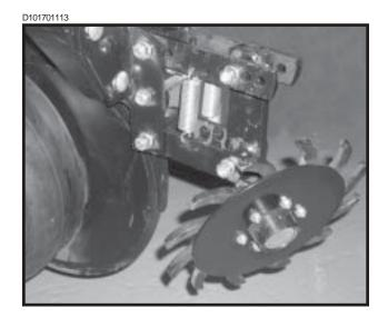
The wheel hub is equipped with sealed bearings. If a bearing sounds or feels rough when the wheel is rotated, replace the bearing.
