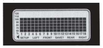
The monitor collects data on the planting rates from all active rows and calculates an average. This average will determine the 100% mark. Seed rate for each row is then compared to the average value and the result is displayed on the bar graph.
