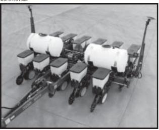
On machines equipped with the squeeze pump option, the rate of liquid fertilizer application is determined by the combination of sprockets on the squeeze pump drive and driven shafts. When changing sprocket combinations, make sure sprockets are in alignment, sprocket retaining collars are tight and chain tension is sufficiently restored.
