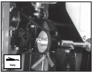
Fertilizer Transmission - 1 Zerk Per Transmission
