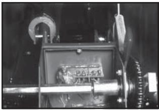
NOTE: The nut on the mounting bolt (on applicable idler assemblies) must be kept tight or chain tension will not be maintained and adjustment wrench will not function properly.
