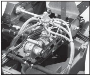
If the machine is equipped with the piston pump option, the rate of liquid fertilizer application is determined by the piston pump settings. The delivery rate chart found at the end of this section provides an approximate application rate only. Actual delivery will vary with temperature and the particular fertilizer being used.
