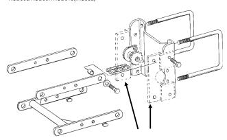
Row unit extension brackets are required on all rear row units if the Model 3000 planter is equipped with coulter mounted residue wheels and HD single disc fertilizer openers. The brackets extend the row units rearward 4" to provide required clearance.
