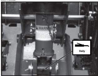
Planter Lift Cylinders (Master, Slave And Assist)-1 Zerk Per Cylinder.
