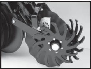
Coulter mounted residue wheels are designed for use on pull row units and push row units. Row unit extension brackets are required on all the pull row units if the planter is equipped with coulter mounted residue wheels and HD single disc fertilizer openers.
