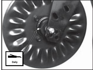
(If Applicable) Frame Mounted Coulter Hubs - STYLE A - 1 Zerk Per Hub
