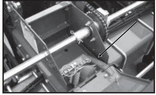
Additional shear pins can be found in the storage area located on the wheel module.
