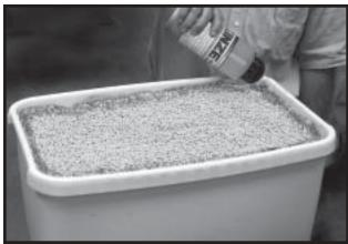
NOTE: Do NOT apply graphite only in the center of the hopper. It will filter too quickly through the seed and not distribute as evenly as desired.
