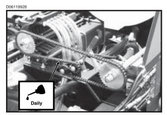
Liquid Fertilizer Drive Chain (Squeeze Pump Shown)
