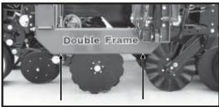
With the planter lowered to proper operating height, check to be sure the frame is level for and aft. Recheck once planter is in the field.
