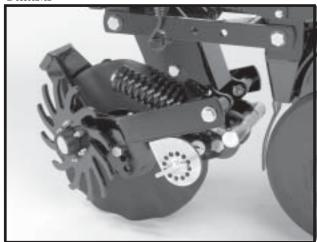
The wheel hub is equipped with sealed bearings. If a bearing sounds or feels rough when the blade is rotated, replace the bearing.
