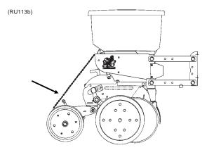
Plant a short distance and check to see if seed is visible in the seed trench. Adjust planting depth to a shallower setting if seed is not visible and recheck.
