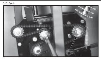
Standard Rate (1 To 1) 17 Tooth Drive Sprocket
