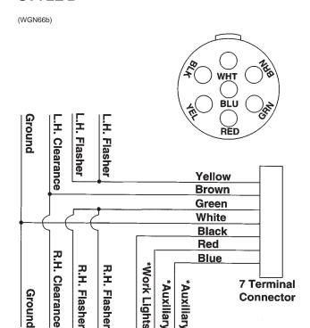
\* Optional customer-supplied auxiliary lights and wires may be wired into existing plug terminals.
