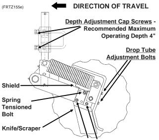
Knife/Scraper Leading Edge Adjustment Bolts (If not equipped with a shield and spring tensioned bolt, the third knife/scraper attachment bolt is also an adjustment bolt.)
