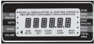
Press the UP or DOWN arrow keys to move the flashing arrow on the lower LCD to change what is displayed on the lower LCD.
