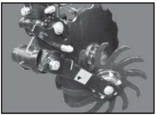
The residue wheel attachment for the notched single disc fertilizer opener is designed for applications where row unit mounted residue wheel attachments cannot be installed. The residue wheel is attached to the notched single disc fertilizer opener using 5/8" x 3 1/2" and 1/2" x 1 3/4" hardware.
