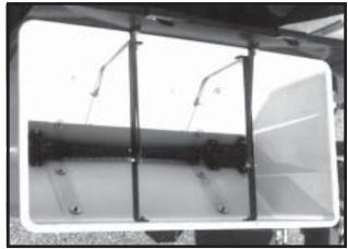
Check auger installation by rotating the shaft in the direction shown below to see that the spirals on the auger move toward the ends of the hopper. If not, remove auger assembly, turn 180° and reinstall.
