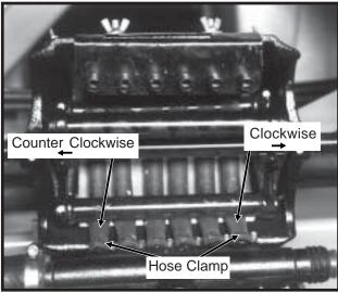
For the right hand hose (facing the pump from front of planter as shown above) twist the hose 1/4 turn in the clockwise direction.
