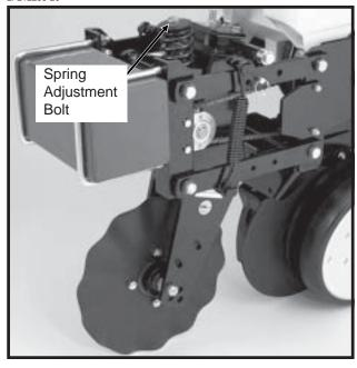
Frame mounted coulters with 1" bubbled, 1" fluted (8 flutes) or <sup>3</sup>/<sub>4</sub>" fluted (13 flutes) blades may be used on pull row units only. (Not compatible with push row units.)
