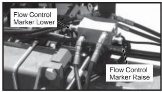
IMPORTANT: The flow controls should be properly adjusted before the marker assemblies are first put into use. Excessive marker travel speed can damage the marker assembly.
