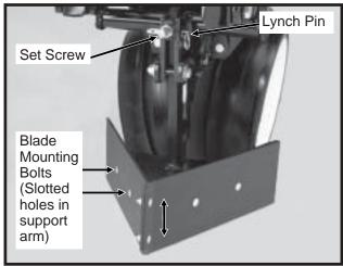
Row unit mounted bed levelers may be used on pull row units only. They are not compatible with push row units.
