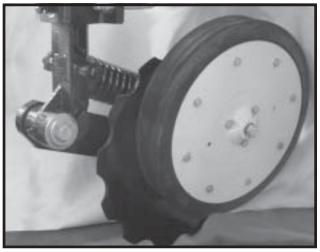
The depth/gauge wheel attachment for the notched single disc fertilizer opener is designed for use in situations where additional gauging is required to maintain desired fertilizer opener depth. The depth/gauge wheel is attached to the notched single disc fertilizer opener using a mounting block fastened to the pivot arm using  $^5/_8$ " hardware through the disc blade bearing.
