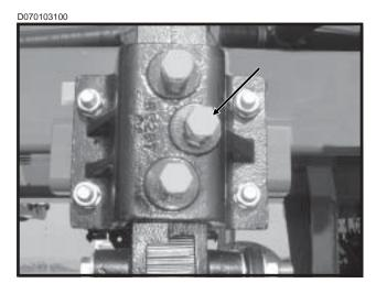
NOTE: Middle cap screw must be tightened prior to tightening depth adjustment cap screws.
