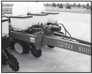
The Interplant® Self-Leveling Hitch Extension is designed to allow the planter to raise level, front to rear, when Interplant® push row units are used.
