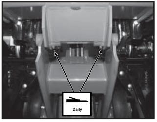
4. Wheel Module Assembly - 2 Zerks Per Module
