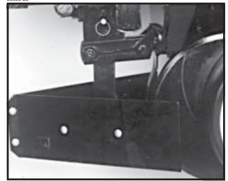
Lubricate the bushings in the mounting bracket and links at the frequency indicated in the Lubrication Section of this manual. Using a torque wrench, check each bolt for proper torque. If the bolt is loose, it should be removed and the bushing inspected for cracks and wear. Replace bushing if necessary. Only hardened flat washers should be used. Replace damaged flat washers with proper part. Torque bolts to 130 ft. lbs.
