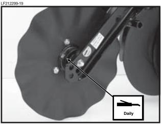
(If Applicable) Row Unit Mounted No Till Coulter Hubs - 1 Zerk Per Hub
