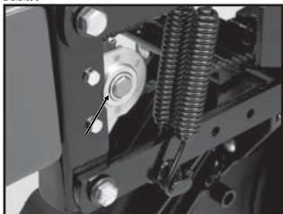
A number of sealed bearings are used on your KINZE® planter to provide trouble free operation. These are located in such areas as the drive shaft, row units and transmission bearings. Sealed bearings are lubricated for life. Due to the seals, relubrication is not practical.
