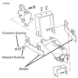
Eccentric bushings allow for lateral adjustment of the drag closing attachment. Using a 3/4" wrench, loosen the hardware which attaches the assembly to the wheel arm stop. Using another 3/4" wrench, turn the eccentric bushings until the drag closing attachment is aligned with the seed trench.
