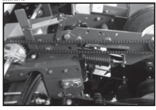
Interplant® push row unit drive chain adjustment is made by loosening the idler sprockets mounting hardware and sliding the sprockets in the slotted mounting holes.
