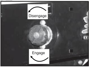
To disengage the drive, turn the knob 1/4 turn counterclockwise. To engage the drive, turn the knob 1/4 turn clockwise.
