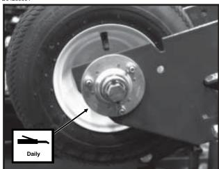
(If Applicable) Contact Wheel Arm Bearing - 2 Zerks Per Arm Assembly (Rotate tire while filling with grease.)
