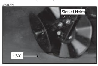
Initial setting for each disc furrower blade is 1 <sup>3</sup>/<sub>4</sub>" shallower than the coulter blade. Further adjustment may be desired for various applications.
