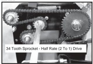
Half rate (2 to 1) drive is recommended only when desired population falls below that on planting rate charts. Replacing the 17 tooth drive sprocket located on the inner side of the top transmission shaft, with the 34 tooth half rate (2 to 1) drive reduction sprocket will reduce the planter transmission speed and reduce planting and application rates by approximately 50%.
