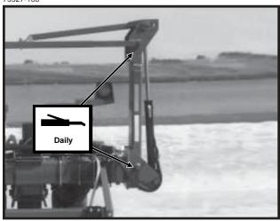
2. Low Profile Marker Assembly - 2 Zerks Per Assembly
