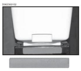
Part No. G7100-258 Red Reflective Decal (Qty. 1 Per Row Unit - Located On The Granular Chemical Hopper Panel Extension On The Outside Row On Both Sides Of The Planter) (If Applicable)
