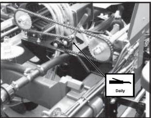
Squeeze Pump/Piston Pump Drive Chain Idler - 1 Zerk Per Idler (Squeeze Pump Shown)
