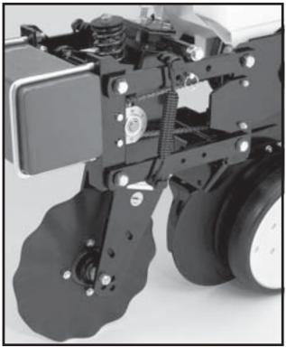
If properly maintained and lubricated (If Applicable) the bearings in the frame mounted coulter hub may never need to be replaced. Lubricate (If Applicable) at frequency indicated in the Lubrication Section of this manual. Check periodically to be sure nuts and hardware are tightened to proper torque specification. Be sure the coulter is positioned square with the planter frame and aligned in front of row unit disc opener.
