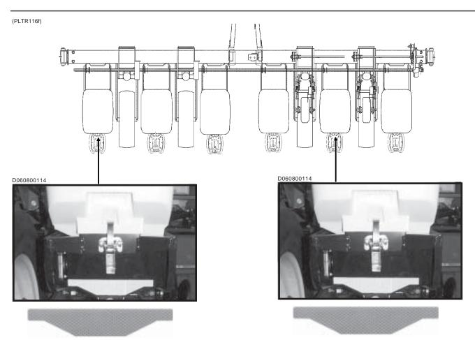
Part No. G7100-261 Red Reflective Decal (Qty. 1 Per Row Unit - Located On The Hopper Support On The Outside Row On Both Sides Of The Planter) (If Applicable)
