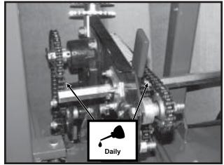
**Transmission Assembly And Reverser Plate Chains**
