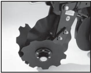
The blade hubs are equipped with sealed bearings. If a bearing sounds or feels rough when the blade is rotated, replace the bearing.
