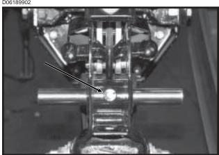
3. Install the replacement spindle and position as shown below. Exact centering is critical.
