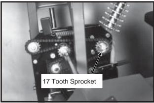
Seed planting rate charts are based on the standard rate drive unless specified otherwise. The standard rate drive uses a 17 tooth sprocket as shown above. Using the 34 tooth half rate (2 to 1) drive reduction sprocket in place of the 17 tooth sprocket will reduce the planting and application rates by approximately 50%. See "Half Rate (2 To 1) Drive".
