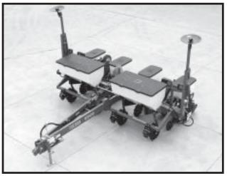
The rate of fertilizer application is determined by the drive/driven sprocket combination on the fertilizer drive and by the auger position in the hopper.
