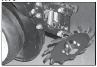
Two adjustable springs on the parallel links on each residue wheel allow for down force adjustment. Position 1 as shown below provides minimum down pressure and position 3 maximum down pressure.
