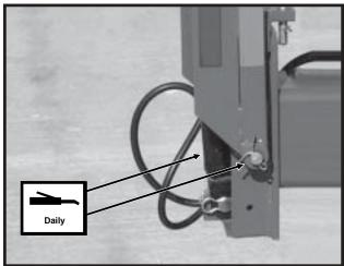
Conventional Marker Assembly - 4 Zerks Per Assembly
