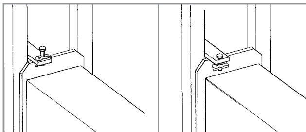
Pin Stored In Raised Position For Marker Operation
