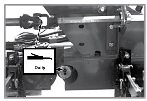
6. Cam Follower - 1 Zerk Per Cam 7. U-Joint Assembly - 1 Zerk Per Assembly
