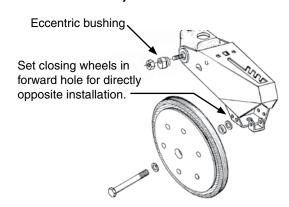
"V" closing wheels should have enough down pressure to close the seed trench and ensure good soil to seed contact. Move 5-position quick adjustable down force lever on the top of closing wheel arm to the rear to increase closing wheel spring pressure. Move lever forward to decrease pressure. Adjust all row units to a similar setting. Light soil usually requires less down force at average depth (approximately 2" (5 cm)) while heavy soil requires increased down force.
