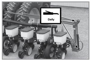
1. Row Markers - 4 Zerks Per Assembly On 8 Row 38"/40" And 12 Row 30" Sizes. 2 Zerks Per Assembly On 12 Row 36"/38", 12 Row 38"/40" And 16 Row 30" Sizes.
