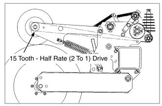
Half rate (2 to 1) drive is recommended only when the desired population falls below that shown on the planting rate charts. Replace the 30 tooth drive sprocket and shorter No. 40 110 pitch chain on each contact wheel with a 15 tooth sprocket. This will reduce the planter transmission speed and reduce planting and application rates by approximately 50%.
