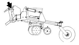
On planters equipped with the optional Dual Lift Assist Wheel Package, adjustment holes on the lift assist cylinder mounts allow for adjustment of lift height.
