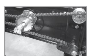
**Mechanical Pull Row Unit Meter Drive**
