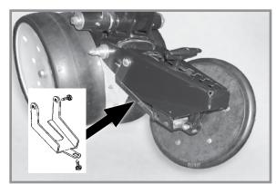
Closing wheel shield (Closing wheel removed)
