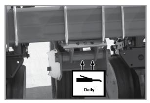
5. Drive Wheel Arm Pivot - 2 Zerks Per Pivot
