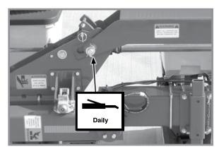
2. Wing Hinge - 2 Zerks Per Hinge Area
