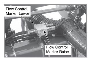
NOTE: Backing flow control valve out too far can cause the o-ring seal on valve to fail when hydraulics are operated.
