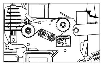
Planting population rate changes are made at the seed rate transmissions. The seed rate transmissions are designed to allow simple, rapid changes of sprockets to obtain the desired planting population. By removing the lynch pins on the hexagon shafts, sprockets can be interchanged with those from the sprocket storage rod bolted near each transmission.
