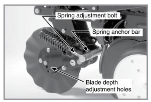
Frame mounted coulter adjustment
