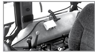
If the circuit breaker on the control box is not tripped, determine if the problem is electrical or mechanical. Place the operational switch in the RIGHT or LEFT position. Check the clutch and wiring harness for power with a test light or volt meter. If the solenoid is operating properly, the plunger on the solenoid will retract causing a clicking sound. The plunger will also be magnetized which can be checked by touching the plunger with a metal object.
