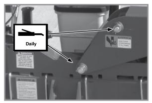
3. Center Hinge - 4 Zerks Per Hinge Area
