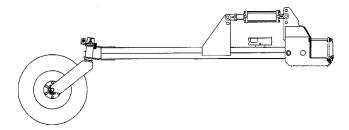
Dual lift assist wheel equipped machines require use of a quick hitch (customer-supplied) and the top link pin is not used.
