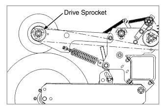
NOTE: 15 tooth, 19 tooth or 30 tooth drive sprockets at each contact drive wheel can be interchanged from the sprocket storage rod bolted near each transmission. The 15 and 19 tooth sprockets require use of a 218 pitch No. 40 chain. The 30 tooth sprocket requires use of a 224 pitch No. 40 chain.
