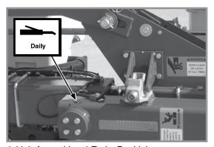
4. Link Assembly - 4 Zerks Per Link
