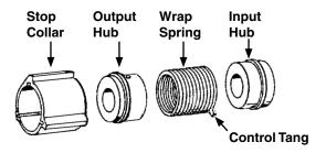
The point row clutch consists of a wrap spring riding on an input hub and an output hub. During operation the wrap spring is wrapped tightly over the hubs connecting them in a positive engagement. The greater the force of rotation the tighter the grip of the spring on the hubs. Rotation in the opposite direction or stopping the spring from rotating prevents the transmission of torque from the input hub to the output hub stopping the planter drive.
