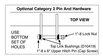
When using a quick hitch (customer-supplied), match pin location to pin spacing in the quick hitch. Adjust the tractor upper link until the quick hitch is vertical when in the planting position.
