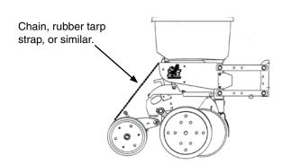
2. Plant a short distance and check to see if seed is visible in the seed trench. Adjust planting depth to a shallower setting if seed is not visible and recheck.
