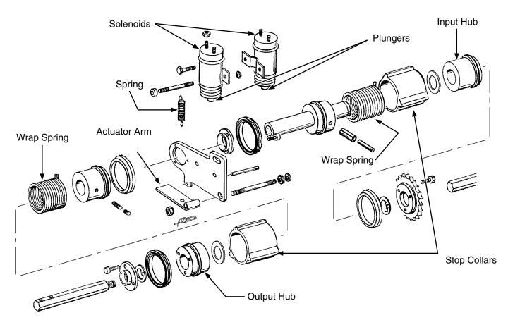
Two-speed point row clutch main parts
