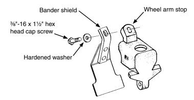
Optional granular chemical bander shield is installed on underside of wheel arm stop to shield crop residue from lodging in granular chemical bander.
