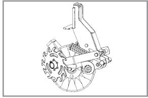
Frame mounted coulter residue wheels
