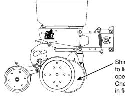
Shim gauge wheel to lightly contact opener disc blade. Check adjustment in field position.
