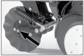
Frame mounted coulter spindle
