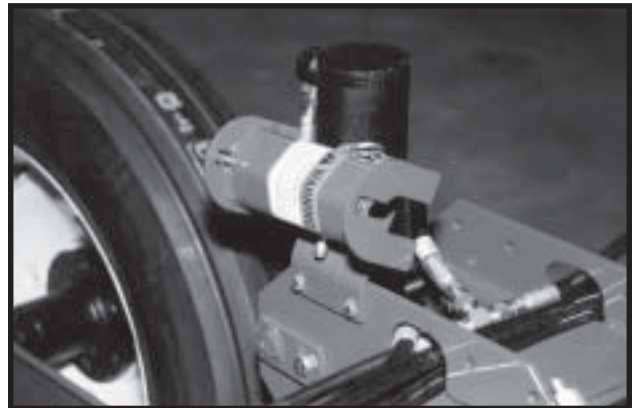
Lift Cylinder Lockup In Storage Position
