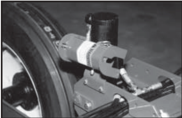
Lift Cylinder Lockup In Storage Position
