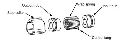
Clutch consists of a wrap spring riding on an input and output hub. Wrap spring is wrapped tightly over hubs during operation locking them together. Higher speeds create a tighter grip of spring on hubs.
