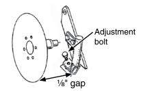
Adjust liquid drop tube/scraper so there is slight contact between blade and scraper lower leading edge, and <sup>1</sup>/<sub>4</sub>" (0.6 cm) (clearance between liquid drop tube trailing edge and blade. Blade should turn with minimum amount of drag.
