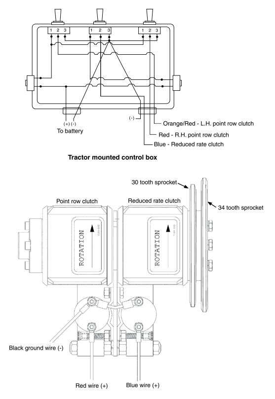
Two-speed point row clutch (Clutch for L.H. side of planter shown)
