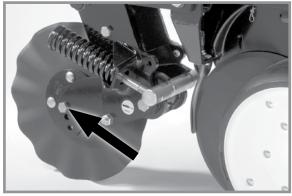
Frame mounted coulter spindle
