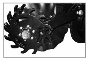
Wheel hubs are equipped with sealed bearings. If bearings sound or feel rough when wheel is rotated, replace them.
