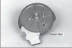
Brush-type seed meter seed disc installed
