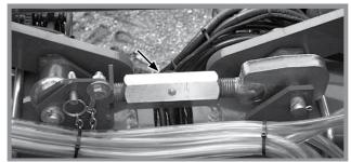
Center turnbuckle installation
