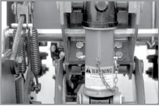
Lift cylinder lockup in transport position
