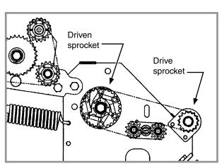
Ratio of population reduction is determined by sprocket ratio between wheel module drive and driven sprockets.
