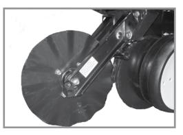
Row unit mounted no till coulters with 1" bubbled, 1" fluted (8 flutes) or <sup>3</sup>/<sub>4</sub>" fluted (13 flutes) blades may be used on pull row units and push row units (<sup>3</sup>/<sub>4</sub>" fluted shown). Four quick adjustable down force springs are required per row when using row unit mounted no till coulters. See "Quick Adjustable Down Force Springs Option".
