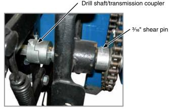
Transmission shaft and drill shaft coupler
