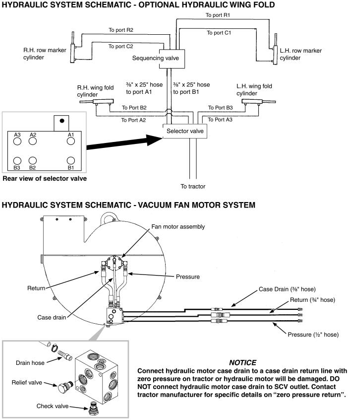
Vacuum fan motor valve block assembly (See machine operation section)
