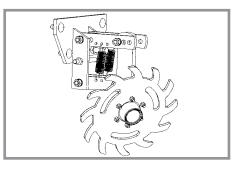
Two adjustable springs on each residue wheel parallel links provide down force adjustment. Position 1 provides minimum down pressure and position 3 maximum down pressure.
