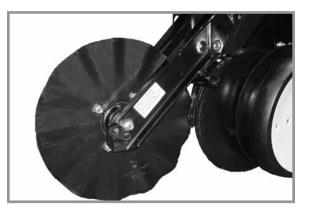
Check nuts and hardware periodically for proper torque.
