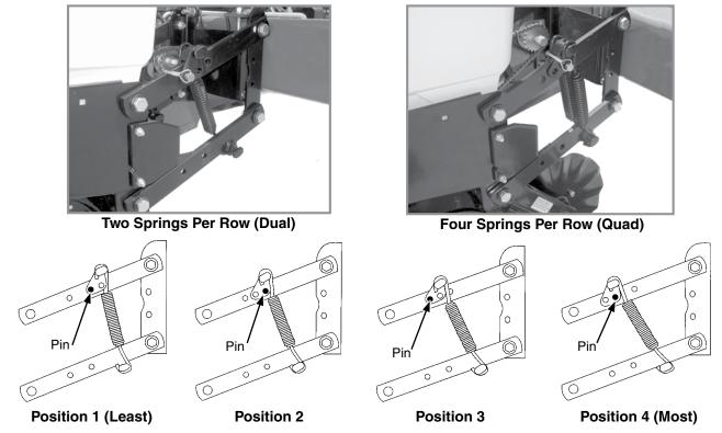
There are four positions to set down pressure spring tension.
