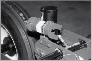
Lift cylinder lockup in storage position
