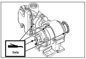
**Liquid fertilizer piston pump - 4** (Fill fitting on outboard stuffing box until lubricant seeps out of drain hole in bottom.)
