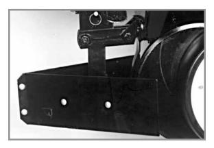
Lubricate bushings in mounting bracket and links at frequency indicated in Lubrication of this section. Check each bolt for proper torque. If bolt is loose, it should be removed and bushing inspected for cracks and wear. Replace bushing if necessary.
