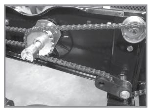
Mechanical pull row unit meter drive
