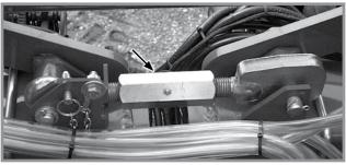
Center turnbuckle installation
