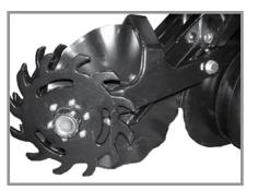
Residue wheels attach to row unit mounted coulter with two cap screws and sleeves allowing unit to free-float. A 2-position spindle bolt mounting positions wheels interlocked or staggered. Depth adjustment is made with a spring-loaded cam and pin with 11 positions in 1/4" (6 mm) increments. A high point on the cam allows wheels to be locked up.
