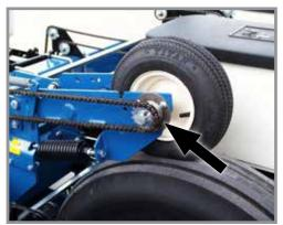
Contact wheel drive sprocket
