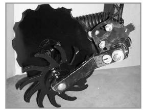
Notched single disc opener residue wheel attachment
