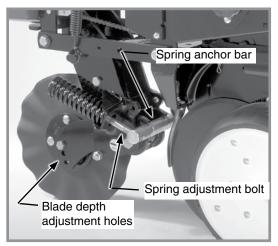
Frame mounted coulter adjustment
