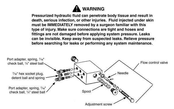
The valve block assembly consists of the row marker sequencing and flow control valves in one assembly. Sequencing valve portion consists of a chambered body containing a spool and series of check valves to direct hydraulic oil flow.
