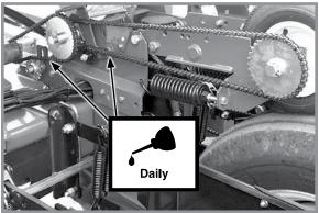
Liquid Fertilizer Piston Pump Drive Chains
