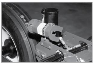
Lift cylinder lockup in storage position
