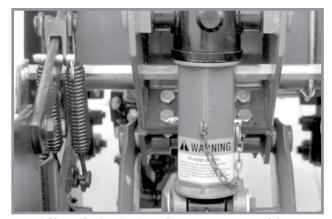
Lift cylinder lockup in transport position
