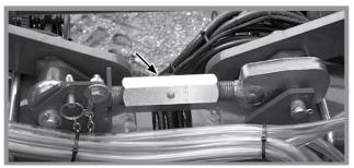
Center turnbuckle installation
