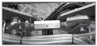
Center turnbuckle installation
