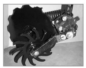
Notched single disc opener residue wheel attachment
