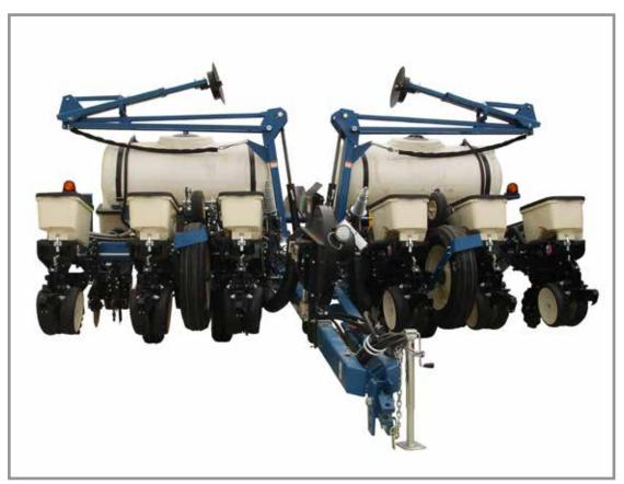
3200 Wing Fold EdgeVac 12 row 30" with liquid fertilizer option (shown folded)
