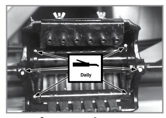
Squeeze pump - 8 per pump NOTE: Grease fittings are on each end of roller assemblies. Rotate pump for access.
