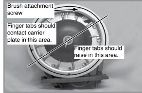
Removing meter and baffle
