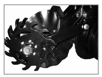
Wheel hubs are equipped with sealed bearings. If bearings sound or feel rough when wheel is rotated, replace them.
