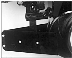
Lubricate bushings in mounting bracket and links at frequency indicated in Lubrication of this section. Check each bolt for proper torque. If bolt is loose, it should be removed and bushing inspected for cracks and wear. Replace bushing if necessary.
