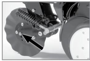
Frame mounted coulter spindle
