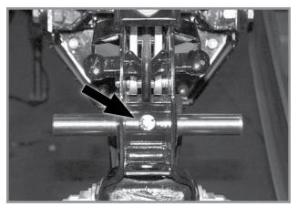
3. Install replacement spindle and position as shown below. Exact centering is critical.
