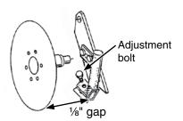
Adjust liquid drop tube/scraper so there is slight contact between blade and scraper lower leading edge, and ½" (0.6 cm) clearance between liquid drop tube trailing edge and blade. Blade should turn with minimum amount of drag.
