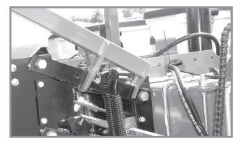
Lift lever positioned on push row unit
