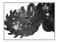
Residue wheels attach to row unit mounted coulter with two cap screws and sleeves allowing unit to free-float. A 2-position spindle bolt mounting positions wheels interlocked or staggered. Depth adjustment is made with a spring-loaded cam and pin with 11 positions in ¼" (0.6 cm) increments. A high point on the cam allows wheels to be locked up.
