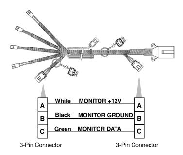
Light package meets ASABE Standards. For correct wiring harness to be wired into lights on your tractor, check with tractor manufacturer.
