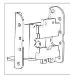
NOTE: Four center row units require special mount and extension brackets when using Frame Mounted Coulter W/Residue Wheels.
