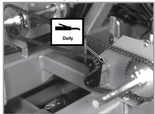
Squeeze pump drive plate - 1 per idler
