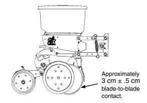
NOTE: Proper blade clearance is critical. Blades should have 1"  $\pm$  ½" (3  $\pm$  .5 cm) contact in this area. When blades are turned by hand in opposite directions against each other, there should be only light resistance to turning. Re-adjust blade scraper if necessary to center it between the blades.
