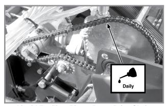
**Liquid Fertilizer Piston Pump Drive Chain**
