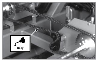
Liquid Fertilizer Squeeze Pump Drive Chain INTERPLANT PUSH ROW UNIT LOCKUPS
