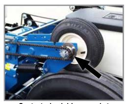
Contact wheel drive sprocket
