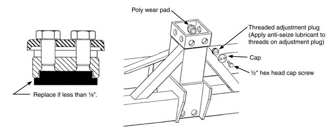
Planter center section consists of a steel tubular frame and 16 adjustable wear pad assemblies that travel up and down against a stainless steel clad center post. Each adjustable wear pad assembly consists of a poly wear pad, threaded adjustment plug, and cap. Assembly is held in place by the threaded adjustment plug and locked in place by the cap and two ½" hex head cap screws.
