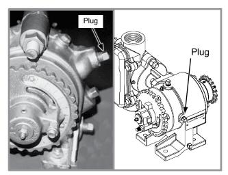
Piston pump oil fill plug location
