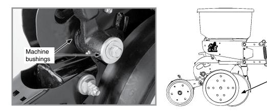
Shim gauge wheel to lightly contact opener disc blade. Check adjustment in field position.
