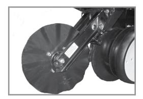
Row unit mounted no till coulters with 1" bubbled, 1" fluted (8 flutes) or  $\frac{3}{4}$ " fluted (13 flutes) blades may be used on pull row units and push row units ( $\frac{3}{4}$ " fluted shown). Four quick adjustable down force springs are required per row when using row unit mounted no till coulters. See "Quick Adjustable Down Force Springs Options".
