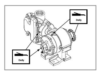
Liquid Fertilizer Piston Pump - 4 NOTE: Fill on outboard stuffing box until lubricant seeps out of drain hole in bottom.
