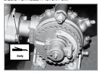
Piston Pump -2 NOTE: Fill on outboard stuffing box until lubricant seeps out of drain hole in bottom.
