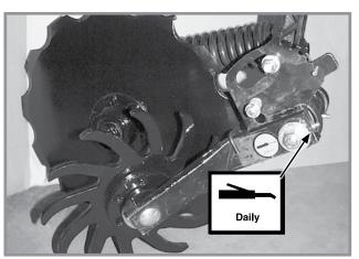
Residue Wheel Attachment For Use With Notched Single Disc Fertilizer Opener - 1
