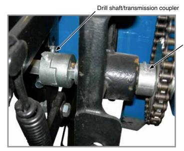
Transmission shaft and drill shaft coupler
