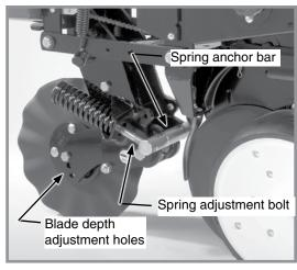
Frame mounted coulter adjustment
