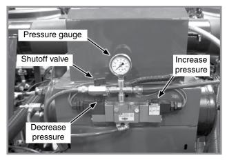
Air compressor assembly controls
