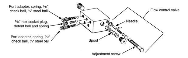
The valve block assembly consists of the row marker sequencing and flow control valves in one assembly. Sequencing valve portion consists of a chambered body containing a spool and series of check valves to direct hydraulic oil flow.
