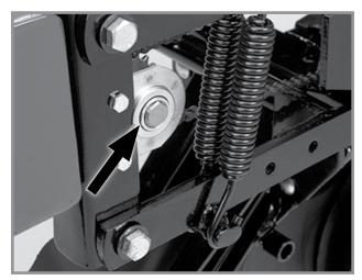
A number of sealed bearings are used on your Kinze planter to provide trouble free operation. These are located in such areas as the drive shaft, row units, and transmission bearings. Sealed bearings are lubricated for life and not serviceable.
