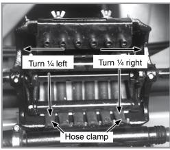
Adjusting squeeze pump end hoses
