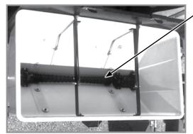
Flighting must move chemicals from center to outside of hopper.
