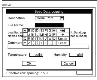
STEP 6 Use the knob or arrow keys to scroll to the "Comment for file" box. Press the knob or Enter key to display the drop down keyboard. Use the keyboard to enter a Comment for the file then press the Enter key.
