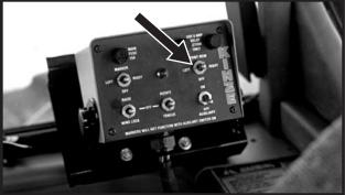
The selector switch for the clutches is located on the planter control console.
