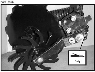
Residue Wheel Attachment For Use With Notched Single Disc Fertilizer Opener - 1 Zerk
