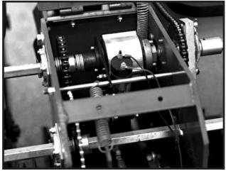
The right hand clutch operates clockwise and the left hand clutch operates counterclockwise. Therefore, some of the parts of the clutch such as the wrap spring differ from one side of the planter to the other. Be sure to use the correct repair part if a clutch must be repaired.
