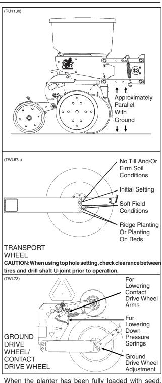
When the planter has been fully loaded with seed, granular chemicals, fertilizer, etc.; a field check should be made to be sure the wings are level with the center frame. If the wings are not level with the center frame, the drive wheels and/or transport wheels can be raised or lowered in the wheel arms to increase or decrease planter toolbar height. Hitch height should be raised accordingly to ensure level operation.
