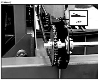
Squeeze Pump Drive Chain Idler - 1 Zerk Per Idler
