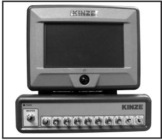
The Cobalt electronic seed monitor system consists of a console, which is mounted on the tractor; seed tubes with computerized sensors, one of which is installed in each planter row unit; a primary harness, which connects the console to the planter harness; and a planter harness (junction Y-harness and/or harness extension where applicable), to which the individual seed tube sensors connect.
