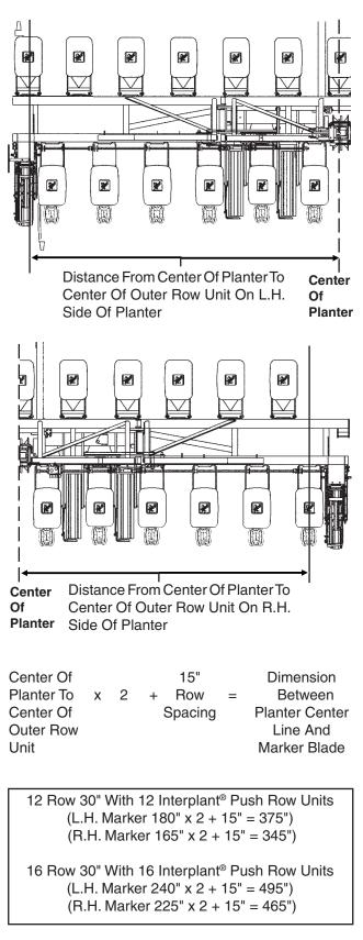
NOTE: If tractor hitch is offset 7  $\frac{1}{2}$ " to the right of the center line of the tractor, add 7  $\frac{1}{2}$ " to the marker dimension on the R.H. side of the planter and subtract 7  $\frac{1}{2}$ " from the marker dimension on the L.H. side of the planter.
