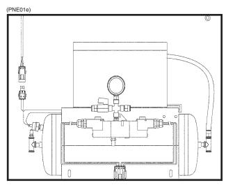
Air Compressor With Dual Solenoid Assembly
