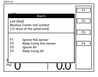
NOTE: When a known sensor or group of sensors are faulty, F1 or F3 should be pressed. The monitor will stop communication with the sensor(s) and the corresponding bargraphs will be grayed out on the main "Planter Configuration" screen as shown below.
