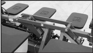
Hold the control console switch labeled "RAISE/ WING LOCK" in "RAISE" and operate the hydraulic control until the two center lift cylinders are fully extended and the safety hook located at the top of the center section rotates into locking position.
