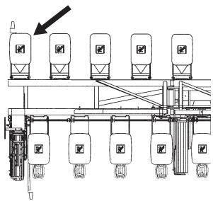
An Even-Row Push Row Unit Package is available to add one additional push row unit onto the L.H. side of the outer end of the front toolbar for use along with the Solid Row Interplant<sup>®</sup> Package.
