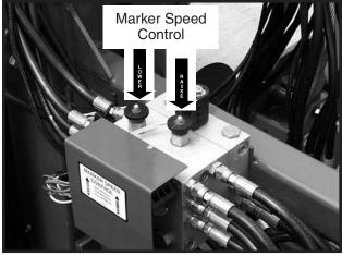
IMPORTANT: The flow controls should be properly adjusted before the marker assembly is first put into use. Excessive travel speed of the markers can damage the marker assembly.
