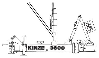
12 Row 30"/36"/38" And 16 Row 30" - "T" And "Y" Hitches Part No. G7100-259 Amber Reflective Decal (Qty. 2 - 1 Located On Each Side Of Hitch)
