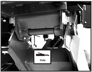
2. Wing Wheel Pivot - 2 Zerks Per Wheel Module 81439-29
