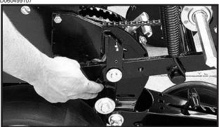
3. Using the lift lever, raise the push row unit to allow the spring loaded lockups to snap out of locked position. Lower row unit to the ground.
