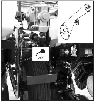
Liquid Fertilizer Ground Drive Chain (Piston Pump)
