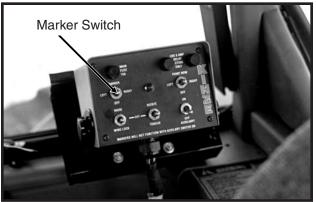
Three Position Selector Switch On Control Console
