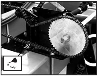
Liquid Fertilizer Drive Chains (Squeeze Pump)
