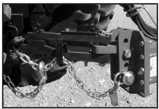
NOTE: A 2-Point Hitch Option, which converts the planter from drawn to semi-mounted, is available for use with Category 3N or 3 three-point hitch designs. The safety chain is not applicable with the 2-point hitch.
