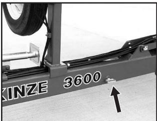
**Tongue Safety Pin Installed For Transport**
