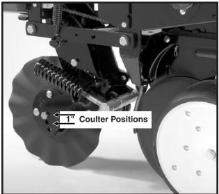
Frame mounted coulters with 1" bubbled, 1" fluted (8 flutes) or  $\frac{3}{4}$ " fluted (13 flutes) blades may be used on pull row units only. (Not compatible with push row units.)
