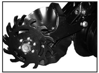
The wheel hubs are equipped with sealed bearings. If bearings sound or feel rough when the wheel is rotated, replace the bearings.
