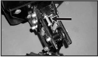
A full threaded bolt and jam nut located on the upper link allows maximum depth to be set for loose soil conditions. Initial setting should be 1 <sup>3</sup>/<sub>4</sub>" above the depth of the row unit double disc opener.
