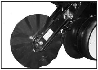
Check periodically to be sure nuts and hardware are tightened to proper torque specification.
