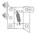
To adjust down force springs, raise the row unit out of the ground and reposition springs as shown for the desired down pressure. D101701112
