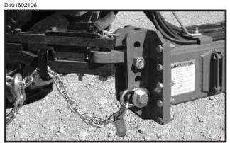
Four holes in the hitch bracket allow the clevis to be raised or lowered. In addition, the clevis may be turned over for a finer adjustment between mounting holes. When installing the clevis mounting bolt, make sure the lock nut is torqued to 840 ft./lbs.
