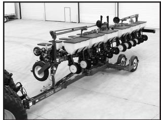
1. With the <u>tongue fully extended</u> and the <u>planter in</u> <u>the raised transport position</u>, remove the tongue safety pin and store it in the storage position.
