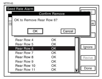
Press the knob or Enter key to confirm removal. The Sensor Setup screen will display "none" next to the row that was removed. Press the F6 key next to "Done". The setup mode screen will appear.
