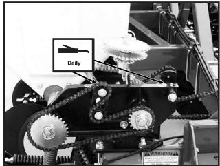
Fertilizer Transmission - 2 Zerks Per Transmission
