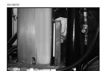
(g) Remove old pads and install new pads. NOTE: Apply a small amount of weather stripping adhesive to hold the pads in place while the pad holder is being reinstalled.
