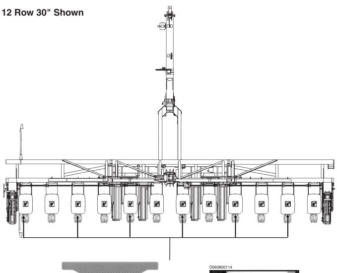
Part No. G7100-262 Amber Reflective Decal (Located On The Hopper Support On Every Other Row Unit Beginning On The 1st Row Unit On The L.H. End Of The Planter - Side-Facing In Transport Position) **(Standard)**
