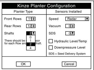
STEP 7 Turn the knob or use the arrow keys to advance to the "Speed" field. Press the knob or Enter key and a drop down menu will appear; select either "Radar" or "Coil Pick-Up" (MDS) by turning the knob or using the arrow keys. When the desired selection is highlighted press the knob or Enter key.
