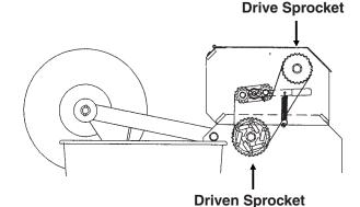
NOTE: Since the two-speed point row clutch is located ahead of the liquid fertilizer squeeze pump and/or dry fertilizer drive, activating the two-speed point row clutch reduced rate switch will cause the same per cent of reduction in dry fertilizer or liquid fertilizer (squeeze pump) application rates. Liquid fertilizer (piston pump) application rates will not be affected as the piston pump uses a dedicated drive tire.
