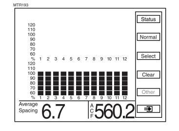
NOTE: The abbreviation for the selected area counter will appear in the bottom R.H. corner of the screen. In the above illustration "ACF" stands for Area Counter Field.
