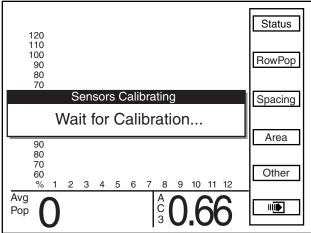
NOTE: Do not attempt planting before the "Wait For Calibration" message disappears. If the planter is moving while sensors are calibrating alarms will be generated.
