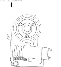
NOTE: To adjust gap between actuator arm and stop, loosen nut on mounting pin and move pin in slot until there is  $\frac{1}{3}$ "( $\pm\frac{1}{32}$ ") gap between arm and stop on stop collar. Retighten nut.
