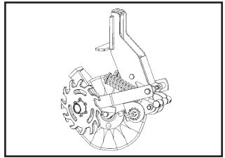
The wheel hub is equipped with sealed bearings. If a bearing sounds or feels rough when the wheel is rotated, replace the bearings.
