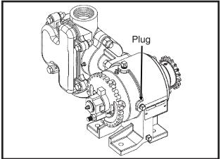
Check crankcase oil daily and maintain at plug level. Fill as needed with EP 90 weight gear oil. Total oil capacity is approximately <sup>3</sup>/<sub>4</sub> pint.
