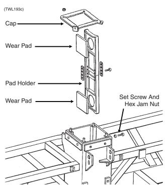
The center section of the planter is contructed around a steel tubular frame with four wear pad assemblies that ride against a stainless steel clad center post. Each wear pad assembly includes a pad holder and two wear pads. The wear pads are held by the pad holder and locked in place by  $\frac{3}{4}$ " set screws and hex jam nuts.
