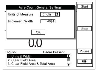
STEP 6 Turn the knob or use the arrow keys to highlight the correct value then press the knob to select the number, for numbers containing more than one digit select one digit at a time. When the desired quantity is displayed above the number pad, press the Enter key.
