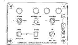
The raise/wing lock and rotate/tongue (fold function) switches are MOMENTARY ON-OFF-MOMENTARY ON type and must be held in position while operating the tractor hydraulic lever. Activating a fold function switch disables the marker circuit.
