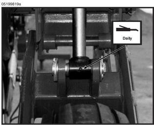
10. Wing Lift Cylinders - 1 Zerk Per Cylinder
