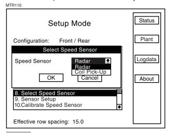
STEP 3 Turn the knob or use the arrow keys to highlight the "OK" button and press the knob or Enter key to return to the "Setup Mode" screen.
