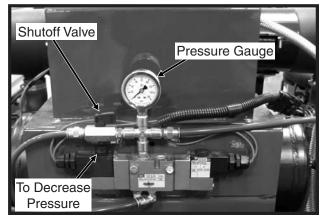
To lock up push row units equipped with pneumatic down pressure springs:
