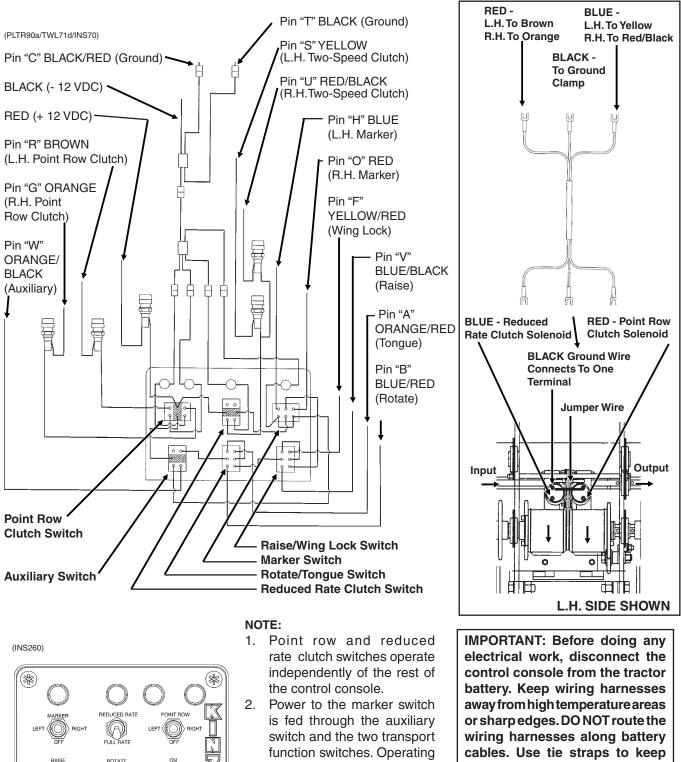
switch and the two transport function switches. Operating any of the switches in the lower row disables the marker function and turns off the panel light for the markers.
