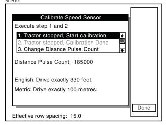
• In field conditions, measure 330 feet or 100 meters, depending on the unit of measurement selected. Place a marker at the start point and end point.
