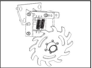
The wheel hub is equipped with sealed bearings. If a bearing sounds or feels rough when the wheel is rotated, replace the bearings.
