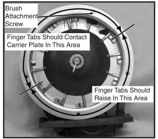
A buildup of debris or chaff may prevent proper finger operation and will require disassembly and cleaning of the finger pickup meter as follows:
