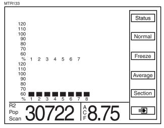
Press the F3 key next to Scan and the monitor will scan through each row in ascending order displaying the average seed population for each row. After all rows have been scanned the average population is displayed and scan function will continue with the first rear row.
