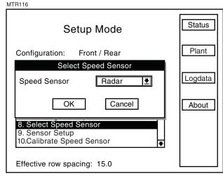
STEP 4 Press the knob or Enter key to select the "Speed Sensor" field and a drop down menu will appear.
