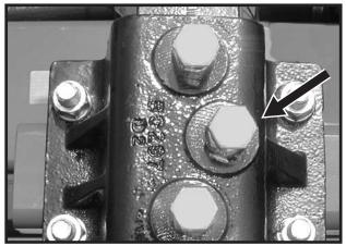
NOTE: Recommended maximum operating depth is 4". To adjust depth: (a) Loosen depth adjustment cap screws. (b) Adjust depth to desired setting. (c) Tighten upper and lower cap screws slightly to hold opener arm in place. (d) Tighten middle cap screw to set the opener arm angle. (e) Tighten upper and lower cap screws and all jam nuts.
