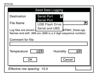
STEP 3 Use the knob or arrow keys to highlight the "File Name" box. Press the knob or Enter key and a drop down list of the files will be displayed. Select "Add new ... " to enter a file name and press the knob or enter key to display a keyboard.
