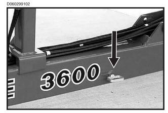
9. Install transport latch locking pin.
