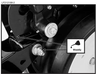
Row Unit "V" Closing Wheel, Covering Discs/ Single Press Wheel And/Or Drag Closing Wheel Eccentric Bushings (2 Per Row)
