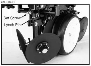
Vertical adjustment in  $\frac{1}{3}$ " increments is possible by removing the lynch pin which secures the vertical support arm and moving the support arm up or down as required. Reinstall lynch pin. Finer adjustment can be attained by removing the lynch pin and using the  $\frac{5}{8}$ " x 2  $\frac{1}{4}$ " set screw to clamp the support arm in the required position.
