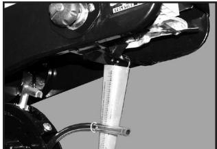
To check, fill insecticide and/or herbicide hoppers. Attach a calibrated vial to each granular chemical meter. Lower the planter and proceed as follows.
