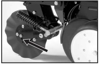
NOTE: Torque 5/8" spindle hardware to 120 ft. lbs.
