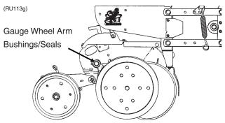
NOTE: A Gauge Wheel Arm Bushing And Seal Driver Kit (G1K296), for use in bushing and seal replacement, is available through your KINZE<sup>®</sup> Dealer.
