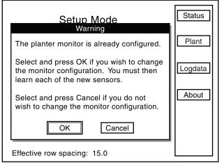
NOTE: To prevent the configuration from being changed, select Cancel, then press the knob, Enter key or ESC key.
