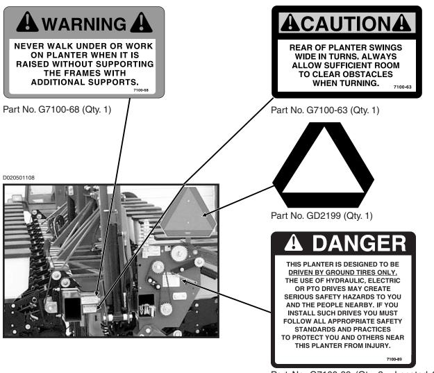
Part No. G7100-89 (Qty. 2 - Located On Wheel Modules On Both Ends Of Planter)
