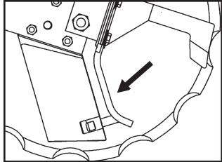
NOTE: Adjusting the liquid drop tube will ensure it is out of the path of the soil flow across the knife. Drop tube and tab will wear quickly if not adjusted correctly.
