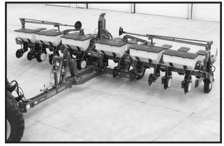
3. Hold the control console switch labeled "ROTATE/ TONGUE" in "**TONGUE**" and operate the hydraulic control until the tongue is fully extended. Tongue lock latch will automatically release.
