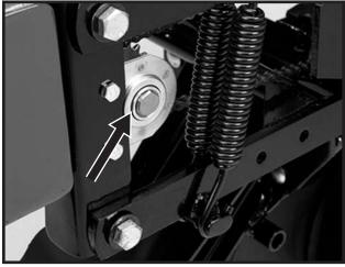
A number of sealed bearings are used on your KINZE<sup>®</sup> planter to provide trouble free operation. These are located in such areas as the drive shaft, row units and transmission bearings. Sealed bearings are lubricated for life. Due to the seals, relubrication is not practical.
