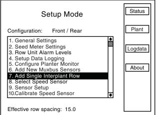
STEP 2 To confirm the note below turn the knob or use the arrow keys to highlight the "OK" button, then press the knob or Enter key to confirm. If the single Interplant<sup>®</sup> row is not to be added select the "Cancel" key and press the knob or Enter key to cancel or press the ESC key.
