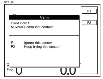
If multiple sensors have lost contact, the message will indicate which sensors have lost contact, see below.
