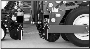
With the planter lowered to operating height, check to be sure the frame is level fore and aft. Recheck once planter is in the field.
