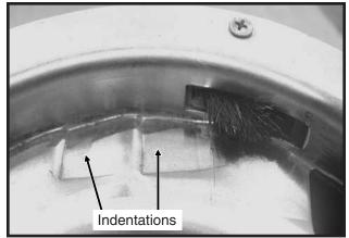
**Photo Shows Worn Carrier Plate**
