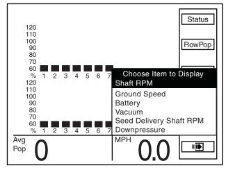
• Press the F5 key next to Other to display items available to display in the bottom R.H. corner. Turn the knob or use the arrow keys to highlight "Shaft RPM". The value will appear in the bottom R.H. corner of the display as "RPM".
