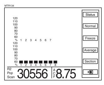
• Press the F3 key next to Freeze to stop scanning, the left display item will be frozen on a particular row. "Frzn" appears in the lower L.H. corner to indicate the display is frozen. To resume scan press the F3 key next to Scan.
