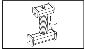
NOTE: The piston pump ground drive wheel assembly is designed to allow the assembly to be locked in raised position when not in use. Remove the two cap screws that attach the upper end of the spring to the spring mount. Reattach the spring using the upper holes in the spring mount. Reverse procedure to reset for field use.
