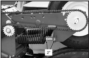
There are two down pressure springs on each contact drive wheel. The down pressure is factory preset and should require no further adjustment.
