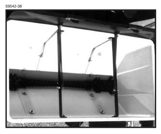
Check auger installation by rotating shaft in the direction of planter travel to see that the spirals on the auger move toward the ends of the hopper. If not, remove auger assembly, turn 180° and reinstall.
