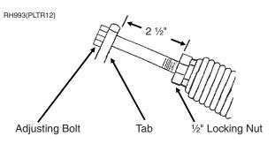
Eccentric bushings in the wheel arm stop allow for lateral adjustment of the covering discs/single press wheel assembly. Using a  $\frac{3}{4}$ " wrench, loosen the hardware which attaches the assembly to the wheel arm stop. Using another  $\frac{3}{4}$ " wrench, turn the eccentric bushings until the press wheel is aligned with the seed trench. (RU94b)
