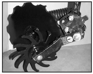
The residue wheel attachment for the notched single disc fertilizer opener is designed for applications where row unit mounted residue wheel attachments cannot be installed. The residue wheel is attached to the notched single disc fertilizer opener using  $\frac{5}{2}$ " x 7  $\frac{1}{2}$ " and  $\frac{1}{2}$ " x 6  $\frac{1}{2}$ " hardware.
