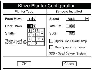
STEP 6 Rotate the knob or use the arrow keys to advance to "Shafts" field. Press the knob or Enter key to select the "Shaft" field. A drop down menu will appear. Turn the knob or use the arrow keys to highlight the number of "Shafts" on the planter. When the correct value is displayed, press the knob or Enter key to return to the "Kinze Planter Configuration" screen.
