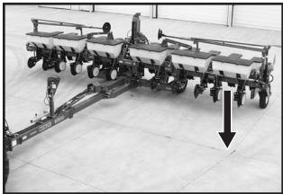
Hold the control console switch labeled "RAISE/ WING LOCK" in "WING LOCK" and operate the hydraulic lever to release the wing locks.
