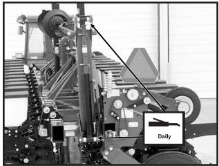
1. Row Marker Assemblies - 4 Zerks Per Assembly On 8 Row Wide And 12 Row 30". 2 Zerks Per Assembly On 12 Row Wide And 16 Row 30".
