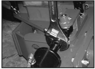
(p) Reset row unit down pressure and other attachments from STEP c.
