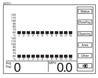
NOTE: The Planter Configuration screen displays the planter rows as programmed into the KPM III software. The above screen shows 12 front (Interplant®) rows and 12 rear rows. If the KPM III were programmed for 8 front (Interplant®) rows and 8 rear rows the screen would display 8 front and 8 rear rows.
