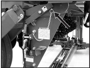
Transport Latch Locking Pin Installed For Transport
