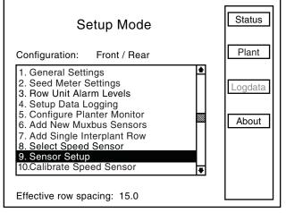
STEP 4 Turn the knob or use the arrow keys to highlight the faulty sensor and press the F2 key next to Remove.
