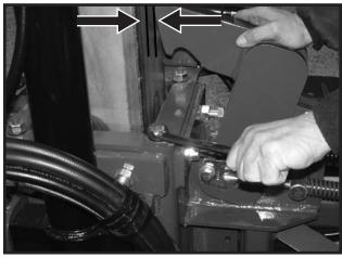
(m) Adjust stop on safety hook. Maximum clearance should be  $1\!\!/_2$ " and minimum clearance  $1\!\!/_8$ " as shown above.
