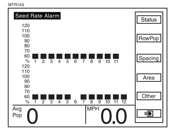
If the sensor is detecting no seed flow it will display which row is not functioning. The alarm may be caused by a mechanical problem reducing seed flow or an electrical problem causing an incorrect seed count. MTR144
