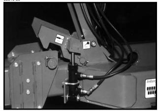
Hold the control console switch labeled "RAISE/ WING LOCK" in "WING LOCK" and operate the hydraulic lever until the wing lock cylinders are fully extended and the wing locks are locked over center.
