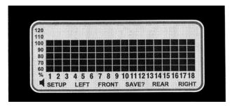
The monitor collects data on the planting rates from all active rows and calculates an average. This average will determine the 100% mark. Seed rate for each row is then compared to the average value and the result is displayed on the bar graph.
