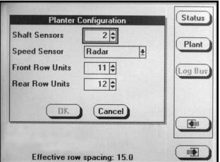
NOTE: The numeric value may be changed only if the item is highlighted. Turning the rotary encoder knob increases or decreases the value of the item. The UP arrow key may be used to increase the value of the item by one and the DOWN arrow key may be used to decrease the value of the field by one.
