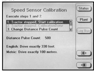
NOTE: A field calibration must be performed to establish the Distance Pulse Count number. Several factors can affect this value, such as wheel slip on the magnetic distance sensor. IT IS NOT UNCOMMON FOR THE SPEED ON THE MONITORTOVARY SLIGHTLY FROMTHETRACTOR SPEEDOMETER. Adjusting the Distance Pulse Count in the monitor to make the speed agree with the tractor can cause serious errors in acre/hectare and population/spacing readings. Do field checks to verify populations and seed spacing.
