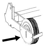
Transport wheel rock guards are designed for use on both sides of each of the four center transport wheels when the planter is used in rocky conditions. Rock guards will help prevent rocks, which can cause damage to the row units, from being picked up by the wheels.
