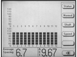
Press the SHAFT key to view the average meter shaft RPM. The value will appear in the bottom R.H. corner of the display.
