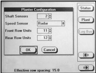
NOTE: To prevent the configuration from being saved press ESC or select the CANCEL button, then press the rotary encoder knob or ENTER key.
