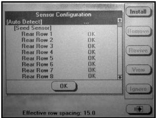
STEP 6 If "OK" appears behind <u>ALL</u> sensors, press the knob or the ENTER key to save the configuration. The "Setup Mode" menu will then appear.
