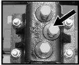
NOTE: Recommended maximum operating depth is 4". To adjust depth: (a) Loosen depth adjustment cap screws. (b) Adjust depth to desired setting. (c) Tighten upper and lower cap screws slightly to hold opener arm in place. (d) Tighten middle cap screw to set the opener arm angle. (e) Tighten upper and lower cap screws and all jam nuts.
