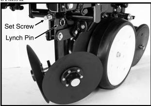
Vertical adjustment in ½" increments is possible by removing the lynch pin which secures the vertical support arm and moving the support arm up or down as required. Reinstall lynch pin. Finer adjustment can be attained by removing the lynch pin and using the 5%" x 2 ½" set screw to clamp the support arm in the required position.
