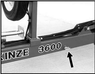
Tongue Safety Pin Installed For Transport
