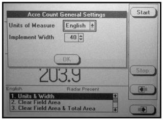
STEP 4 Press the knob or ENTER key to highlight the field. Turn the knob or use the UP or DOWN arrow keys to select desired number in feet. When desired number is obtained press the knob or ENTER key. The black box will advance to OK key.
