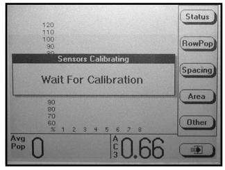
NOTE: Do not attempt planting before the "Wait For Calibration" message disappears. If planter is moving while sensors are calibrating alarms will be generated.
