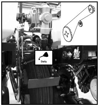
**Liquid Fertilizer Ground Drive Chain (Piston Pump)**
