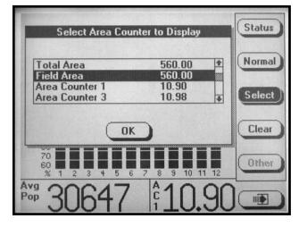
STEP 4 Press the knob or ENTER key to select OK. The planting screen will then be displayed. Press NORMAL to display main planting screen.
