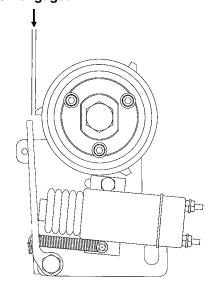
NOTE: To adjust gap between actuator arm and stop, loosen nut on mounting pin and move pin in slot until there is  $\frac{1}{8}$ "( $\pm\frac{1}{32}$ ") gap between arm and stop on stop collar. Retighten nut.
