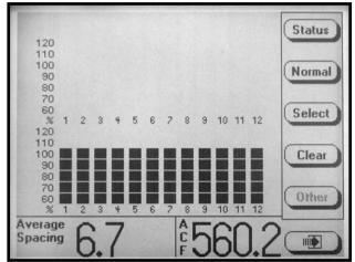
NOTE: The abbreviation for the selected area counter numerical value will appear in the bottom R.H. corner of the screen. In the above photo "ACF" represents "Area Counter Field".
