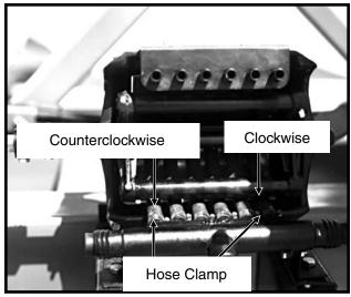
For the right hand hose (facing the pump from front as shown above) twist the hose  $\frac{1}{4}$  turn in the clockwise direction.
