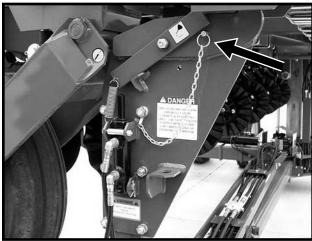
10. Remove manual safety bar from its storage location on the left side of the axle assembly and position it behind the front center lift cylinder.
