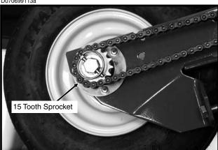
Half rate (2 to 1) drive is recommended only when desired population falls below that shown on planting rate charts. Replace the 30 tooth sprocket on each contact wheel with a 15 tooth sprocket and shorter No. 40 110 pitch chain. This will reduce the planter transmission speed and reduce planting and application rates by approximately 50%.
