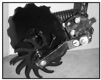
The residue wheel attachment for the notched single disc fertilizer opener is designed for applications where row unit mounted residue wheel attachments cannot be installed. The residue wheel is attached to the notched single disc fertilizer opener using \%" x 7 1/2" and 1/2" x 6 1/2" hardware.
