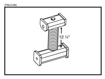
NOTE: The piston pump ground drive wheel assembly is designed to allow the assembly to be locked in raised position when not in use. Remove the two cap screws that attach the upper end of the spring to the spring mount. Reattach the spring using the upper holes in the spring mount. Reverse procedure to reset for field use.
