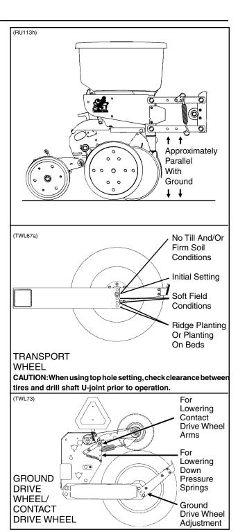
When the planter has been fully loaded with seed, granular chemicals, fertilizer, etc.; a field check should be made to be sure the wings are level with the center frame. If the wings are not level with the center frame, the drive wheels and/or transport wheels can be raised or lowered in the wheel arms to increase or decrease planter toolbar height. Hitch height should be raised accordingly to ensure level operation.
