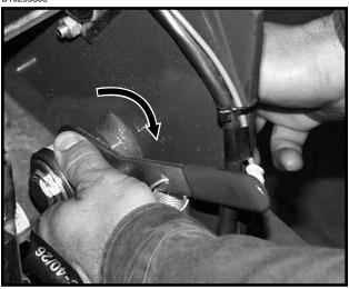
To add chain tension, rotate chain idler into the chain while rotating handle to tension idler spring.
