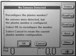
NOTE: Selecting OK will reconfigure the monitor requiring all sensors to be re-learned. Selecting CANCEL will maintain the current configuration and the monitor will continue trying to communicate with the sensors.
