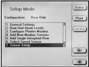
STEP 4 Highlight faulty sensor. Press REMOVE key and unplug sensor. Plug in new sensor and press INSTALL key.
