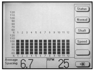
• Press the SPEED key to view the ground speed. The value will appear in the bottom R.H. corner of the display.
