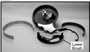
The lower brush has several functions. One function is to move seed down the seed loading slots to the seed pockets. The second function is to isolate seed in the reservoir from entering the seed tube and a third is to clean the seed loading slots.
