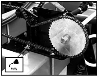
**Liquid Fertilizer Drive Chains (Squeeze Pump)**
