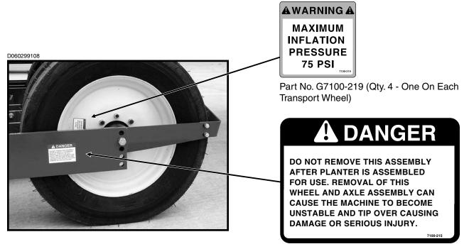
Part No. G7100-215 (Qty. 1 - Located On Rear Side Of Stub Axle)
