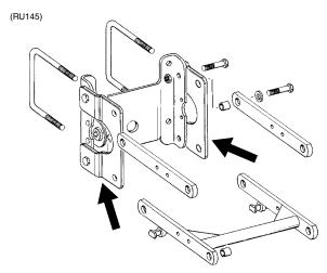
Row unit extension brackets are required on the 4 center pull row units if the Model 3600 planter is equipped with coulter mounted residue wheels. The brackets extend the row units rearward 4" to provide required clearance.
