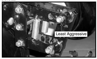
To lock the residue wheel up out of the ground, remove the  $\frac{1}{2}$ " x 5" lockup bolt, raise the residue wheel and install bolt.
