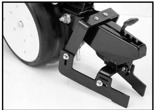
The drag closing attachment is designed to pull loose soil over the seed trench.
