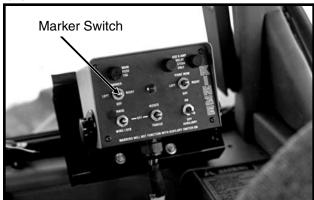
Three Position Selector Switch On Control Console
