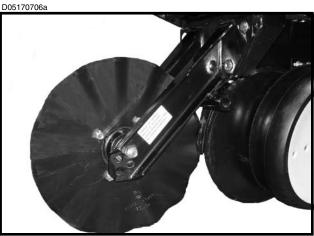
STYLE B (One Sleeve For Installing Coulter Mounted Residue Wheels)
