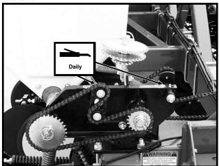
Fertilizer Transmission - 2 Zerks Per Transmission
