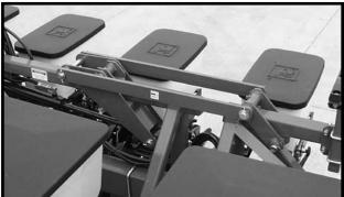
5. Hold the control console switch labeled "RAISE/ WING LOCK" in "RAISE" and operate the hydraulic lever until the two center lift cylinders are fully extended and the safety hook located at the top of the center section rotates into locking position.
