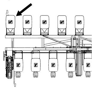
An Even-Row Push Row Unit Package is available to add one additional push row unit onto the L.H. side of the outer end of the front toolbar for use along with the Solid Row Interplant® Package.
