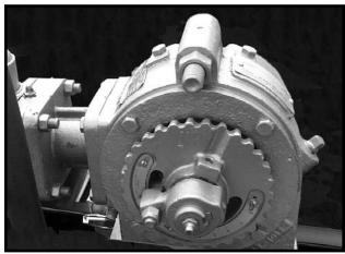
If the machine is equipped with the piston pump option, the rate of liquid fertilizer application is determined by the piston pump settings.
