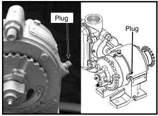
Check crankcase oil daily and maintain at plug level. Fill as needed with EP 90 weight gear oil. Total oil capacity is approximately ¾ pint.
