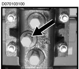
NOTE: Recommended maximum operating depth is 4". To adjust depth: (a) Loosen depth adjustment cap screws. (b) Adjust depth to desired setting. (c) Tighten upper and lower cap screws slightly to hold opener arm in place. (d) Tighten middle cap screw to set the opener arm angle. (e) Tighten upper and lower cap screws and all jam nuts.
