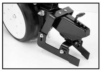
Prior to storage of the planter, inspect each drag closing attachment and replace any worn or broken parts. Check for loose hardware and tighten as needed.
