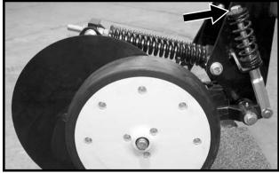
NOTE: The soil press wheel is not intended to be used for gauging fertilizer opener operating depth.
