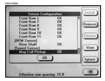
Turn the knob or use the UP or DOWN arrow keys to select "Select Speed Sensor" and press the knob or ENTER key. Press the knob or ENTER key to select the "Speed Sensor" field and a drop down menu will appear. Turn the knob or use the UP or DOWN arrow keys to select "Coil Pick-Up" and press the knob or ENTER key to make selection. The black box will advance to OK press the knob or ENTER key to save the information.
