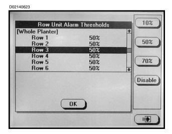
The alarm thresholds can be set for the whole planter, any planter section or individual rows.
