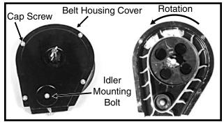
If the belt is being replaced, make sure it is installed to correctly orient the paddles as shown. A diagram molded into the drive sprocket also illustrates the correct orientation.
