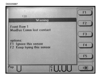
If multiple sensors have lost contact, the message will indicate which sensors have lost contact.
