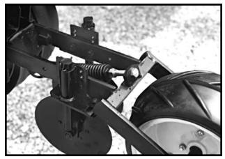
After adjusting planting depth, check the operation of the covering discs/single press wheels.
