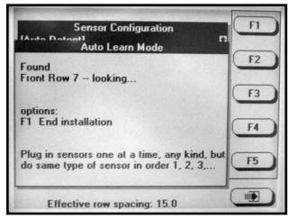
NOTE: After each sensor has been installed "OK" will appear after the sensor name.
