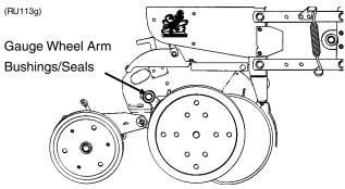
NOTE: A Gauge Wheel Arm Bushing And Seal Driver Kit (G1K296), for use in bushing and seal replacement, is available through your KINZE® Dealer.
