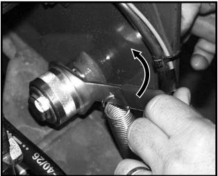
The wrap spring wrenches are made in L.H. and R.H. configurations, which can be identified by the silver or gold release collars, respectively.
