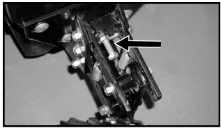
A full threaded bolt and jam nut located on the upper link allows maximum depth to be set for loose soil conditions. Initial setting should be 1 ¾" above the depth of the row unit double disc opener.
