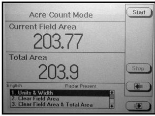
STEP 3 A drop down menu will appear. Select the correct units of measure "English" or "Metric" by turning the knob or using the UP or DOWN arrow keys. Press the knob or ENTER key to make the selection. The black box will advance to "Implement Width" field showing implement width in feet.
