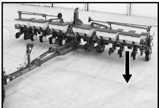
7. Hold the control console switch labeled "RAISE/WING LOCK" in "WING LOCK" and operate the hydraulic lever to release the wing locks.
