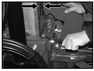
(m) Adjust stop on safety hook. Maximum clearance should be  $1\!\!/\!_2$  and minimum clearance  $1\!\!/\!_8$  as shown above.
