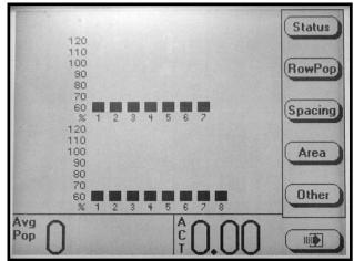
If the monitor does not detect any sensors the message shown below will appear.
