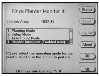
Either select the "Planting Mode" by turning the knob or using the UP arrow key and press the knob or ENTER key or press F6 to return to the "Planting Mode".
