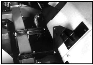
At the end of the planting season, or when the fertilizer attachment is not going to be used for a period of time, the hoppers should be disassembled, cleaned and coated with a rust preventative.
