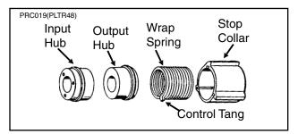
The point row clutch consists of a wrap spring riding on an input hub and an output hub. During operation the wrap spring is wrapped tightly over the hubs connecting them in a positive engagement. The greater the force of rotation the tighter the grip of the spring on the hubs.
