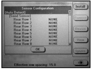
NOTE: Highlighting a sensor and pressing VIEW gives additional information when troubleshooting a problem. If a faulty sensor has been ignored it may be highlighted in the list of sensors, press REVIVE. The monitor will try to communicate with the sensor. If successful, "OK" will appear next to the sensor.
