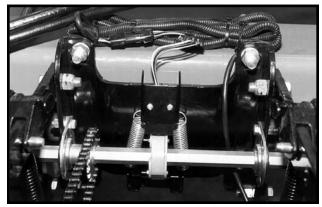
"LSHAFT" or "SHAFT 1" will display on the lower LCD when the first shaft rotation sensor is installed. "RSHAFT" or "SHAFT 2" will display when the second shaft rotation sensor is installed.
