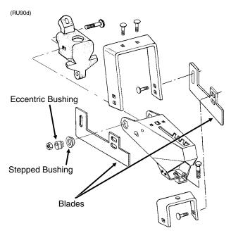
Eccentric bushings allow for lateral adjustment of the drag closing attachment. Using a ¾" wrench, loosen the hardware which attaches the assembly to the wheel arm stop. Using another ¾" wrench, turn the eccentric bushings until the drag closing attachment is aligned with the seed trench.
