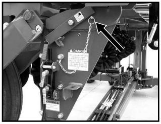
**Transport Latch Locking Pin Installed For Transport**
