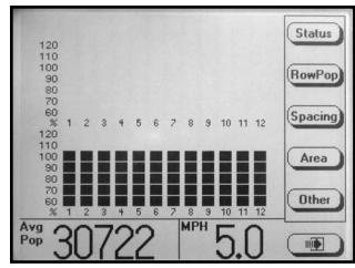
Press the SCAN key and the monitor will scan through each row in ascending order displaying the average seed population for each row. After all rows have been scanned the average population is displayed and scan function will continue with the first rear row.
