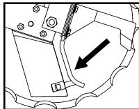
NOTE: Adjusting the liquid drop tube will ensure it is out of the path of the soil flow across the knife. Drop tube and tab will wear quickly if not adjusted correctly.
