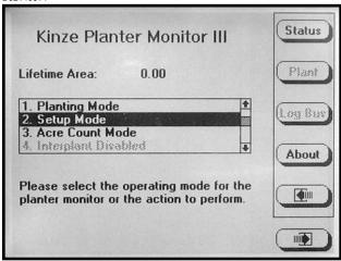
STEP 2 Turn the knob or use the UP or DOWN arrow keys to choose "Sensor Setup". Turn the knob or use the UP or DOWN arrow keys to highlight "Mag Coil Pickup". Press the REMOVE key, a note will appear for confirmation select as appropriate. Unplug Magnetic Distance Sensor and press the knob or ENTER key to save the information.
