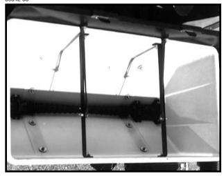
Check auger installation by rotating shaft in the direction of planter travel to see that the spirals on the auger move toward the ends of the hopper. If not, remove auger assembly, turn 180° and reinstall.
