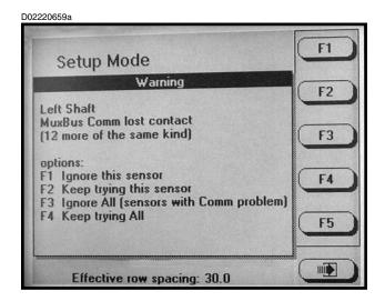
NOTE: When it is known that a sensor or a group of sensors are faulty, F1 or F3 should be pressed. The monitor will no longer try to communicate with the sensor(s). In the planting mode the corresponding bargraphs will be grayed out in the main screen.
