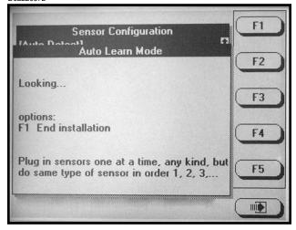
STEP 8 When all sensors are learned select F1 to end installation. Scroll down to verify the front rows are learned. Select OK by pressing the knob or ENTER key.
