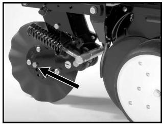
NOTE: Torque %" spindle hardware to 120 ft. lbs.
