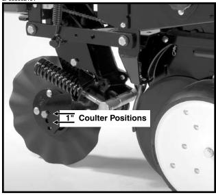
Frame mounted coulters with 1" bubbled, 1" fluted (8 flutes) or 3/4" fluted (13 flutes) blades may be used on pull row units only. (Not compatible with push row units.)
