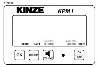
NOTE: Model 3600 planters will use the rear/front configuration only. When all rows can be viewed on a single display (rear), pressing the select key has no function.
