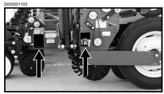
With the planter lowered to correct operating height, check to be sure the frame is level fore and aft. Recheck once planter is in the field.
