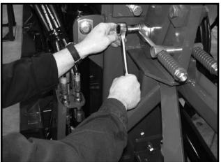
(n) Rotate cam roller against front guide and tighten to 200 ft. lbs. Make sure gap between roller guide and center frame are equal on both sides. (o) Raise planter out of the roller guides and lower back down into roller guides to be sure the roller guides operate smoothly. If not, adjust the roation cylinder rod as shown below.
