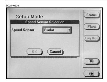
NOTE: To prevent the configuration from being changed select CANCEL, then press the rotary encoder knob, ENTER key or ESC key.
