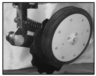
The depth/gauge wheel attachment for the notched single disc fertilizer opener is designed for use in situations where additional gauging is required to maintain desired fertilizer opener depth. The depth/gauge wheel is attached to the notched single disc fertilizer opener using a mounting block fastened to the pivot arm using 5%" hardware through the disc blade hub w/bearing.
