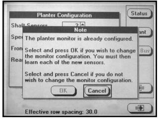
NOTE: To prevent the configuration from being changed select CANCEL, then press the knob, ENTER key or ESC key.
