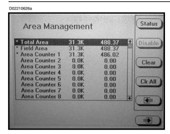
NOTE: If the total area is highlighted and the CLEAR key is pressed the following request for confirmation will appear.
