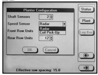
STEP 6 If there are front rows on the planter, press the knob or ENTER key to highlight the "Front Row Units" field. Turn the knob or use the UP or DOWN arrow keys to obtain correct number of push row units. Press the knob or ENTER key when desired quantity is displayed. The black box will advance to "Rear Row Units" field. If no front rows need to be entered simply turn the knob or press the DOWN arrow key to advance to "Rear Row Units".
