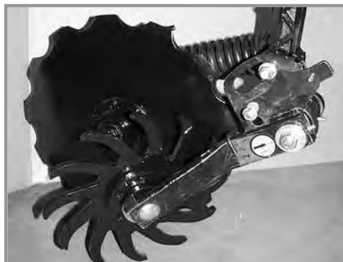
Notched single disc opener residue wheel attachment
