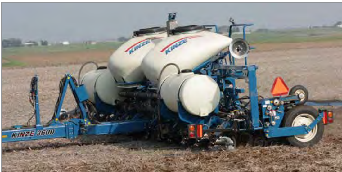
Liquid fertilizer installed on 3600 bulk fill
