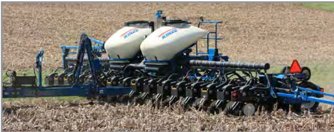
Model 3600 16 Row Planter with Vacuum Meter, Interplant, and Bulk Fill System
