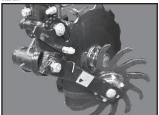
The residue wheel attachment for the notched single disc fertilizer opener is designed for applications where row unit mounted residue wheel attachments cannot be installed. The residue wheel is attached to the notched single disc fertilizer opener using  $\frac{5}{8}$ " x 3  $\frac{1}{2}$ " and  $\frac{1}{2}$ " x 1  $\frac{3}{4}$ " hardware.
