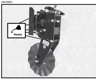
Frame Mounted Coulter Parallel Linkages - STYLE A (10 Per Row)
