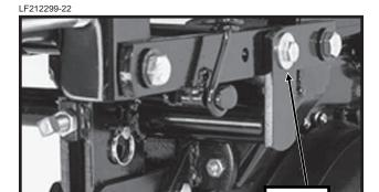
Row Unit Mounted Disc Furrower Parallel Linkages (6 Per Row)
