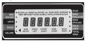
Press the UP or DOWN arrow keys to move the flashing arrow on the lower LCD to change what is displayed on the lower LCD.
