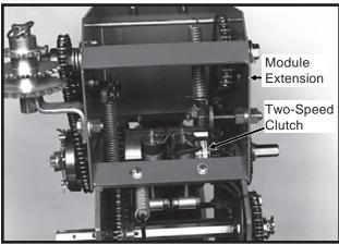
The Two-Speed Point Row Clutch Package is designed to allow on-the-go population rate adjustment as well as the capability to shutoff either half of the planter for finishing up fields or for long point row situations.
