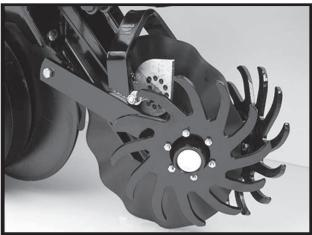
Coulter mounted residue wheels are designed for use on pull row units and push row units. Row unit extension brackets are required on the four center pull row units if the planter is equipped with coulter mounted residue wheels.
