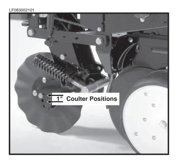
Frame mounted coulters with 1" bubbled, 1" fluted (8 flutes) or <sup>3</sup>/<sub>4</sub>" fluted (13 flutes) blades may be used on pull row units only. (Not compatible with push row units.)
