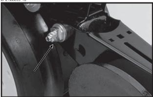
Bushings used for installation of the closing wheels can be moved from side to side for closing wheel spacing adjustment and the closing wheels can be installed in two locations either "offset" (to improve residue flow) or "directly" opposite. If set "directly" opposite, the forward installation holes should be used. Under normal conditions the narrow position is preferred.
