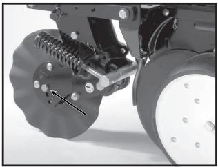
NOTE: Torque 5/8" spindle bolts to 120 ft. lbs.
