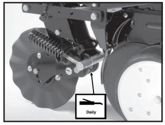
(If Applicable) Frame Mounted Coulter - STYLE B - 1 Zerk Per Arm
