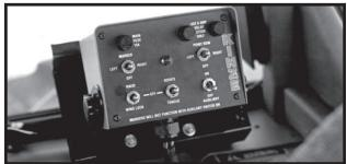
The tractor's hydraulic system and switches on the control console located on the tractor are used to raise the planter to transport position, operate the rotate and tongue extension functions, lock and release the planter wings, and raise and lower the row markers.
