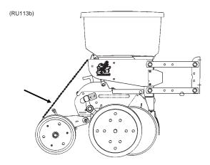
Plant a short distance and check to see if seed is visible in the seed trench. Adjust planting depth to a shallower setting if seed is not visible and recheck.
