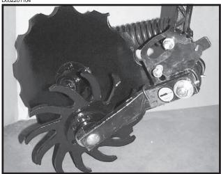
The residue wheel attachment for the notched single disc fertilizer opener is designed for applications where row unit mounted residue wheel attachments cannot be installed. The residue wheel is attached to the notched single disc fertilizer opener using  $^{5}/_{8}$ " x 7  $^{1}/_{2}$ " and  $^{1}/_{2}$ " x 6  $^{1}/_{2}$ " hardware.
