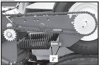
There are two down pressure springs on each contact drive wheel. The down pressure is factory preset and should need no further adjustment.
