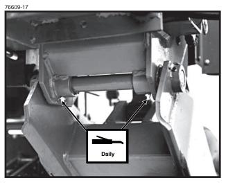
2. Wing Wheel Pivot - 2 Zerks Per Wheel Module
