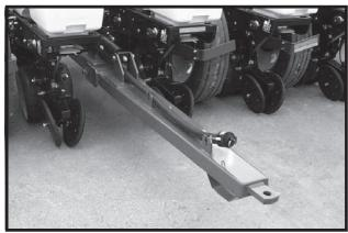
The Rear Trailer Hitch is used to tow a 3 or 4 wheel wagon behind the planter. A spring, chain and mounting bracket are used to support the 1 1/4" feed hose from the hitch to the piston pump. This extra length or loop is required to allow the planter to be moved into transport position without stretching the hose.
