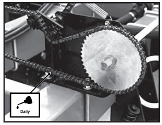
**Liquid Fertilizer Drive Chains (Squeeze Pump)**
