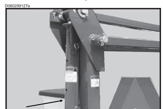
2. Using the hydraulic lever, raise the planter to the raised field position as shown below.
