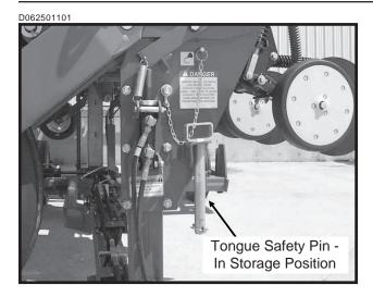
2. Remove the transport latch locking pin from the locked position and place it in the storage location.
