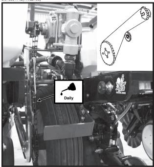
Liquid Fertilizer Ground Drive Chain (Piston Pump)
