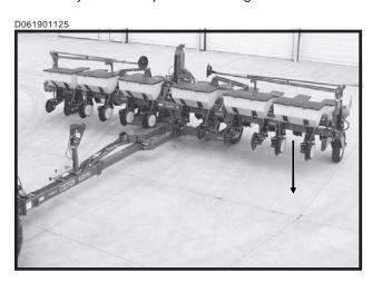
Hold the control console switch labeled RAISE/ WING LOCK in WING LOCK and operate the hydraulic lever to release the wing locks.
