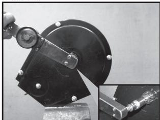
Turn finger holder by hand to make sure it is positioned firmly against the carrier plate, but is not over tightened and can be rotated with moderate force.
