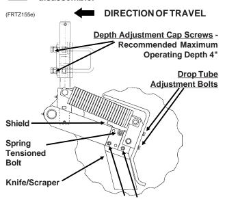
Knife/Scraper Leading Edge Adjustment Bolts (If not equipped with a shield and spring tensioned bolt, the third knife/scraper attachment bolt is also an adjustment bolt.)
