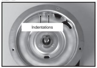
**Photo Shows Worn Carrier Plate**
