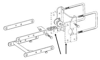
Row unit extension brackets are required on the 4 center pull row units if the Model 3600 planter is equipped with coulter mounted residue wheels. The brackets extend the row units rearward 4" to provide required clearance.
