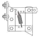
To adjust down force springs, raise the row unit out of the ground and reposition springs as shown for the desired down pressure.
