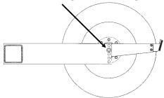
NOTE: The toolbar should operate at a 20-22" height measured from the bottom of the toolbar to the planting surface.
