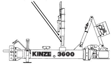
Part No. G7100-259 Amber Reflective Decal (Qty. 2 - 1 Located On Each Side Of Hitch) 12 Row 30"/36"/38" And 16 Row 30" - "T" And "Y" Hitches (If Applicable)
