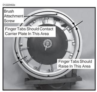
A buildup of debris or chaff may prevent proper finger operation and will require disassembly and cleaning of the finger pickup meter as follows:
