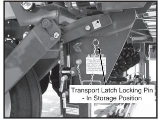
3. Remove the manual safety lockup from under the front center lift cylinder and place it in the storage location on the left side of the planter axle.
