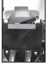
Part No. G7100-259 Amber Reflective Decal (Qty. 3 Used On 8 Row; 5 On 12 Row; 7 On 16 Row - Located On The Front Of Every Other Push Row Unit Beginning With The Center Row And Every Other Row To Both Ends - Side-Facing In Transport Position) (If Applicable)
