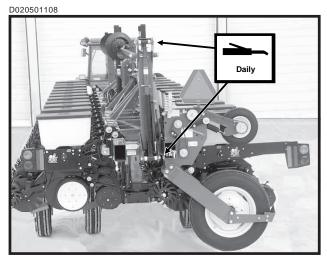
Row Marker Assemblies - 4 Zerks Per Assembly On 8 Row Wide And 12 Row 30". 2 Zerks Per Assembly On 12 Row Wide And 16 Row 30".
