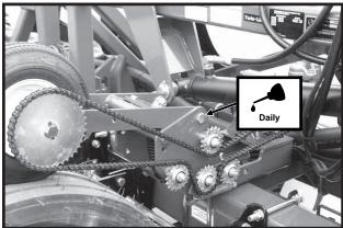
Optional Piston Pump Contact Drive Wheel Arm Assembly (2 Per Wheel Assembly)
