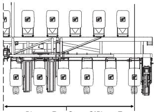
Center Of Planter To Of Center Of Outer Row Unit On R.H.
