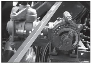
If the machine is equipped with the piston pump option, the rate of liquid fertilizer application is determined by the piston pump settings.
