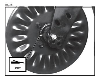
(If Applicable) Frame Mounted Coulter Hubs - STYLE A - 1 Zerk Per Hub
