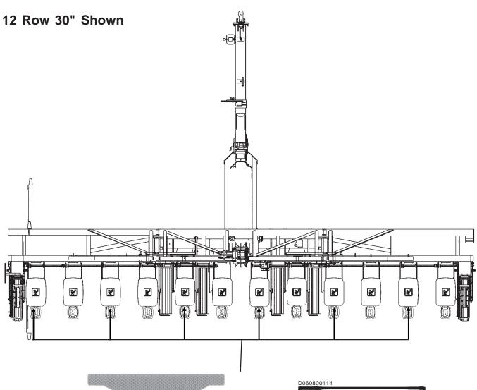
Part No. G7100-262 Amber Reflective Decal (Located On The Hopper Support On Every Other Row Beginning On The 1st Row On The L.H. End Of The Planter - Side-Facing In Transport Position) (Standard) (If Applicable)
