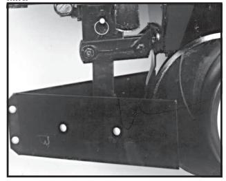
Lubricate the bushings in the mounting bracket and links at the frequency indicated in the Lubrication Section of this manual. Using a torque wrench, check each bolt for proper torque. If the bolt is loose, it should be removed and the bushing inspected for cracks and wear. Replace bushing if necessary. Only hardened flat washers should be used. Replace damaged flat washers with proper part. Torque bolts to 130 ft. lbs.
