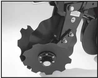
The blade hubs are equipped with sealed bearings. If bearings sound or feel rough when the blade is rotated, replace the bearings.
