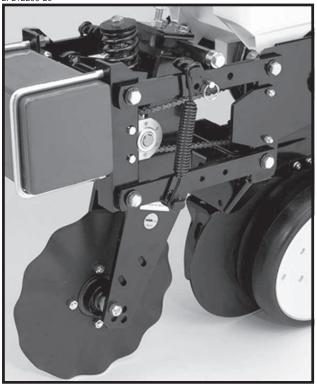
If properly maintained and lubricated (If Applicable) the bearings in the frame mounted coulter hub may never need to be replaced. Lubricate (If Applicable) at the frequency indicated in the Lubrication Section of this manual. Check periodically to be sure nuts and hardware are tightened to proper torque specification. Be sure the coulter is positioned square with the planter frame and aligned in front of row unit disc opener.
