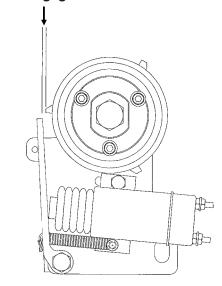
NOTE: To adjust gap between actuator arm and stop, loosen nut on mounting pin and move pin in slot until there is 1/8" ( $\pm 1/32$ ") gap between arm and stop on stop collar. Retighten nut.
