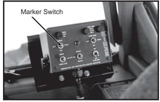
Three Position Selector Switch On Control Console
