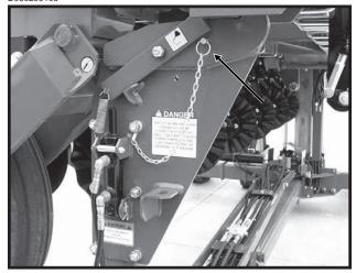
**Transport Latch Locking Pin Installed For Transport**
