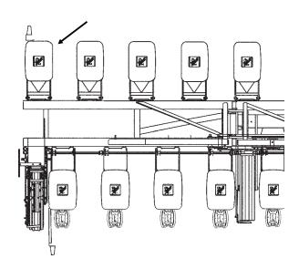
An Even-Row Push Row Unit Package is available to add one additional push row unit onto the L.H. side of the outer end of the front toolbar for use along with the Solid Row Interplant® Package.
