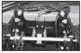
"LSHAFT" will display on the lower LCD when the first shaft rotation sensor is installed. "RSHAFT" will display when the second shaft rotation sensor is installed.
