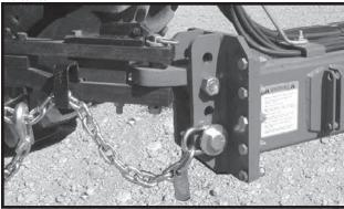
Four holes in the hitch bracket allow the clevis to be raised or lowered. In addition, the clevis may be turned over for a finer adjustment between mounting holes. When installing the clevis mounting bolt, make sure the lock nut is tightened to proper torque setting.
