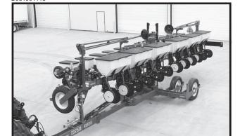
With the tongue fully extended and the planter in the raised transport position, remove the tongue safety pin and store it in the storage position.
