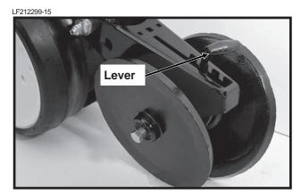
Light soil usually requires less down force at average depth (approximately 2") while heavy soil requires increased down force.
