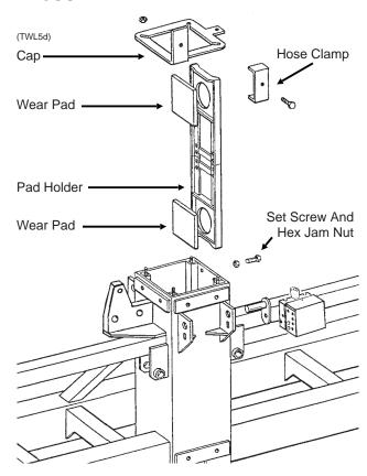
The center section of the planter consists of a steel tubular frame equipped with four wear pad assemblies which travel up and down against a stainless steel clad center post. Each wear pad assembly consists of a pad holder and two wear pads. The wear pads are held in place by the pad holder and adjusted and locked in adjustment by <sup>3</sup>/<sub>4</sub>" set screws and hex jam nuts.
