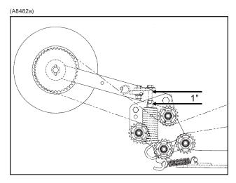
The initial spring tension, on the down pressure spring(s) on the piston pump contact drive wheel, is set leaving 1" between the bottom of the mounting plate and the plug on the top of the spring.
