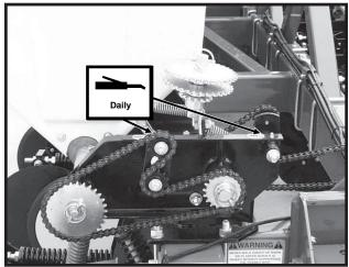
Fertilizer Transmission - 2 Zerks Per Transmission
