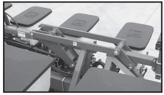
Hold the control console switch labeled RAISE/ WING LOCK in RAISE and operate the hydraulic lever until the two center lift cylinders are fully extended and the safety hook located at the top of the center section rotates into locking position.
