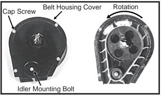
If the belt is being replaced, make sure it is installed to correctly orient the paddles as shown. A diagram molded into the drive sprocket also illustrates the correct orientation.
