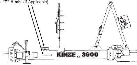
Part No. G7100-259 Amber Reflective Decal (Qty. 2 - 1 Located On Each Side Of Transport Latch Post) 8 Row 36"/38" - "Y" Hitch (If Applicable)
