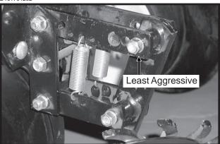
To lock the residue wheel up out of the ground, remove the  $^{1}/_{2}$ " x 5" lockup bolt, raise the residue wheel and install bolt.
