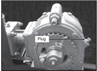
Check crankcase oil daily and maintain at plug level. Fill as needed with EP 90 weight gear oil. Total oil capacity is approximately  $^{3}/_{4}$  pint.
