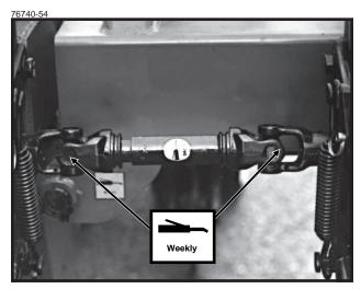
8. U-Joints - 2 Zerks Per Hinge Area
