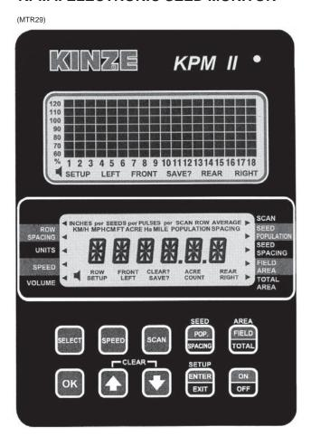
The electronic seed monitor system consists of a console, which is mounted on the tractor; seed tubes with computerized sensors, one of which is installed in each planter row unit; a primary harness\*, which connects the console to the planter harness; and a planter harness (junction Y-harness and/or harness extensions where applicable) to which the individual seed tube sensors and rotation sensors connect. The monitor works with a magnetic (pickup) distance sensor or radar distance sensor.
