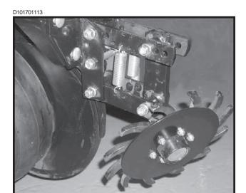
The wheel hub is equipped with sealed bearings. If bearings sound or feel rough when the wheel is rotated, replace the bearings.
