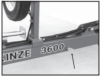
**Tongue Safety Pin Installed For Transport**
