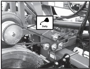
Liquid Fertilizer Contact Drive Chain (Piston Pump)
