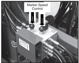
IMPORTANT: The flow controls should be adjusted to restrict flow before the row marker assembly is first put into use. Excessive row marker travel speed can damage the marker assembly.
