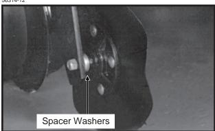
Field adjustment should be made as needed. Operating height of the planter frame will affect operating depth of the frame mounted coulter.
