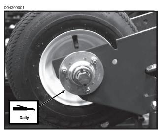
9. (If Applicable) Contact Wheel Arm Bearing - 2 Zerks Per Arm Assembly (Rotate tire while filling with grease.)
