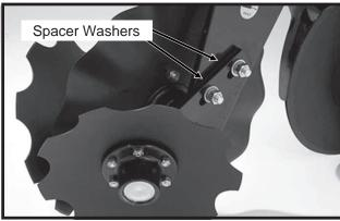
Blades can be adjusted so front edges meet by adding spacer washers between the disc furrower arm and frame mounted coulter fork mount.
