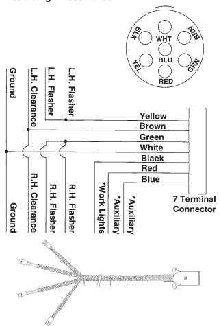
\* Optional customer-supplied auxiliary lights and wires may be wired into existing plug terminals.
