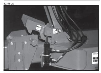
4. Hold the control console switch labeled RAISE/ WING LOCK in WING LOCK and operate the hydraulic lever until the wing lock cylinders are fully extended and the wing locks are locked over center.
