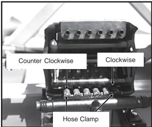
For the right hand hose (facing the pump from front as shown above) twist the hose 1/4 turn in the clockwise direction.
