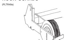
Transport wheel rock guards are designed for use on both sides of each of the four center transport wheels when the planter is used in rocky conditions. Rock guards will help prevent rocks, which can cause damage to the row units, from being picked up by the wheels.
