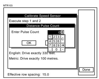
NOTE: If the Distance Pulse Count number starts to count pulses with the tractor not moving, check radar distance sensor for vibration or other interference.
