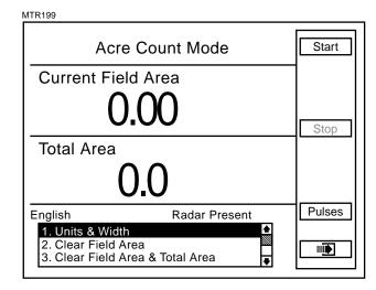
• To Clear Both Field Area And Total Area. Highlight "Clear Field Area & Total Area" and press the knob or Enter key. A note will appear to verify the decision to reset the field area and the total area to zero. Highlight "OK" and press the knob or Enter key to clear the field. Highlight "Cancel" and press the knob or Enter key to retain the current field values.
