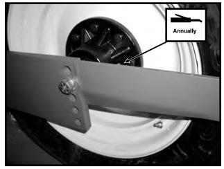
9. Transport Wheel Bearings - 1 Zerk Per Hub
