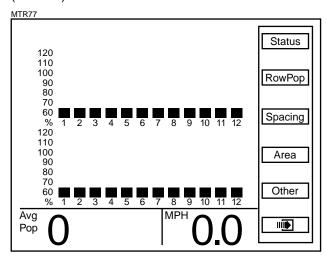
NOTE: The Planter Configuration screen displays the planter rows as programmed into the KPM III software. The above screen shows 12 front (Interplant®) rows and 12 rear rows. If the KPM III were programmed for 8 front (Interplant®) rows and 8 rear rows the screen would display 8 front and 8 rear rows.
