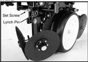
Vertical adjustment in 1/3" increments is possible by removing the lynch pin which secures the vertical support arm and moving the support arm up or down as required. Reinstall lynch pin. Finer adjustment can be attained by removing the lynch pin and using the 5/8" x 2 1/4" set screw to clamp the support arm in the required position.
