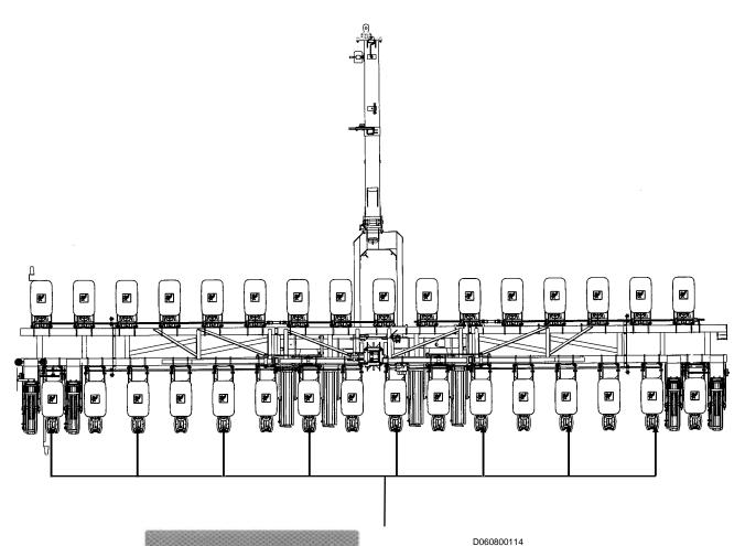
Part No. G7100-262 Amber Reflective Decal (Located On The Hopper Support On Every Other Row Unit Beginning On The 1st Row Unit On The L.H. End Of The Planter - Side-Facing In Transport Position) (Standard)
