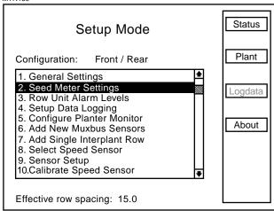
STEP 2 Select meter type by highlighting "Meter Type" and pressing the knob or Enter key, then highlight "Mechanical" or "Vacuum" and press the knob or enter key.
