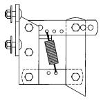
To adjust down force springs, raise the row unit out of the ground and reposition springs as shown for the desired down pressure. D101701112
