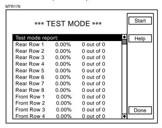
STEP 6 Begin the test with the tractor stopped. For EdgeVac planters, ensure the vacuum is on and that the seed discs are full.
