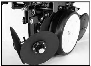
Lubricate the bushings in the support arm and mounting bracket at the frequency indicated in the Lubrication Section of this manual. Using a torque wrench, check each bolt for proper torque. If the bolt is loose, it should be removed and the bushing inspected for cracks and wear. Replace bushings as necessary. Only hardened flat washers should be used. Replace damaged flat washers with proper part. Torque cap screws to 57 ft. lbs.
