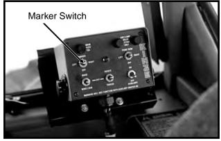
Three Position Selector Switch On Control Console
