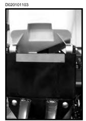
Part No. G7100-259 Amber Reflective Decal (Qty. 6 Used On 12 Row; 8 On 16 Row - Located On The Front Of Every Other Push Row Unit Beginning With The Center Row Unit And Every Other Row Unit To Both Ends - Side-Facing In Transport Position)
