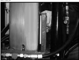
(g) Remove old pads and install new pads. NOTE: Apply a small amount of weather stripping adhesive to hold the pads in place while the pad holder is being reinstalled.
