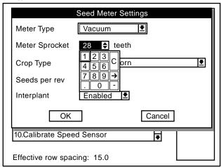
NOTE: When Vacuum "Meter Type" is selected "Meter Sprocket" automatically defaults to 28 teeth. To change "Meter Sprocket" select "Meter Sprocket" by turning the knob or using the arrow keys. Press the knob or enter key, a drop down number pad will appear. Turn the knob or use the arrow keys to highlight the first digit of the desired number and press the knob. When the correct number is obtain press the knob or enter key.
