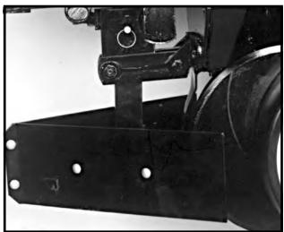
Lubricate the bushings in the mounting bracket and links at the frequency indicated in the Lubrication Section of this manual. Using a torque wrench, check each bolt for proper torque. If the bolt is loose, it should be removed and the bushing inspected for cracks and wear. Replace bushing if necessary. Only hardened flat washers should be used. Replace damaged flat washers with proper part. Torque cap screws to 57 ft. lbs.
