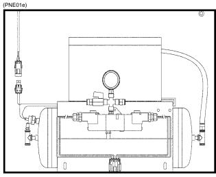
**Air Compressor With Dual Solenoid Assembly**
