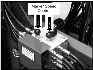
IMPORTANT: The flow controls should be properly adjusted to restrict flow before the row marker assembly is first put into use. Excessive row marker travel speed of the marker can damage the marker assembly.
