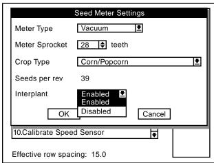
STEP 6 Turn the knob or use the arrow keys to highlight either "enable" or "disable" and press the knob or Enter key.
