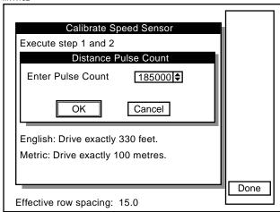
• When the "Enter Pulse Count" value is highlighted press the knob or Enter key and a drop down key pad will appear. Turn the knob or use the arrow keys to highlight "0", zero, and press the knob or Enter key. Turn the knob or use the arrow keys to highlight "OK" and press the knob or Enter key to return to the "Calibrate Speed Sensor" screen.
