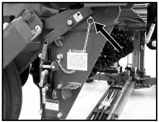
**Transport Latch Locking Pin Installed For Transport**
