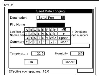
STEP 6 Use the knob or arrow keys to scroll to the "Comment for file" box. Press the knob or Enter key to display the drop down keyboard. Use the keyboard to enter a Comment for the file then press the Enter key.
