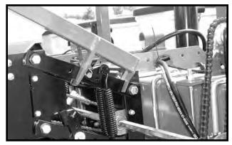
Lift Lever Positioned To Lift Push Row Unit
