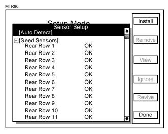
STEP 6 When "OK" appears behind ALL sensors, press the F6 key next to Done. The "Setup Mode" menu will then appear.
