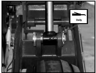
10. Wing Lift Cylinders - 1 Zerk Per Cylinder
