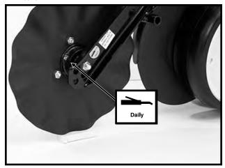
Row Unit Mounted No Till Coulter Hubs - 1 Zerk Per Hub
