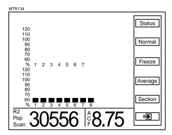
Press the F3 key next to Freeze to stop scanning, the left display item will be frozen on a particular row. "Frzn" appears in the lower L.H. corner to indicate the display is frozen. To resume scan press the F3 key next to Scan.
