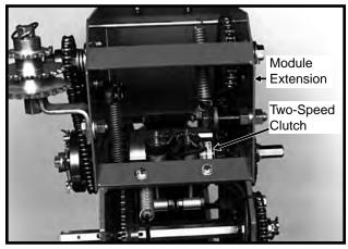
The Two-Speed Point Row Clutch Package is designed to allow on-the-go population rate adjustment as well as the capability to shutoff either half of the planter for finishing up fields or for long point row situations.
