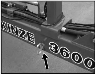
**Tongue Safety Pin Installed For Transport**
