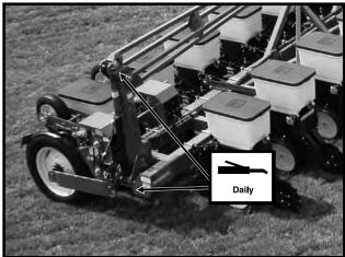
Row Marker Assemblies - 4 Zerks Per Assembly On 8 Row Wide And 12 Row 30". 2 Zerks Per Assembly On 12 Row Wide And 16 Row 30".
