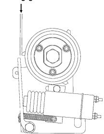
NOTE: To adjust gap between actuator arm and stop, loosen nut on mounting pin and move pin in slot until there is  $\frac{1}{8}$ "( $\pm\frac{1}{32}$ ") gap between arm and stop on stop collar. Retighten nut.
