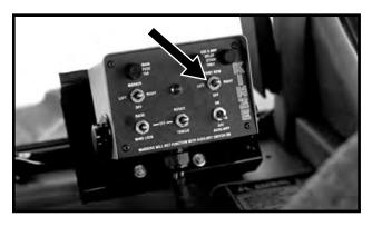
The selector switch for the clutches is located on the planter control console.
