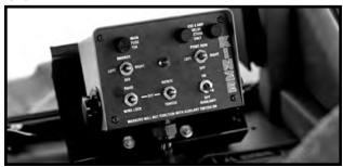
The tractor's hydraulic system and switches on the control console located on the tractor are used to raise the planter to transport position, operate the rotate and tongue extension functions, lock and release the planter wings, and raise and lower the row markers.
