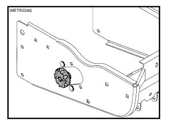
To disengage the drive, turn the knob ½ turn counterclockwise. To engage the drive, turn the knob ¼ turn clockwise.
