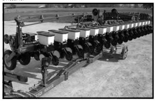
5. Raise the planter 1"-2". The safety hook will release and snap away from the catch pin on the top of the pivot post.
