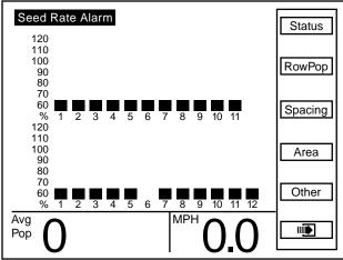
If the sensor is detecting no seed flow it will display which row is not functioning. The alarm may be caused by a mechanical problem reducing seed flow or an electrical problem causing an incorrect seed count.
