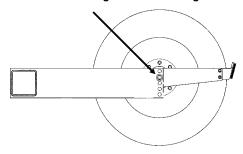
NOTE: The toolbar should operate at a 20"-22" height measured from the bottom of the toolbar to the planting surface.
