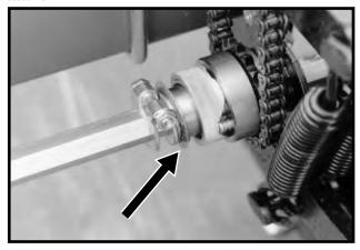
The push row unit clutch sprocket is designed to allow the push row unit drill shaft to be disengaged when only the pull row units are being used.
