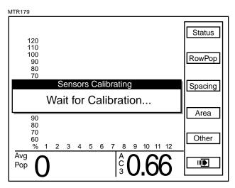
NOTE: Do not attempt planting before the "Wait For Calibration" message disappears. If the planter is moving while sensors are calibrating alarms will be generated.
