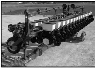
1. With the tongue fully extended and the planter in the raised transport position, remove the tongue safety pin and store it in the storage position.
