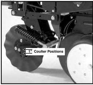
Frame mounted coulters with 1" bubbled, 1" fluted (8 flutes) or ¾" fluted (13 flutes) blades may be used on pull row units only. They are not compatible with push row units.
