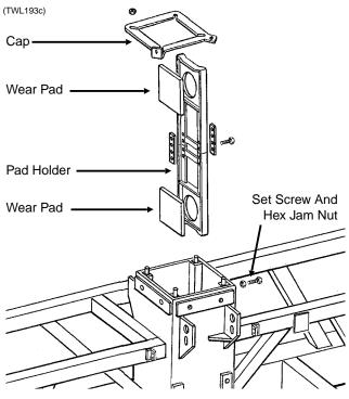
The center section of the planter is contructed around a steel tubular frame with four wear pad assemblies that ride against a stainless steel clad center post. Each wear pad assembly includes a pad holder and two wear pads. The wear pads are held by the pad holder and locked in place by 3/4" set screws and hex jam nuts.
