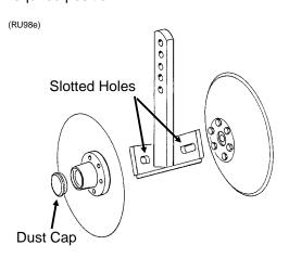
Slotted holes in the support arm where the blades are mounted allow fore and aft adjustment of the disc blades. Blades can be adjusted so the front edges meet or one blade can be moved to the rear and the other to the front of the slot so the cutting edge of one blade overlaps the edge of the other blade. The dust cap must be removed to make these adjustments.
