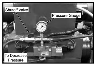
To lock up push row units equipped with pneumatic down pressure springs:
