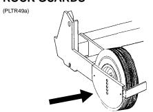
Transport wheel rock guards are designed for use on both sides of each of the four center transport wheels when the planter is used in rocky conditions. Rock guards will help prevent rocks, which can cause damage to the row units, from being picked up by the wheels.
