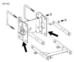
Row unit extension brackets are required on the 4 center pull row units if the Model 3600TR planter is equipped with coulter mounted residue wheels. The brackets extend the row units rearward 4" to provide required clearance.
