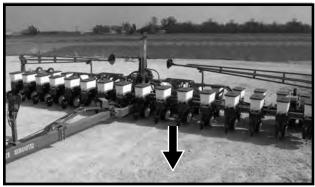
Hold the control console switch labeled "RAISE/ WING LOCK" in "WING LOCK" and operate the hydraulic lever to release the wing locks.
