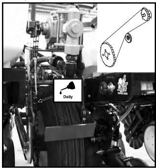
Liquid Fertilizer Ground Drive Chain (Piston Pump)
