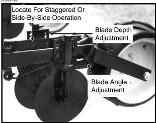
Five sets of holes in each disc bracket allow for  $\frac{1}{2}$ " incremental blade depth adjustment.
