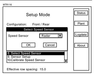
STEP 4 Press the knob or Enter key to select the "Speed Sensor" field and a drop down menu will appear.
