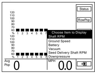
Press the F5 key next to Other to display items available to display in the bottom R.H. corner. Turn the knob or use the arrow keys to highlight "Shaft RPM". The value will appear in the bottom R.H. corner of the display as "RPM".
