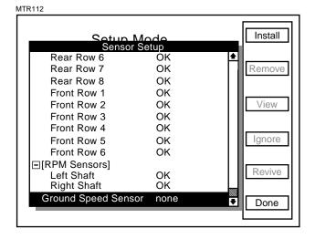
STEP 8 Press the F1 key next to Install. The monitor will beep twice to confirm selection.
