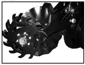
**STYLE B - Used With Style B Row Unit Mounted No Till Coulter**
