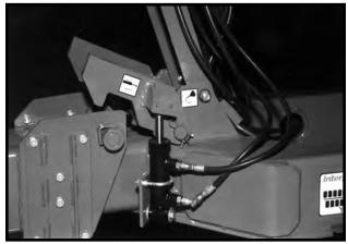
4. Hold the control console switch labeled "RAISE/ WING LOCK" in "WING LOCK" and operate the hydraulic control until the wing lock cylinders are fully extended and the wing locks are locked over center.
