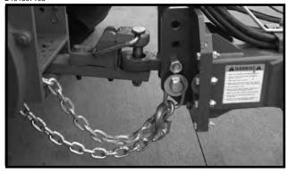
Four holes in the hitch bracket allow the clevis to be raised or lowered. In addition, the clevis may be turned over for a finer adjustment between mounting holes. When installing the clevis mounting bolt, make sure the lock nut is tightened to proper torque setting. (840 ft./lbs.)
