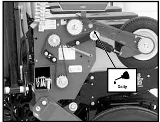
Contact Drive Wheel Arm (2 Per Wheel Assembly)
