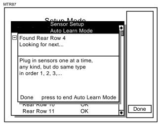
NOTE: After each sensor has been installed "OK" will appear after the sensor name on the LCD screen.
