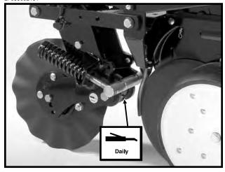
Frame Mounted Coulter - 1 Zerk Per Arm
