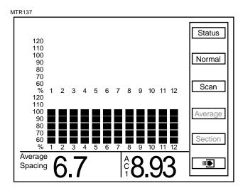
Press the F3 key next to Scan and the monitor will scan through each row in ascending order displaying the average seed spacing for each row. Scan appears in the L.H. corner to indicate the display is scanning. After all rows have been scanned the average population is displayed and scanning will continue with the first rear row.
