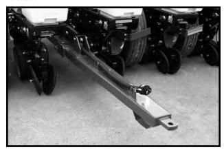
The Rear Trailer Hitch is used to tow a 3 or 4 wheel wagon behind the planter. A spring, chain and mounting bracket are used to support the 1 ½" feed hose from the hitch to the piston pump. This extra length or loop is required to allow the planter to be moved into transport position without stretching the hose.
