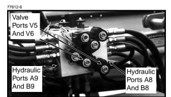
Valve Block Located On Rear Center Frame (Shown With Cover Removed)
