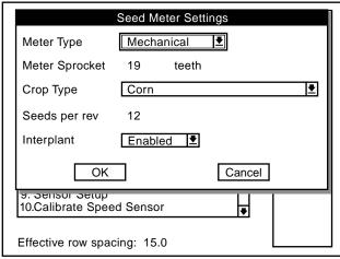
NOTE: When Mechanical "Meter Type" is selceted "Meter Sprocket" automatically sets.
