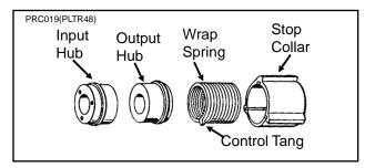
The point row clutch consists of a wrap spring riding on an input hub and an output hub. During operation the wrap spring is wrapped tightly over the hubs connecting them in a positive engagement. The greater the force of rotation the tighter the grip of the spring on the hubs.
