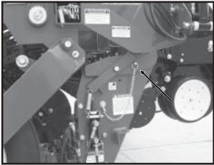
**Transport Latch Locking Pin Installed For Transport**
