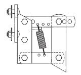
To adjust down force springs, raise the row unit out of the ground and reposition springs as shown for the desired down pressure.
