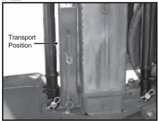
Manual Safety Lockup In Locked Position
