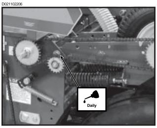
Contact Drive Wheel Arm (2 Per Wheel Assembly)
