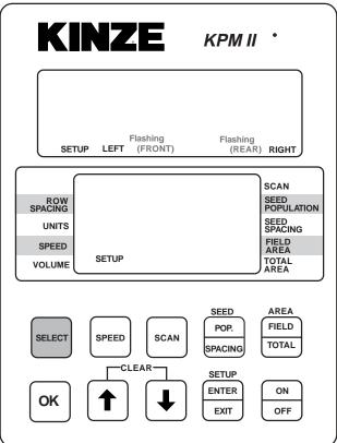
NOTE: Model 3650 planters select the rear configuration only. When Interplant® Package rows are in use, select the rear/front configuration.
