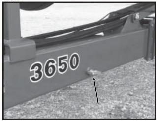
**Tongue Safety Pin Installed For Transport**
