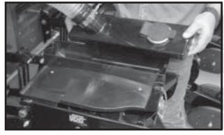
Disengage the seed drive and remove the seed minihopper and meter.
