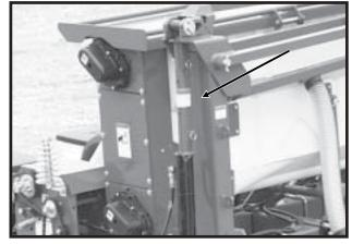
Marker Lockup (Bulk Fill System Shown)
