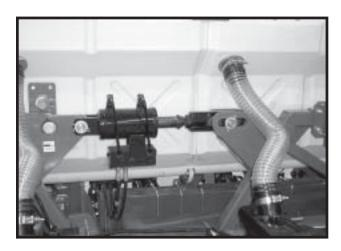
Wing Lock Cylinder With Counter Balance Valve
