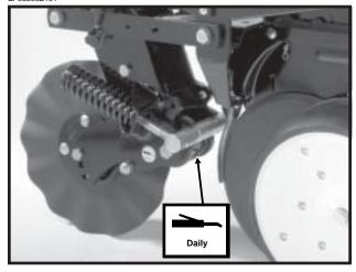
(If Applicable) Frame Mounted Coulter - 1 Zerk Per Arm
