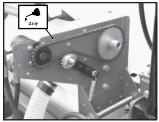
Bulk Fill System Hydraulic Motor Chains (NOTE: Shown With Cover Removed - Slot in rear of cover allows chain to be oiled without removing cover.)
