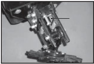
A full threaded bolt and jam nut located on the upper link allows maximum depth to be set for loose soil conditions. Initial setting should be 1  $^{3}/_{4}$ " above the depth of the row unit double disc opener.
