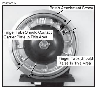
A build-up of debris or chaff may prevent proper finger operation and will require disassembly and cleaning of the finger pickup meter as follows:
