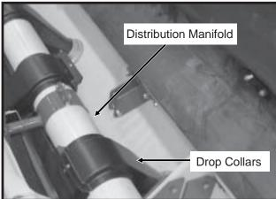
NOTE: After all row outlets are filled to capacity, seed will continue to be evenly distributed to all rows until the bulk seed hopper is empty. When the bulk seed hopper is empty or the auger system is shut off, all drop hoses will "plant out" equally and all rows should run out of seed at approximately the same time.
