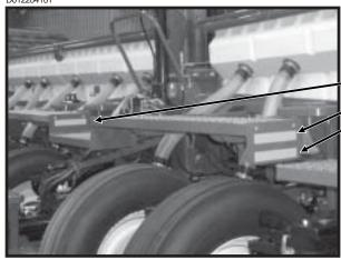
Part No. G7100-260 Orange Reflective Decal (Qty. 6 - Located On Catwalk End Plates)
