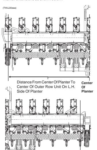
Center Distance From Center Of Planter To Of Center Of Outer Row Unit On R.H.
