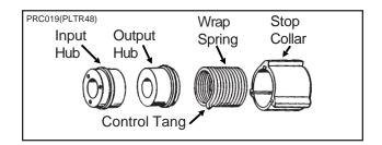
The point row clutch consists of a wrap spring riding on an input hub and an output hub. During operation the wrap spring is wrapped tightly over the hubs connecting them in a positive engagement. The greater the force of rotation the tighter the grip of the spring on the hubs.
