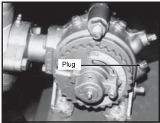
Check crankcase oil daily and maintain at plug level. Fill as needed with EP 90 weight gear oil. Total oil capacity is approximately  $^{3}/_{4}$  pint.
