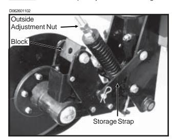
NOTE: The HD single disc fertilizer opener is equipped with a lockup bar that automatically raises and locks the soil press wheel when the blade assembly is raised.
