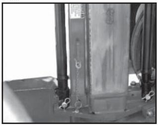
The center post is clad with stainless steel. To prolong service life keep stainless steel surface clean and free of any lubrication.
