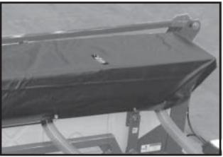
NOTE: The bulk seed hoppers are not water tight. Store the planter inside when possible. Fitted covers, for use if the planter must be stored outside, are available from KINZE® through your KINZE® Dealer. Secure covers using grommets in covers and customer-supplied rubber-tarp straps as needed.
