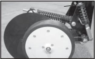
NOTE: The soil press wheel is not intended to be used for gauging fertilizer opener operating depth.
