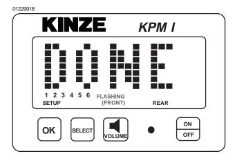
STEP 8 Follow STEPS 5 through 7 to install the second section. If no seed tubes are installed on the second section, press and hold the OK key until the word "DONE" shows on the screen followed by a long beep and the SAVE? icon turns off.
