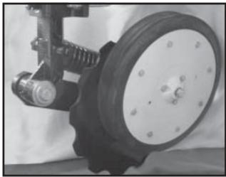
The depth/gauge wheel attachment for the notched single disc fertilizer opener is designed for use in situations where additional gauging is required to maintain desired fertilizer opener depth. The depth/gauge wheel is attached to the notched single disc fertilizer opener using a mounting block fastened to the pivot arm using 5/8" hardware through the disc blade hub w/bearing.
