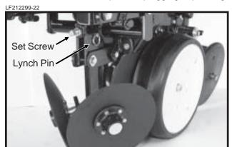
Vertical adjustment in  $^{1}/_{3}$ " increments is possible by removing the lynch pin which secures the vertical support arm and moving the support arm up or down as required. Re-install lynch pin. Finer adjustment can be attained by removing the lynch pin and using the  $^{5}/_{8}$ " x 2  $^{1}/_{4}$ " set screw to clamp the support arm in the required position.
