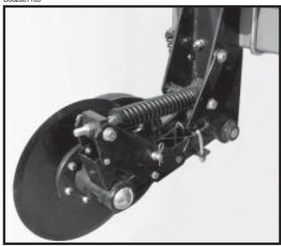
Placement of fertilizer with the HD single disc fertilizer opener is recommended at 3 ½" - 4" from the row. **Never locate the opener to place fertilizer closer than 2**".
