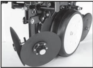
Lubricate the bushings in the support arm and mounting bracket at the frequency indicated in the Lubrication Section of this manual. Using a torque wrench, check each bolt for proper torque. If the bolt is loose, it should be removed and the bushing inspected for cracks and wear. Replace bushings as necessary. Only hardened flat washers should be used. Replace damaged flat washers with proper part. Torque bolts to 130 ft. lbs.
