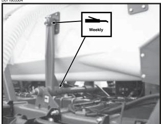
12. Outside Bulk Seed Hopper Link - 2 Zerks Per Link
