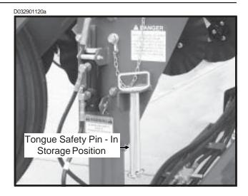
Remove the transport latch locking pin from the locked transport position and place it in the storage location.
