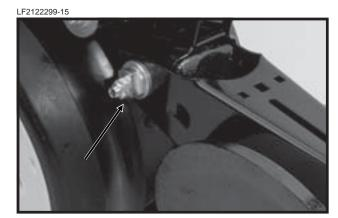
The closing wheels can be installed in two locations either "offset" (to improve residue flow) or "directly" opposite. If set "directly" opposite, the forward installation holes should be used.
