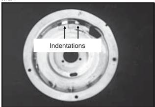
**Photo Shows Worn Carrier Plate**
