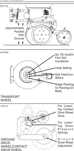
When the planter has been fully loaded with seed, granular chemicals, etc.; a field check should be made to be sure the wings are level with the center frame. If the wings are not level with the center frame, the drive wheels and/or transport wheels can be raised or lowered in the wheel arms to increase or decrease planter toolbar height. Hitch height should be raised accordingly to ensure level operation.
