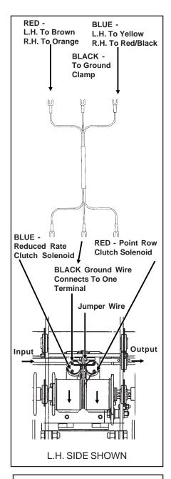
NOTE: Before doing any electrical work, disconnect the control console from the tractor battery. Keep wiring harnesses away from high temperature areas or sharp edges. DO NOT route the wiring harnesses along battery cables. Use tie straps to keep wire harness away from moving parts on tractor and planter. Be sure ground connections to the tractor frame are clean to provide good electrical contact.
