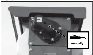
Bulk Fill System Gearbox Drive Chains (5-10 Pumps For Each Gearbox)
