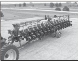
1. With the tongue fully extended and the planter in the raised transport position, remove the tongue safety pin and store it in the storage position.
