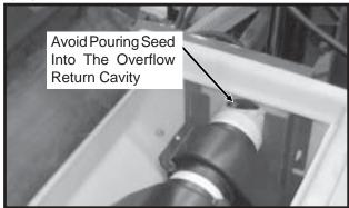
NOTE: When filling the bulk seed hoppers, avoid pouring seed into the overflow return cavity.
