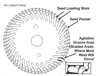
Most wear on the seed disc will be found in the agitation groove area (area between the seed loading slots). Wear will affect planting accuracy at high RPM. To measure for wear, lay a straight edge across the surface of the disc and measure the gap between the disc (at the agitation groove area) and the straight edge. If the agitation groove areas are worn in excess of .030" and accuracy starts to drop off at higher meter RPM, the seed disc should be replaced.
