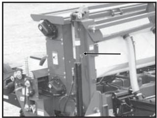
Marker Safety Lockup In Locked Position
