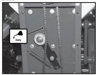
Bulk Fill System Gearbox Chains (NOTE: Shown With Center Cover Removed - Chain can be oiled through top mesh cover without removing cover.)
