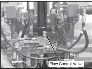
To adjust auger speed, loosen the jam nut and turn the control clockwise, or IN, to decrease auger speed and counterclockwise, or OUT, to increase the auger speed. The auger speed can also be adjusted from the tractor. Adjust flow control on the planter for full flow and control auger speed using the tractor's flow control.
