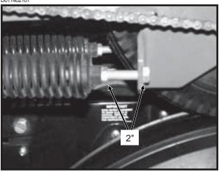
There are two down pressure springs on each contact drive wheel. The down pressure is factory preset and should need no further adjustment.
