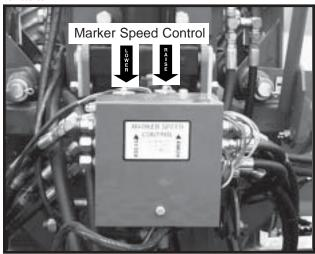
IMPORTANT: The flow controls should be properly adjusted before the marker assembly is first put into use. Excessive travel speed of the markers can damage the marker assembly.
