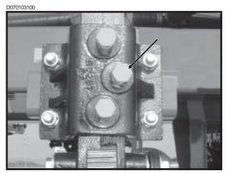
NOTE: Middle cap screw must be tightened prior to tightening depth adjustment cap screws.
