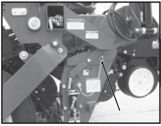
Remove manual safety lockup from its storage location on the hose take-up on the planter hitch and position it behind the front center lift cylinder.
