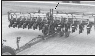
6. Hold the control console switch labeled "ROTATE/TONGUE" in "ROTATE" and operate the hydraulic lever to rotate the planter until the transport latch is engaged.
