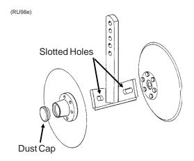
Slotted holes in the support arm where the blades are mounted allow fore and aft adjustment of the disc blades. Blades can be adjusted so the front edges meet or one blade can be moved to the rear and the other to the front of the slot so the cutting edge of one blade overlaps the edge of the other blade. The dust cap must be removed to make these adjustments.
