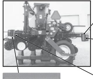
Part No. G7100-260 Orange Reflective Decal (Qty. 1 - Located On The Rear Light Bracket On The L.H. Wing Of The Planter - Rear-Facing In Transport Position)
