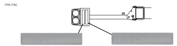
Part No. G7100-258 Red Reflective Decal (Qty. 1 - Located On The Front Light Bracket On The L.H. Wing Of The Planter -Rear-Facing In Transport Position)
