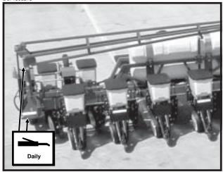
Marker Assemblies - 4 Zerks Per Assembly On 12 Row 30". 2 Zerks Per Assembly On 16 Row 30".
