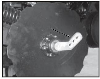
Due to space restrictions, the depth/gauge wheel attachment for the notched single disc fertilizer opener is not applicable to Model 3650 planters equipped with row unit coulter mounted residue wheels.
