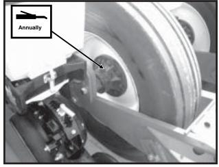
10. Transport Wheel Bearings - 1 Zerk Per Hub
