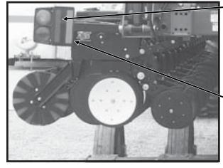
Part No. G7100-258 Red Reflective Decal (With Optional Interplant® Package) (Qty. 1 - Located On Light Bracket On The L.H. Wing Of The Planter - Rear-Facing In Transport Position)
