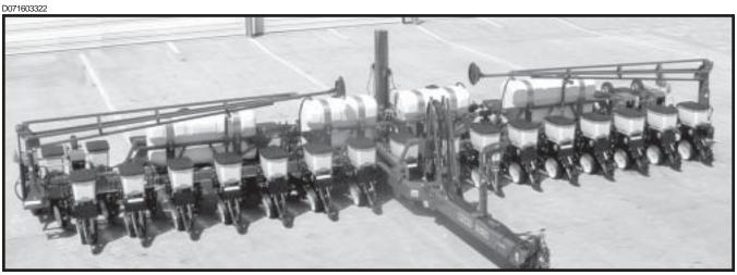
Model 3650 Twin-Line® 16 Row 30" Planter Shown With Conventional Seed Hoppers And Interplant® Package, Even-Row Push Row Unit And Liquid Fertilizer Package Options
