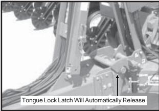
Hold the control console switch labeled "RAISE/ WING LOCK" in "WING LOCK" and operate the hydraulic lever until the wing lock cylinders are fully retracted.
