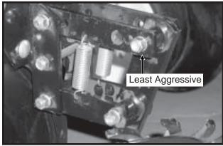
To lock the residue wheel up out of the ground, remove the  $^{1}/_{2}$ " x 5" lockup bolt, raise the residue wheel and install bolt.
