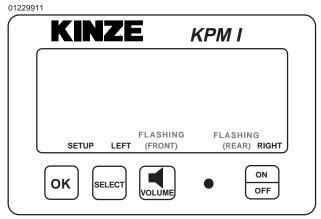
NOTE: Model 3650 planters will use the rear configuration only. When Interplant® Package rows are in use, select the rear/front configurations. When all rows can be viewed on a single display (rear), pressing the select key has no function.
