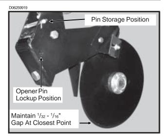
The outer scrapers on each disc blade may also be adjusted to make up for wear that may occur. Make sure the scrapers are adjusted to allow only slight contact with the blades.
