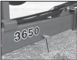
**Tongue Safety Pin Installed For Transport**
