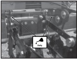
Special Interplant® System Drive Chains (Frame Mounted Coulters)
