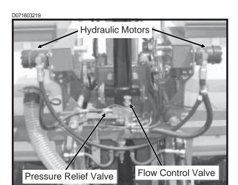
The hydraulic system includes two centrally-mounted hydraulic motors plumbed in series, a pressure relief valve, a check valve and an adjustable flow control valve. The flow control allows auger speed to be varied to meet seed demand.
