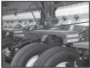
Part No. G7100-260 Orange Reflective Decal (Qty. 6 - Located On Catwalk End Plates)
