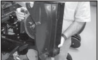
Remove seed disc by loosening wing nuts. Empty the meter. Thoroughly inspect brushes to ensure all seed is removed. Replace seed disc and install wing nuts.
