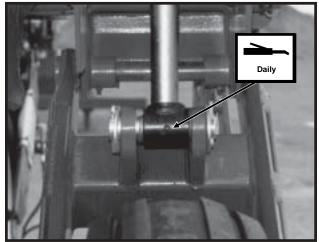
11. Wing Lift Cylinders - 1 Zerk Per Cylinder
