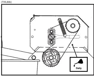
Two-Speed Point Row Clutch Module Drive Chain
