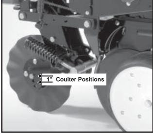
Frame mounted coulters with 1" bubbled, 1" fluted (8 flutes) or 3/4" fluted (13 flutes) blades may be used on pull row units only. (Not compatible with push row units.)
