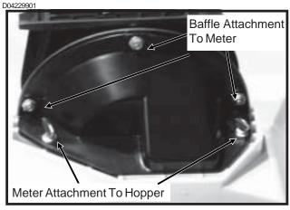
Rotate the seed meter drive by hand to ensure that the springs are holding the tabs of the fingers against the carrier plate where indicated in the photo and that the fingers are being raised in the correct area.
