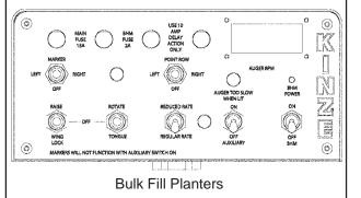
The raise/wing lock and rotate/tongue (fold function) switches are MOMENTARY ON-OFF-MOMENTARY ON type and must be held in position while operating the tractor hydraulic lever. Activating a fold function switch disables the marker circuit.
