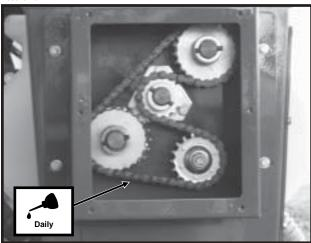
Bulk Fill System Drive Chains NOTE: Shown With Non-Production Cover For Visual Clarity
