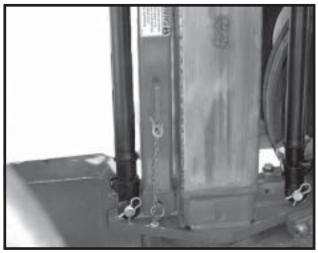
The center post is clad with stainless steel. To prolong service life keep stainless steel surface clean and free of any lubrication.
