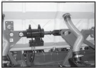
Wing Lock Cylinder With Counter Balance Valve
