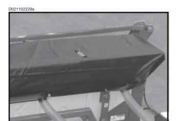
NOTE: The bulk seed hoppers are not water tight. Store the planter inside when possible. Fitted covers, for use if the planter must be stored outside, are available from KINZE® Repair Parts. Secure covers using grommets in covers and customer-supplied rubber tarp straps as needed.
