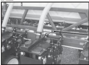
Part No. G7100-89 (Qty. 2 - Located On Wheel Modules On Both Ends Of Planter)
