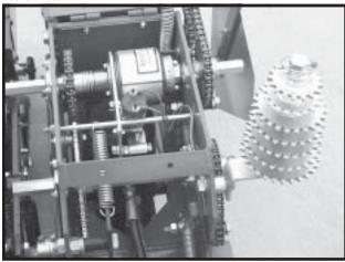
The point row clutches are permanently lubricated and sealed and require no periodic maintenance. DO NOT LUBRICATE. KEEP CLUTCHES CLEAN.
