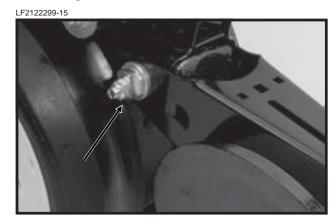
The closing wheels can be installed in two locations either "offset" (to improve residue flow) or "directly" opposite. If set "directly" opposite, the forward installation holes should be used.
