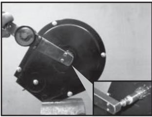
Turn finger holder by hand to make sure it is positioned firmly against the carrier plate, but is not over tightened and can be rotated with moderate force.
