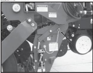
**Transport Latch Locking Pin Installed For Transport**
