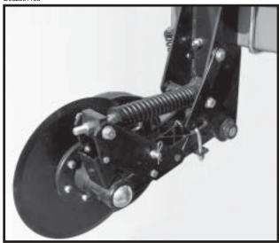
Placement of fertilizer with the HD single disc fertilizer opener is recommended at  $3\frac{1}{2}$ -4" from the row. **Never locate the opener to place fertilizer closer than 2**".
