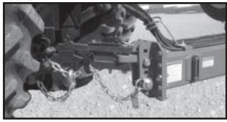
Four holes in the hitch bracket allow the clevis to be raised or lowered. In addition, the clevis may be turned over for a finer adjustment between mounting holes. When installing the clevis mounting bolt, make sure the lock nut is tightened to proper torque setting.
