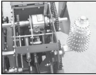
The right hand clutch operates clockwise and the left hand clutch operates counterclockwise. Therefore, some of the parts of the clutch such as the wrap spring differ from one side of the planter to the other. Be sure to use the correct repair part if a clutch must be repaired.
