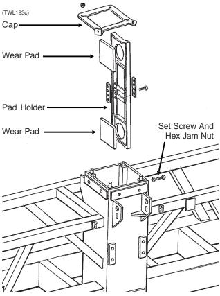
The center section of the planter consists of a steel tubular frame equipped with four wear pad assemblies which travel up and down against a stainless steel clad center post. Each wear pad assembly consists of a pad holder and two wear pads. The wear pads are held in place by the pad holder and adjusted and locked in adjustment by <sup>3</sup>/<sub>4</sub>" set screws and hex jam nuts.
