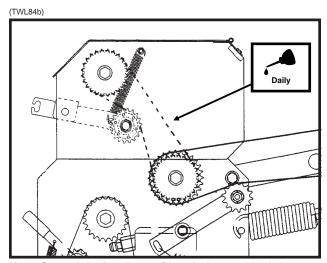
Two-Speed Point Row Clutch Inner Module Drive Chain
