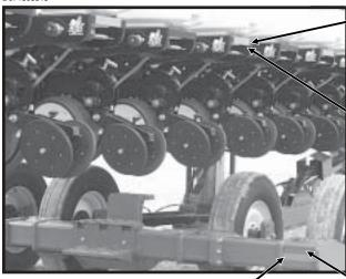
Part No. G7100-262 Amber Reflective Decal (Qty. 6 On 12 Row 30" And 8 On 16 Row 30" -Located On Every Other Row Unit Beginning On The First Row Unit On The L.H. End Of The Planter - Rear-Facing In Planting Position/Side-Facing In Transport Position)
