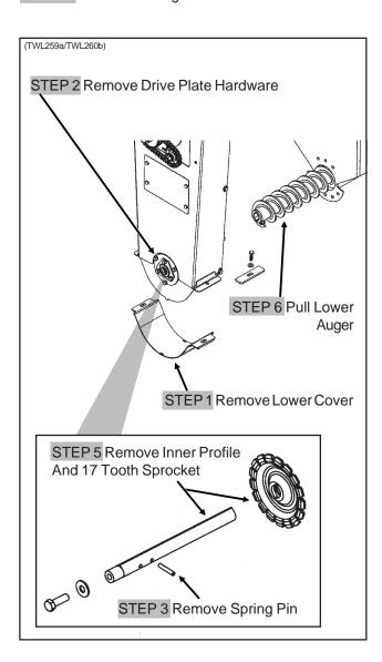
To remove upper bulk seed hopper auger:
