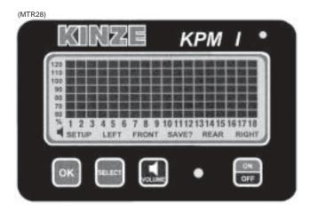
The electronic seed monitor system consists of a console, which is mounted on the tractor; seed tubes with computerized sensors, one of which is installed in each planter row unit; a primary harness\*, which connects the console to the planter harness; and a planter harness (junction Y-harness and/or harness extension where applicable), to which the individual seed tube sensors connect.
