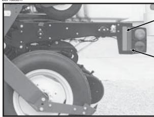
Part No. G7100-260 Orange Reflective Decal (Qty. 1 - Located On The Rear Light Bracket On The L.H. Wing Of The Planter - Rear-Facing In Transport Position)
