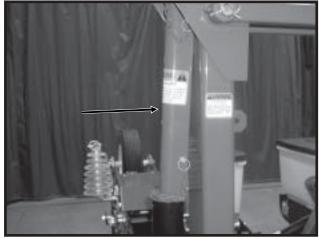
Marker Safety Lockup In Locked Position
