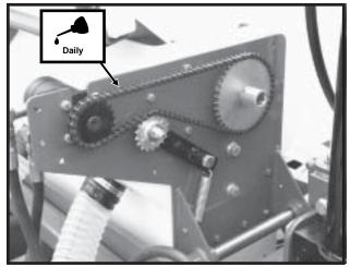
Bulk Fill System Hydraulic Motor Drive Chains NOTE: Shown With Cover Removed - Slots in rear of covers allow chains to be oiled without removing covers.
