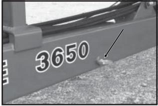
8. Install transport latch locking pin.
