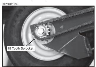
Half rate (2 to 1) drive is recommended only when desired population falls below that shown on planting rate charts. Replace the 30 tooth sprocket on each contact wheel with a 15 tooth sprocket. This will reduce the planter transmission speed and reduce planting and application rates by approximately 50%.
