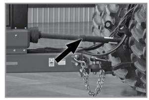
Planter mounted PTO shaft -Lubricate every 8 hours
