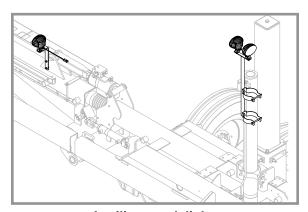
Auxiliary work lights (Additional light mounted on opposite wing)
