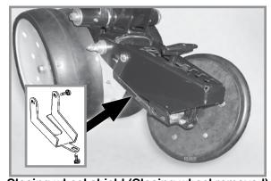
Closing wheel shield (Closing wheel removed)
