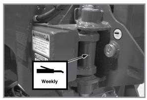
**9. Row marker breakaway** 1 fitting per breakaway - 2 breakaways
