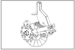
Frame mounted coulter residue wheels
