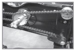
Mechanical pull row unit meter drive
