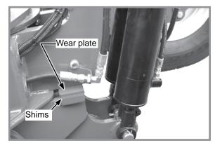
Wear plate an shim installation
