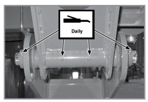
**3. Wing wheel pivot** 4 fittings per wing wheel - 4 wing wheels
