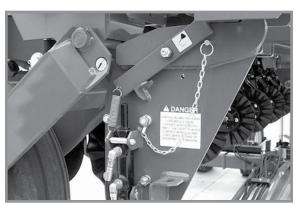
Transport latch locking pin Locked transport position
