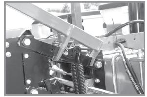
Lift lever positioned on push row unit
