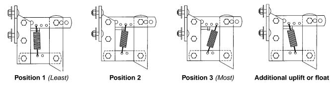
Raise row unit and reposition springs to adjust down pressure.
