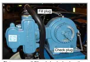
Piston pump oil fill and check plug locations
