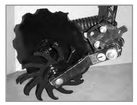
Notched single disc opener residue wheel attachment
