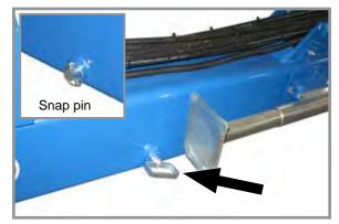
Tongue safety pin installed for transport
