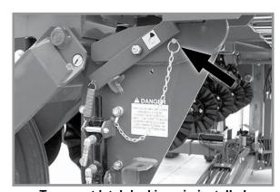
Transport latch locking pin installed
