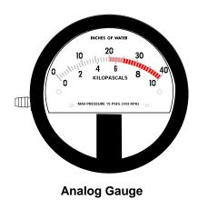
NOTE: Analog gauges are identical EXCEPT for plug and hose barb locations in side of gauge housing. DO NOT connect vacuum meter or bulk fill hose to wrong gauge. Check plug and hose barb installation if readout is erratic or appears inaccurate.
