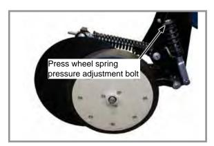
Press wheel down pressure adjustment
