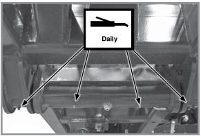
2. Wing hinges 4 fittings per hinge - 2 hinges
