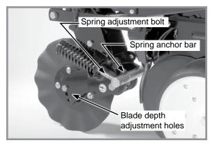
Frame mounted coulter adjustment
