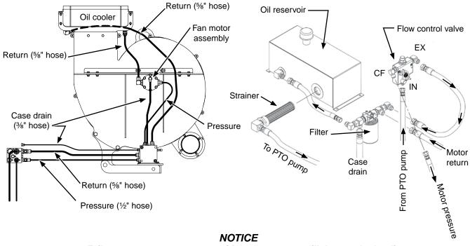
Failure to connect to a return with zero pressure will damage hydraulic motor. Connect hydraulic motor case drain to a case drain return line with zero pressure on tractor. DO NOT connect hydraulic motor case drain to SCV outlet. Contact tractor manufacturer for specific details on "zero pressure return".
