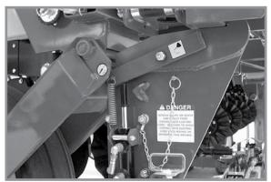
Transport latch locking pin Storage position
