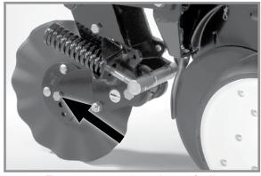
Frame mounted coulter spindle
