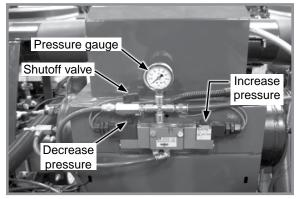
Air compressor assembly controls
