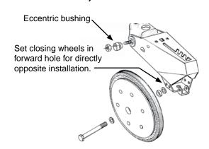
"V" closing wheels should have enough down pressure to close the seed trench and ensure good soil to seed contact. Move 5-position quick adjustable down force lever on the top of closing wheel arm to the rear to increase closing wheel spring pressure. Move lever forward to decrease pressure. Adjust all row units to a similar setting. Light soil usually requires less down force at average depth (approximately 2") while heavy soil requires increased down force.
