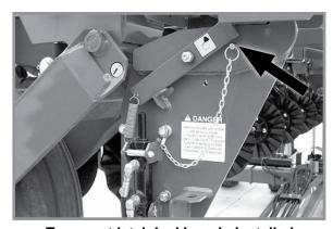
Transport latch locking pin installed
