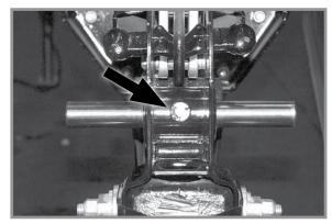
Pivot spindle cap screw
