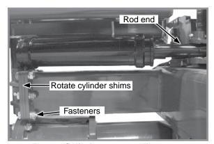
**Rotate Cylinder mount adjustment**
