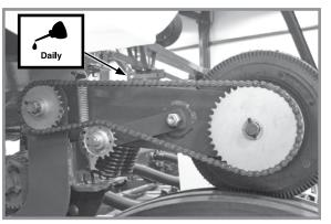
Liquid fertilizer ground drive chains (Piston pump)
