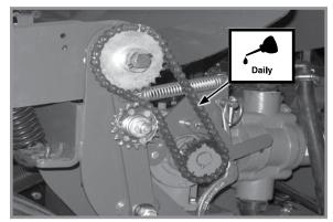
Liquid fertilizer ground drive chains (Piston pump)
