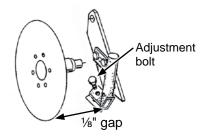
Adjust liquid drop tube/scraper so there is slight contact between blade and scraper lower leading edge, and ½" clearance between liquid drop tube trailing edge and blade. Blade should turn with minimum amount of drag.
