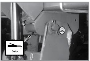
2. Ground drive wheel pivot (2 per wheel module)
