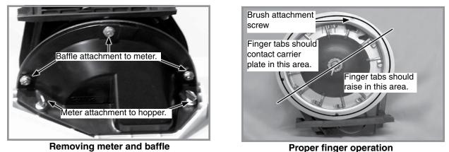
1. Remove two thumbscrews and meter from seed hopper and remove three cap screws and baffle from meter assembly.
