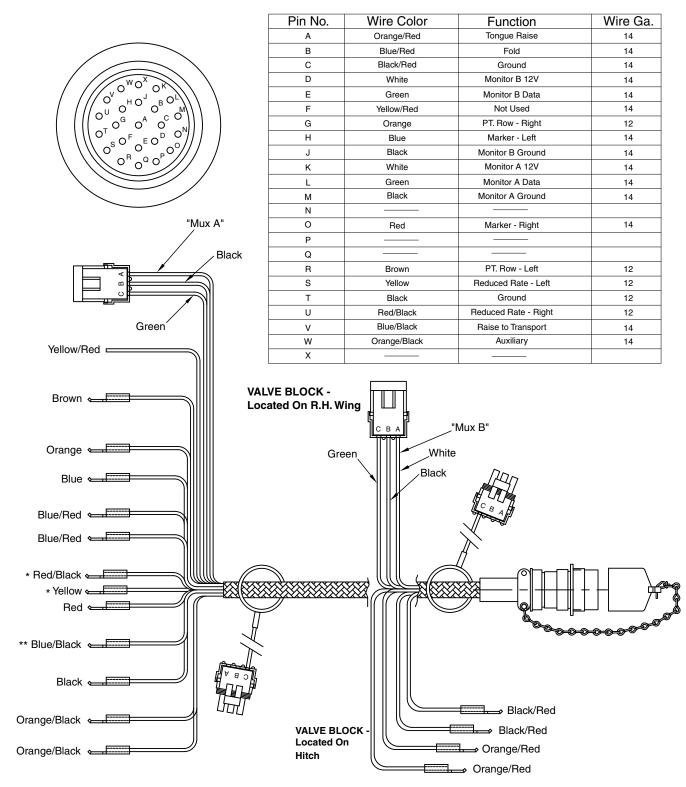
\*\* NOTE: Harness To Port V14 On Valve Block Located On Tower
