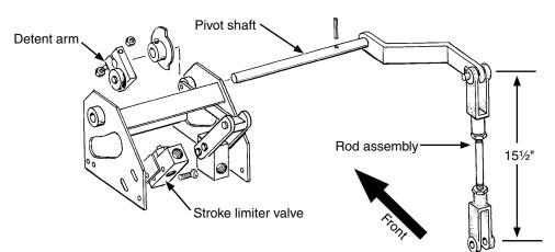
2. Check rod assembly adjustment bolt is set at 15<sup>3</sup>/<sub>4</sub>" pin to pin when planter is fully lowered. Adjust as needed.
