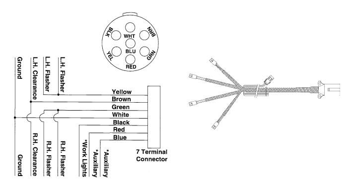
Light packages supplied on Model 3700 Front Folding Planters meet ASABE Standards. Check with tractor manufacturer for correct wiring harness to be wired into lights on your tractor, .
