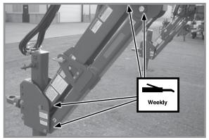
3. Upper and lower hitch linkage (2 per link)
