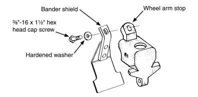
Optional granular chemical bander shield is installed on underside of wheel arm stop to shield crop residue from lodging in granular chemical bander.
