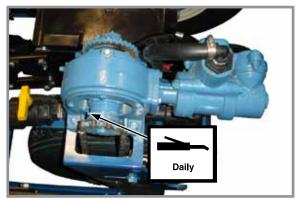
**Piston pump L.H. side (1)** Fill until grease seeps out of bottom drain hole.
