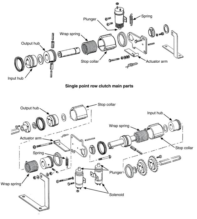
Two-speed point row clutch main parts
