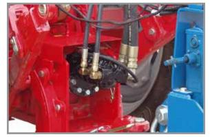
**Two-section PTO hydraulic pump**
