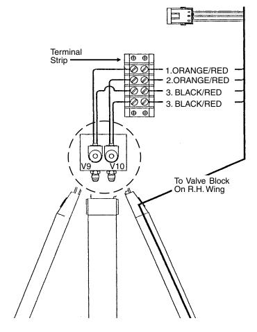
1. ORANGE/RED - Pin "A" (Tongue Retract/Extend) - Port V9 2. ORANGE/RED - Pin "A" (Tongue Retract/Extend) - Port V10 3. BLACK/RED - Pin "C" (Ground)
