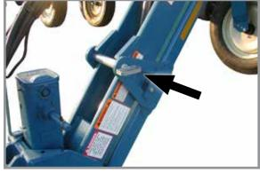
Hitch parallel linkage pin installed
