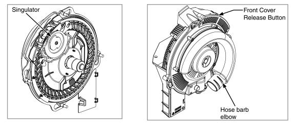
NOTE: Foreign material in seed disc orifices, such as seed chips, hulls, stems, etc., may affect seed delivery. Clean seed ensures accurate seed metering from vacuum seed meter. Remove Seed discs daily to check for buildup of foreign material in seed disc orifices.
