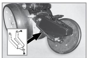
Closing wheel shield (Closing wheel removed)
