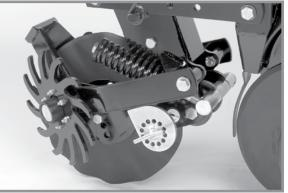
Frame mounted coulter residue wheel
