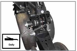
**Gauge wheel arms (2)** Seals in gauge wheel arm are installed with lip facing out to allow grease to purge dirt away from seal. Pump grease into arm until fresh grease appears between washers and arm.
