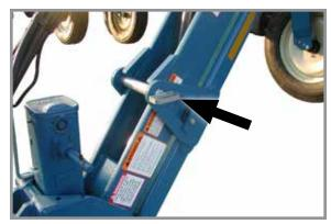
Hitch parallel linkage pin installed
