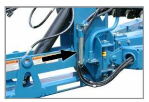
Hitch parallel linkage pin stored
