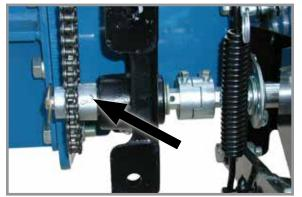
Transmission shaft shear pin
