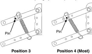
There are four positions to set down pressure spring tension.
