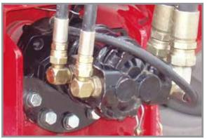
**PTO pump installed**
