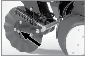
Frame mounted coulter spindle
