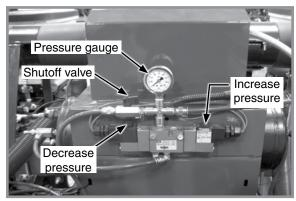
Air compressor assembly controls
