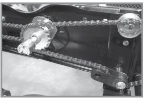
Mechanical pull row unit meter drive
