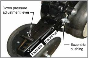
Eccentric bushing Set closing wheels in forward hole for directly opposite installation.
