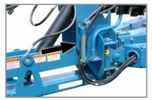
Hitch parallel linkage pin stored
