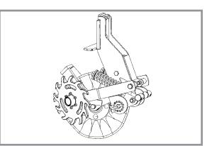
Frame mounted coulter residue wheels
