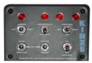
Two-speed point row clutch control box
