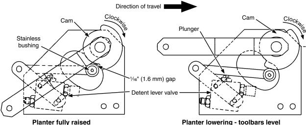
2. Raise planter to fully raised position. With cam positioned as shown, adjust detent lever (lowering control) value in its mounting slots so there is 1/16" (1.6 mm) gap between stainless bushing and cam. Lower edge of cam must be above pivot point of stainless bushing.
