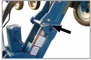
Hitch parallel linkage pin installed
