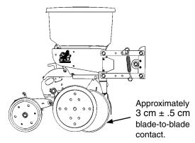
NOTE: Proper blade clearance is critical. Blades should have  $1" \pm \frac{1}{2}" (3 \pm .5 \text{ cm})$  contact in this area. When blades are turned by hand in opposite directions against each other, there should be only light resistance to turning. Re-adjust blade scraper if necessary to center it between the blades.
