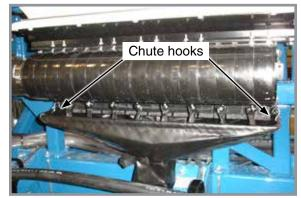
**Cleanout chute installed**
