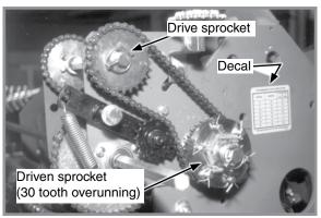
Two-speed point row clutch driven sprockets
