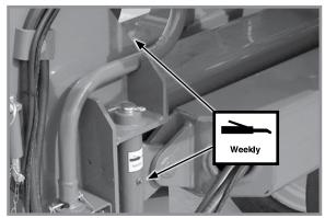
7. Link assemblies (1 per assembly) Front wear pads (4)
