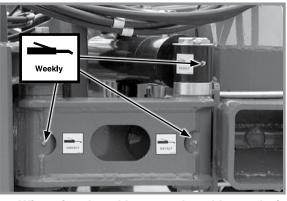
10. Wing pivot knuckle - 1 per knuckle on shaft Helper cylinders (1 per cylinder)
