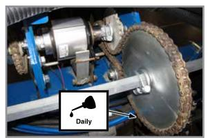
Inner module (point row clutch) drive chains
