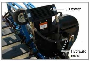
Vacuum fan assembly with oil cooler
