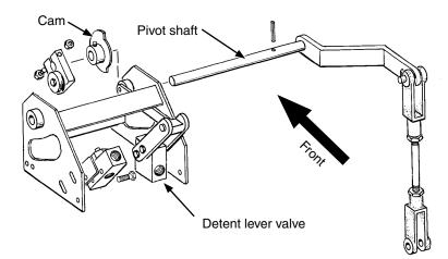
1. Raise planter to field turn around position and check toolbar height is 39"-41" (99 cm - 104 cm). Adjust following procedure for stroke limiter valve adjustment. Stroke limiter (height stop) valve must be correctly adjusted prior to adjusting detent lever (lowering control) valve.
