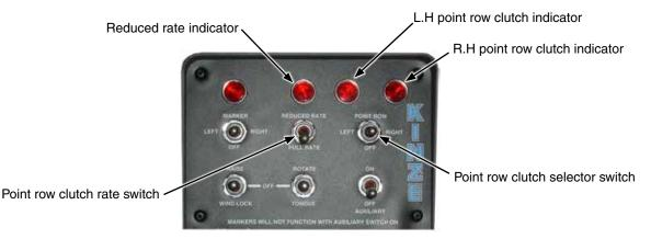
Two-speed point row clutch control box
