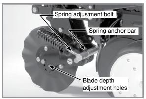
Frame mounted coulter adjustment
