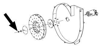
NOTE: Torque vacuum fan impeller assembly to motor shaft <sup>5</sup>/<sub>8</sub>"-18 hex jam nut 50 ft-lb (67.8 N-m).
