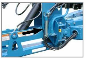
Hitch parallel linkage pin stored
