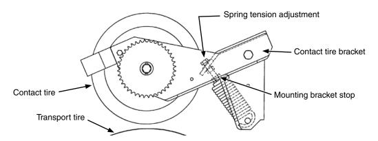
Set piston pump drive spring tension so there is no slack in springs when contact tire bracket is resting on mounting bracket stop. Contact tire and transport tire should not be touching.
