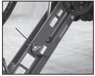
Hitch Parallel Linkage Lock Pin (Prior To Serial No. 750404)
