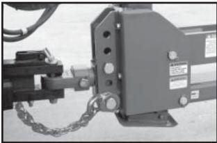
Adjust tractor drawbar in as close to the tractor as practical and to 13-17 inches above the ground. Adjust the drawbar so the hitch pin hole is directly in line with the center of the tractor. Make sure the drawbar is in a stationary position.
