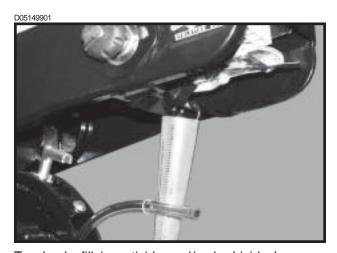
To check, fill insecticide and/or herbicide hoppers. Attach a calibrated vial to each granular chemical meter. Lower the planter and proceed as follows.
