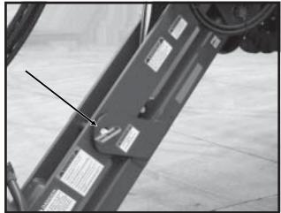
Hitch Parallel Linkage Lock Pin In Transport Position (Prior To Serial No. 750404)
