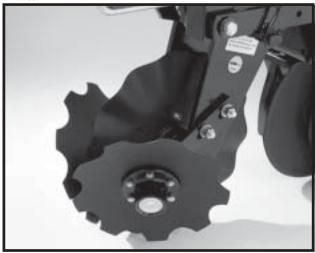
The blade hubs are equipped with sealed bearings. If bearings sound or feel rough when the blade is rotated, replace the bearings.
