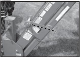
Hitch Parallel Linkage Lockup Pin In Transport Position (Serial No. 750404 And On)
