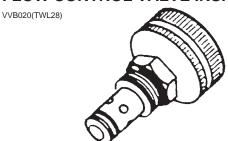
The row marker flow control valves, located in the valve block on the right wing of the planter, should be adjusted for raise and lower speed as part of the assembly procedure or upon initial operation. If a valve fails to function properly or requires frequent adjustment, it should be removed for inspection. Check for foreign material and contamination on both the valve and the seating area of the valve body. Replace any components found to be defective.
