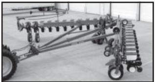
Raise the planter to remove weight from the center lift cylinder lockup brackets. Remove the pin which locks each bracket in place and store the lockup brackets and pins as shown below.
