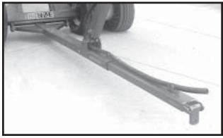
The Rear Trailer Hitch is used to tow a 3 or 4 wheel wagon behind the planter.
