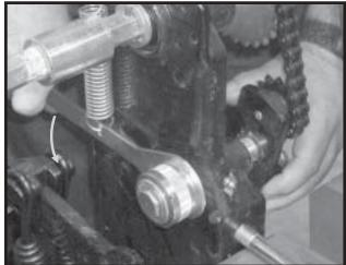
To add chain tension, rotate chain idler into the chain while rotating handle to tension idler spring.
