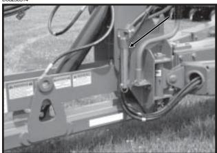
Hitch Parallel Linkage Lockup Pin In Storage Location (Serial No. 750404 And On)
