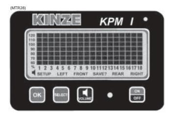
The electronic seed monitor system consists of a console, which is mounted on the tractor; seed tubes with computerized sensors, one of which is installed in each planter row unit; a primary harness\*, which connects the console to the planter harness; and a planter harness (junction Y-harness and/or harness extension where applicable), to which the individual seed tube sensors connect.
