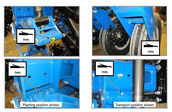
8. Flip Axle, one each at four center wheels 4 fittings per axle
