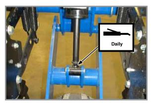
7. Lift Cylinder, 8 per machine 1 fitting per cylinder
