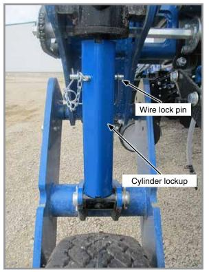
Transport axle cylinder lockup installed
