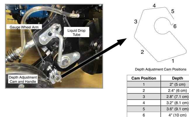
Rotate the depth adjustment cam to adjust depth of fertilizer placement into the soil.
