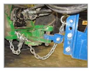
Tractor and Safety Chain Hookup for Drawbar Hitch
