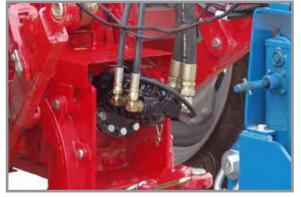
**Two-section PTO Hydraulic Pump**
