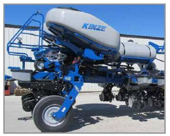
Liquid fertilizer installed on 4900 bulk fill
