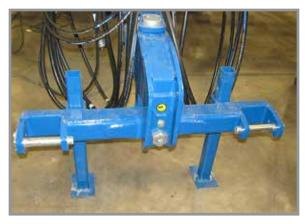
Jacks in Maintenance Position For transporting, store jacks on both sides of hitch. Secure in place with spring pin.
