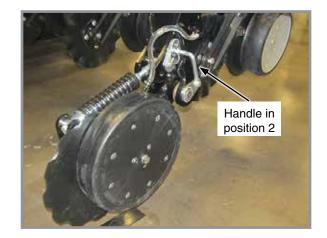
NOTE: The opener is designed to operate with the gauge wheel as the primary depth stop when in position 3. In softer conditions, position 2 can be used to control depth using the gauge wheel as well as planter frame to limit opener travel. In all positions, the opener will spring up when encountering a foreign object or hard ground.
