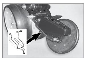
Closing Wheel Shield (closing wheel removed)
