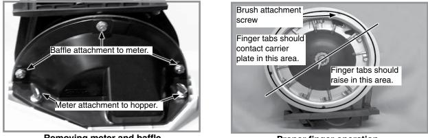
Removing meter and baffle
