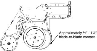
NOTE: Proper blade clearance is critical. Blades should have  $1" \pm \frac{1}{2}"$  ( $3 \pm 5$  cm) contact in this area. When blades are turned by hand in opposite directions against each other, there should be only light resistance to turning. Re-adjust blade scraper if necessary to center it between the blades.
