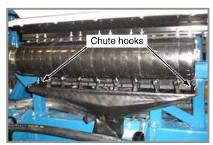
**Cleanout Chute Installed**
