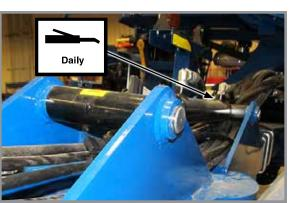
6. Wing Down Pressure Cylinder, 2 per machine 2 fittings per cylinder (one each end)
