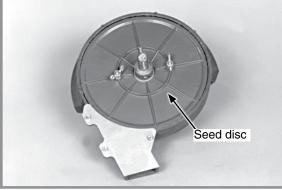
Brush-type seed meter seed disc installed
