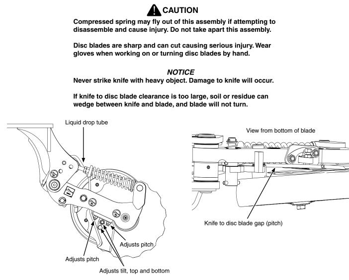
Check knife to disc blade clearance and adjust if necessary as described below.
