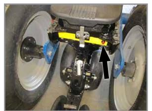
Use the manual run button to turn on seed meter, fertilizer and insecticide on each row unit to check functionality.
