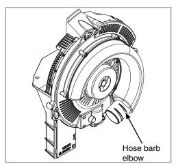
NOTE: Foreign material in seed disc orifices, such as seed chips, hulls, stems, etc., may affect seed delivery. Clean seed ensures accurate seed metering from vacuum seed meter. Remove Seed discs daily to check for buildup of foreign material in seed disc orifices.
