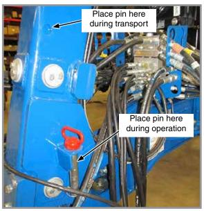
Place the drawbar hitch lockup pin in the hole shown above when machine is in operation.
