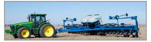
3. For planters equipped with drawbar hitch, operate proper hydraulic tractor control and press and hold the RAISE HITCH button on your ISOBUS monitor to raise drawbar to level planter frame.
