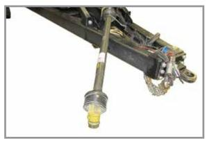
PTO shaft positioned for tractor hookup
