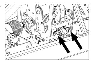
9. Remove two bolts which secure idler assembly to tower auger housing. Slide idler assembly to the side for clearance to remove belt from lower pulley.
