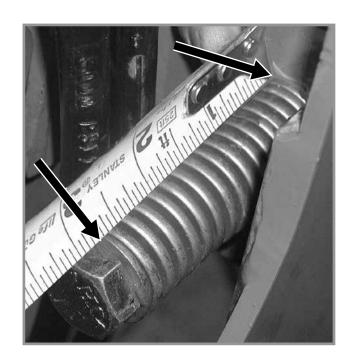
8. Collapse belt tension springs by tightening nylon lock nuts.
