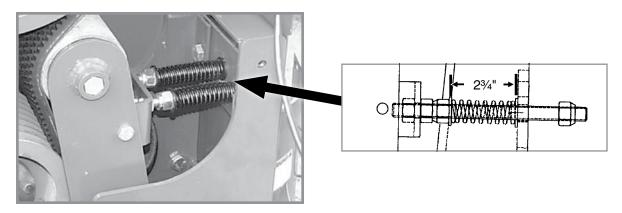
14. Check and adjust belt tension.
