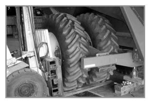
Place blocking under cart at rear undercarriage/frame and lower jack until frame is supported by blocking. Place blocking to provide a wide base of support.
