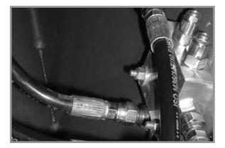
Counter balance valves prevent auger fold cylinder from extending or retracting without applied hydraulic pressure. If valve(s) fail to lock auger in position or fail to function properly, remove valve(s) from valve block and check for foreign material. Replace valve if defective.
