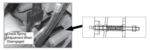
6. Check and adjust spring dimension. See "V-Belt Tension Adjustment And Alignment"
