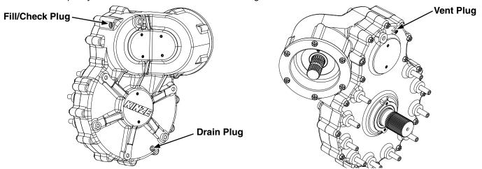
Remove plug from fill/check plug hole on the gearbox. Oil level should be even with fill/check plug hole. Inspect oil at end of each annual season of use for moisture and contaminates, if found, change oil before storage.
