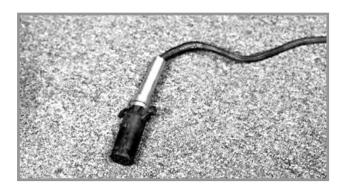
Additional auxiliary work lights are available from Kinze Repair Parts which may be wired into existing auxiliary light wires in the harness. The vertical auger work light is wired into the black terminal connector.
