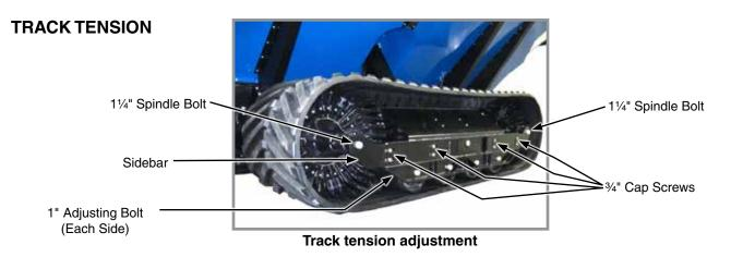
There should be approximately 2" sag in track at midpoint between front and rear end wheels.
