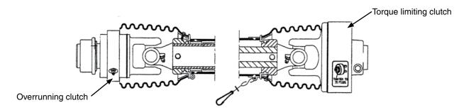
The torque limiting clutch disengages if auger becomes obstructed to prevent driveline and gearbox damage. The torque limiting clutch resets automatically when PTO RPM is reduced.
