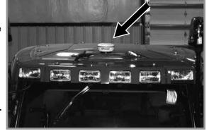
Route the GPS cable into the right side or bottom of the cab (dependent upon the location of the KINZE Vision<sup>™</sup> display).
