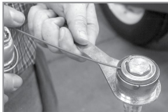
Wrap Spring Wrench Lubrication
