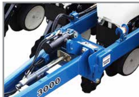
Interplant self-leveling hitch extension
