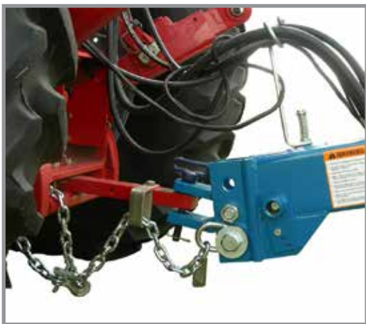
Drawbar and safety chain connection (Prior to 2019 Production)
