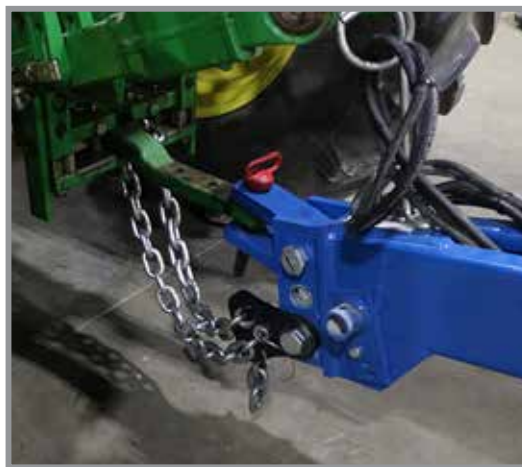
Drawbar and safety chain connection (2019 Production and on)
