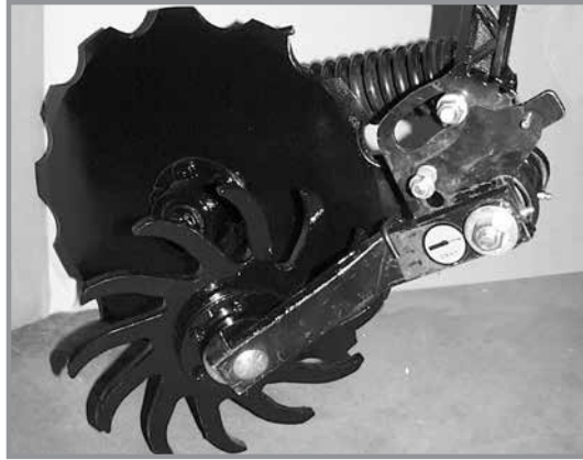
Notched single disc opener residue wheel attachment
