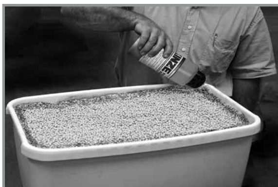
Adding graphite to conventional hopper
