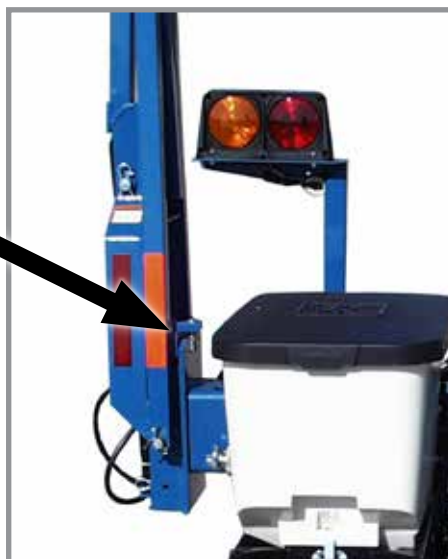
Marker arm safety lockup pin location
