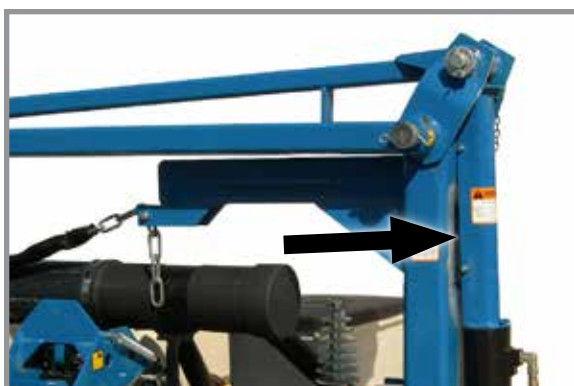
Row marker safety lockup installed
