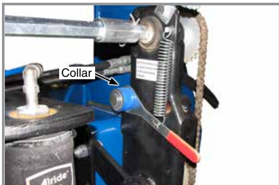
Wrap spring wrench (L.H. rotation shown)
