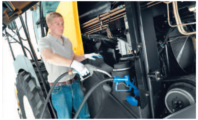
The fill openings for the fuel and 40 gallon AdBlue® tanks are conveniently located next to each other under the left side shield.
